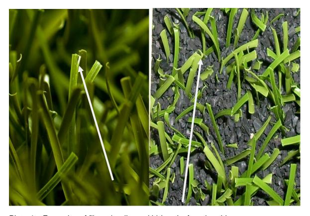
Plate 4 – Examples of fibre a) splits and b) breaks from brushing
