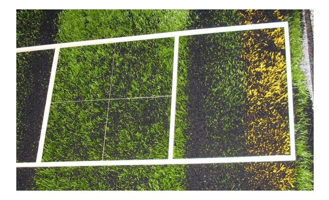
Plate 2 – Measuring quadrangle frame, set on a rubber crumb infilled system – the central portion showing loss of fill highlights the channel tracked by the power brush.
