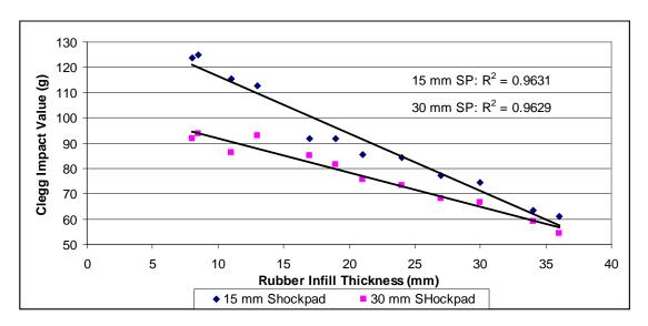
Figure 1. The effect of Rubber infill depth on the Clegg Impact Value of a third generation synthetic long pile turf surface, and for two thickness shockpads. The linear regression lines show a good fit between rubber infill thickness and Clegg Impact Value.
