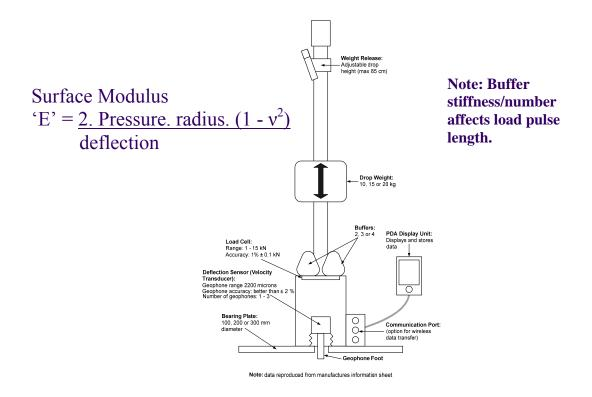
Figure 4 Schematic of and LWD Device, and the Bousinessque Equation
