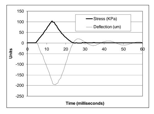
Figure 5, A Typical (good) Test Trace of Load and Deflection. (Note the small amount of rebound in the deflection trace and that deflection lags slightly behind load).
