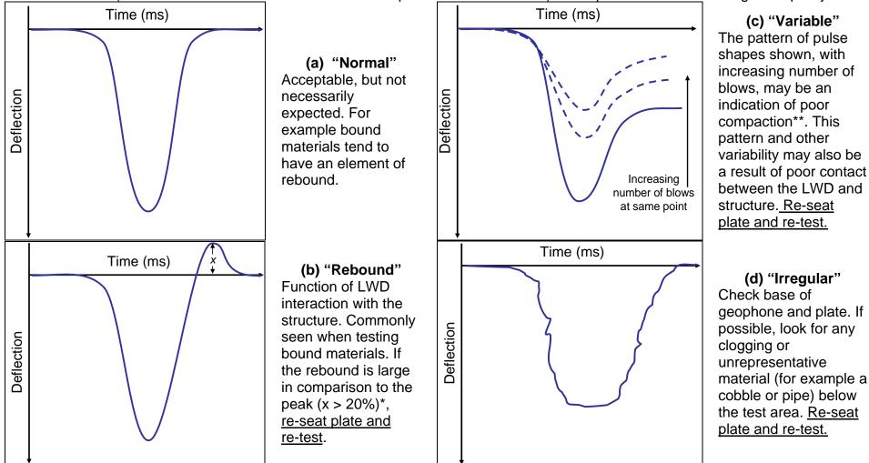
\* This arbitrary value is selected in the absence of other guidance. A lower value of x may be suitable for Foundation Class 1 and 2 (Unbound). \*\* LWD testing is not a proxy for measurement for adequate compaction (density), but can be used to highlight areas for further investigation
