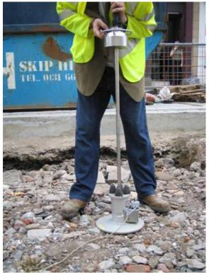
Figure 8 Testing on Large Particle Size Materials
