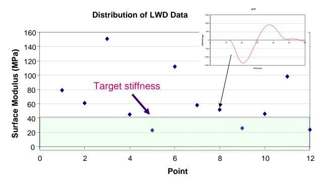
Figure 10 Sample Test Data (Note Failures at areas 5, 9 and 12, and although Point 8 is above the target stiffness examination of the signal response shows large rebound and therefore has failed)
