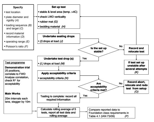
• Note: 200kPa contact stress requires a 20 kg mass with a 300mm diameter plate.
