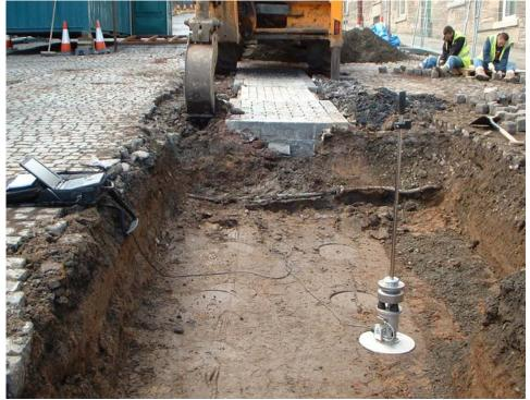
Figure 9 Shearing of Ground During Testing
