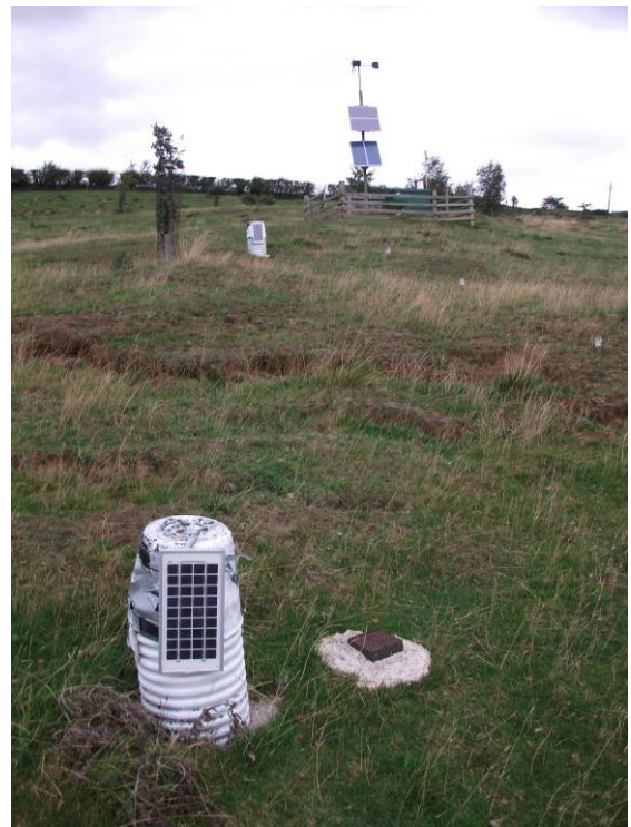
Figure 3. A view looking up the slope of the middle lobe with Cluster 1 acoustic waveguide protective cover and adjacent inclinometer casing in the foreground and Cluster 2 next to the small tree. BGS resistivity instrumentation compound and solar
