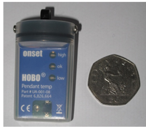
Fig. 2. Hobo data logger used to measure internal air temperature in 469 dwellings in Leicester City.
