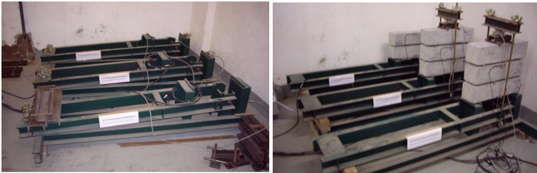
Figure 3 - Side view of the frame for the creep test (a), creep frame before (b) and after (c) loading.
