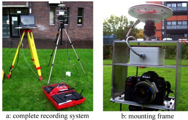
FIG. 1. Complete recording system and mounting frame.
