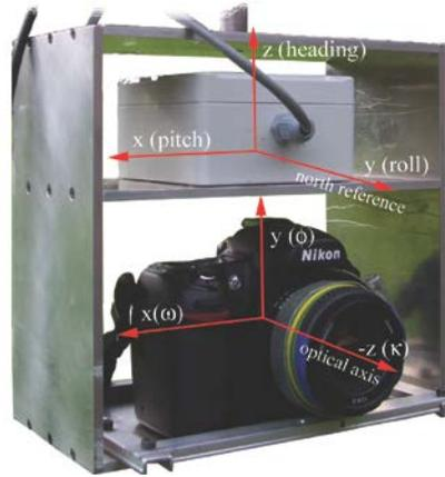
FIG. 5. Alignment of orientation sensor coordinate system with respect to the camera coordinate system (terrestrial orientation).
