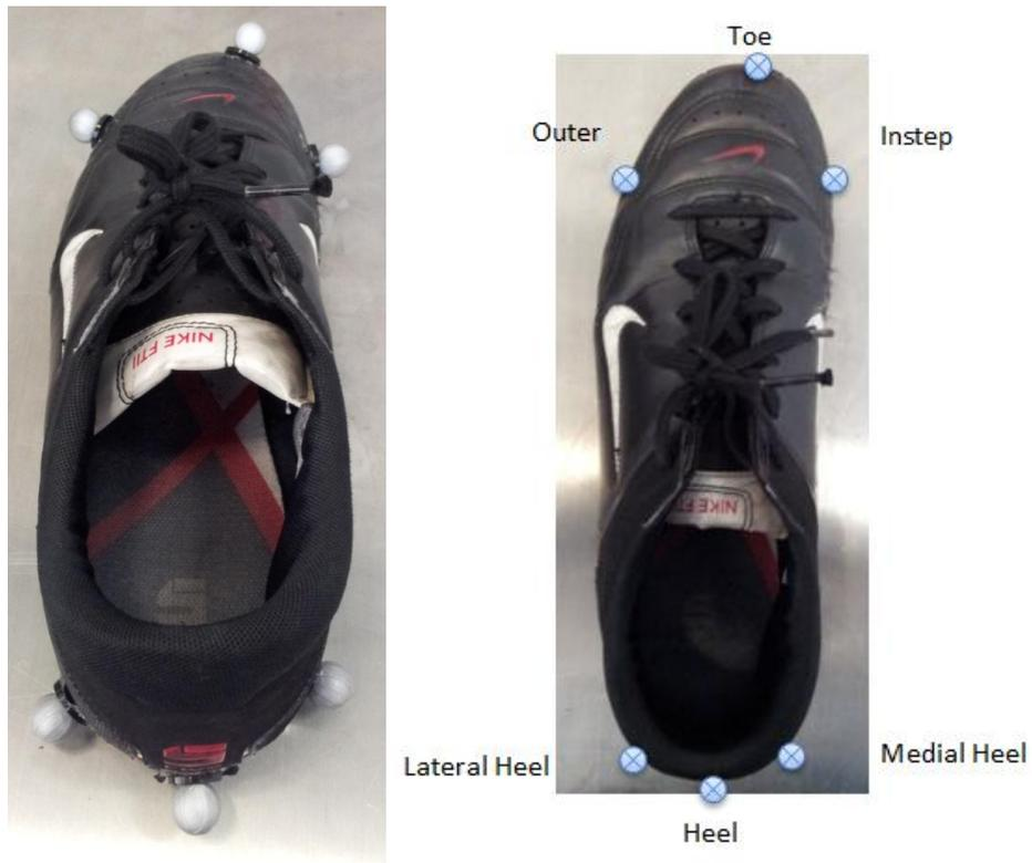
Figure 4.6: Position of markers on the left boot of player in the pilot experiment
