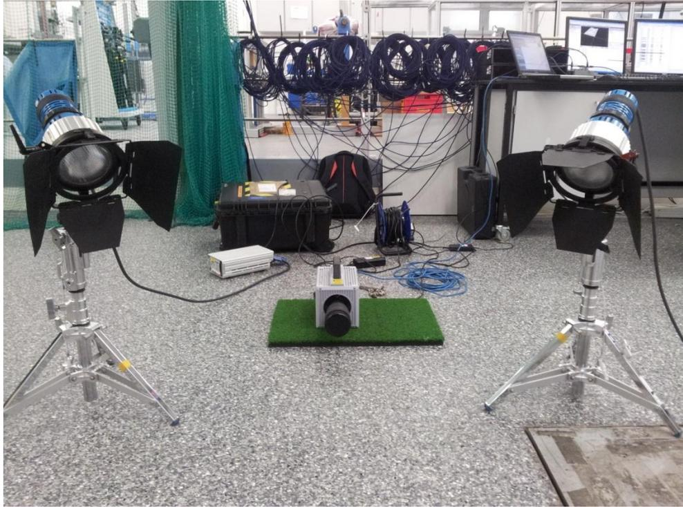
Figure 4.8: High speed camera with lighting system orientated laterally to the surface system
