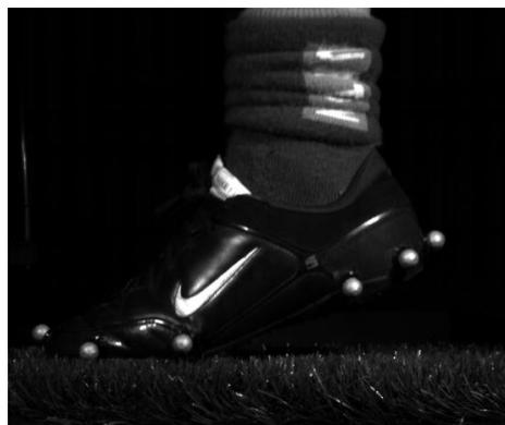
Figure 4.29: HSV footage shows the large surface deflection on 3G turf system at touchdown where the boot was inclined to the horizontal and boot-surface contact area was small
