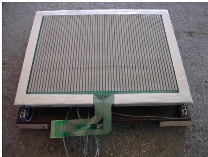
Figure 2.18: Tekscan Matscan system was mounted on top of a force plate (Carvalho et al., 2005)
