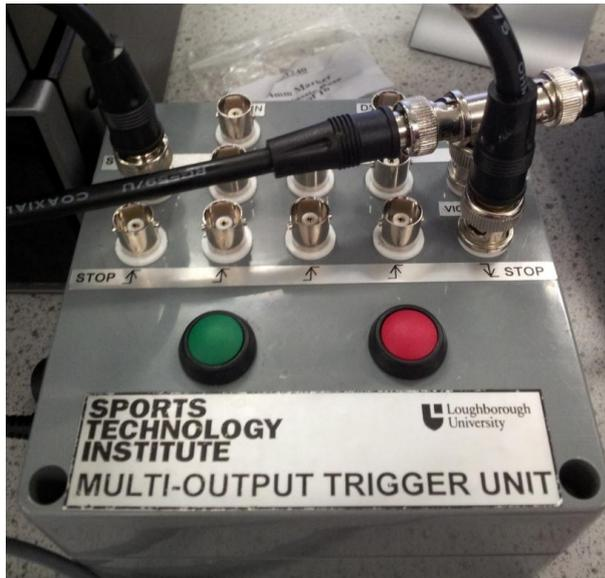
Figure 4.10: Multi-output trigger box for various devices (Vicon, force plate, pressure mat and high-speed camera)
