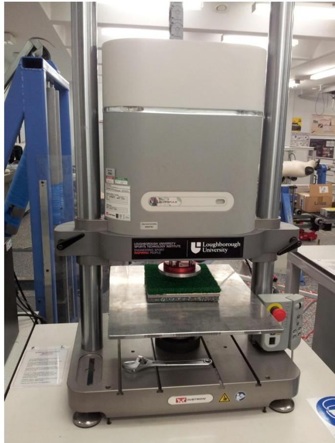
Figure 3.1: Instron ElectroPuls E3000 machine with sample
