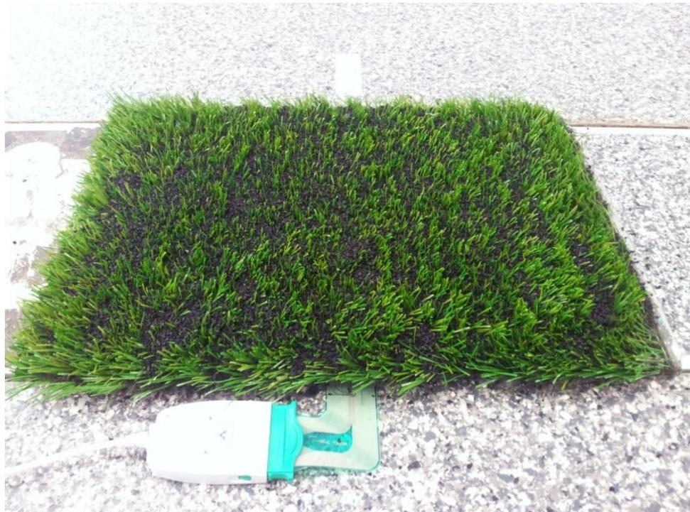
Figure 4.3: Schematic graph (above) and picture (below) of the pressure mat position in the measurement set-up
