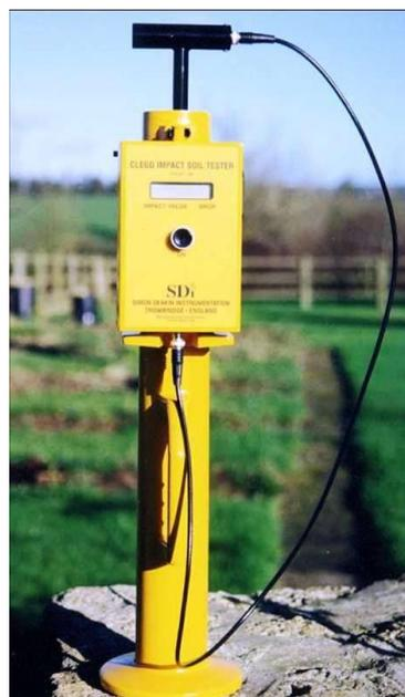
Figure 2.6: The Clegg Impact Hammer (Severn, 2010)
