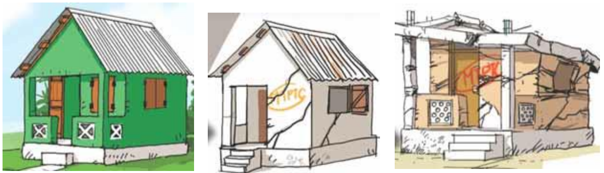
Figure 5.4 Demonstrates the 3 level coding system applied to the status of damage a house has undergone, presenting a sprayed tag ‘MTPTC’ in the respected code colour. [Source: IOM 2012]
