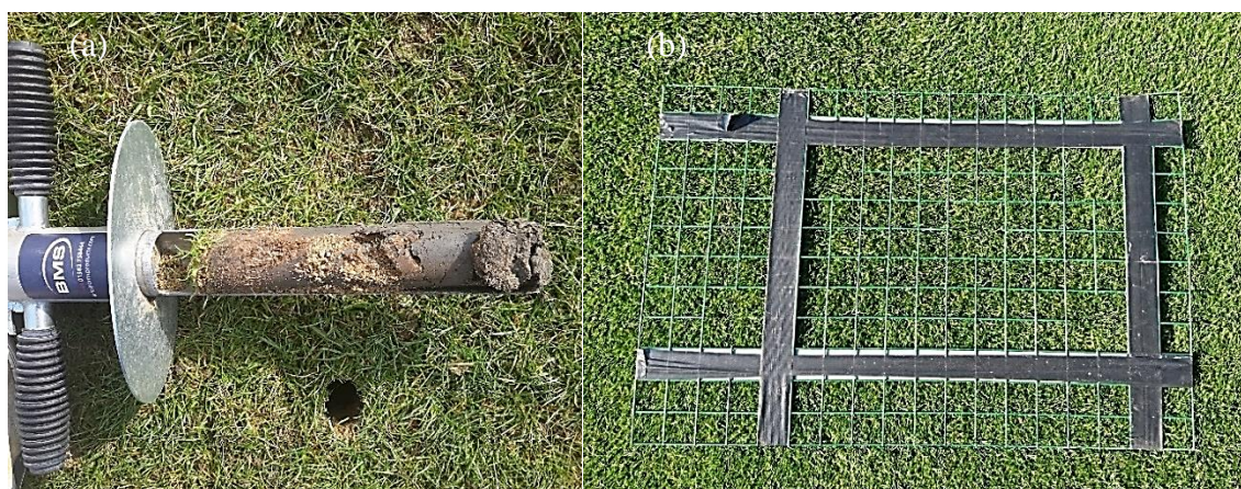
Figure 17 – The (a) corer and (b) quadrat
