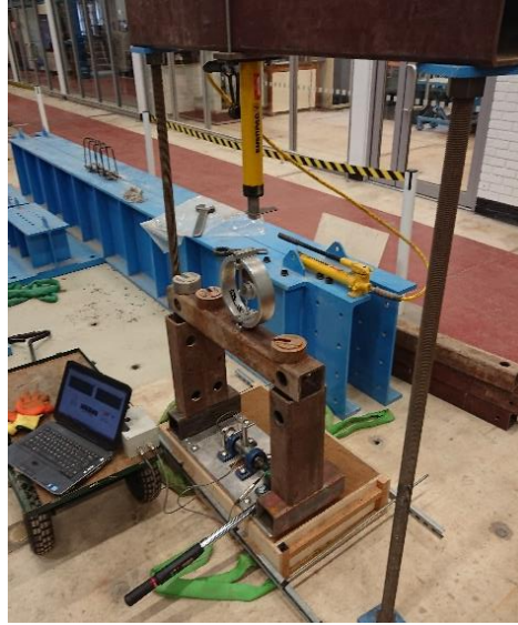
Figure 1 – The steel frame around the rig and the jack which applies the pressure to the sandy soil
