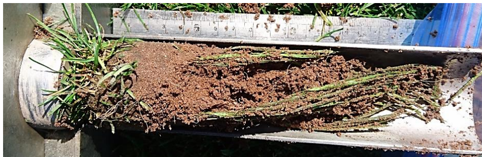
Figure 12 – A core of injected synthetic fibre construction
