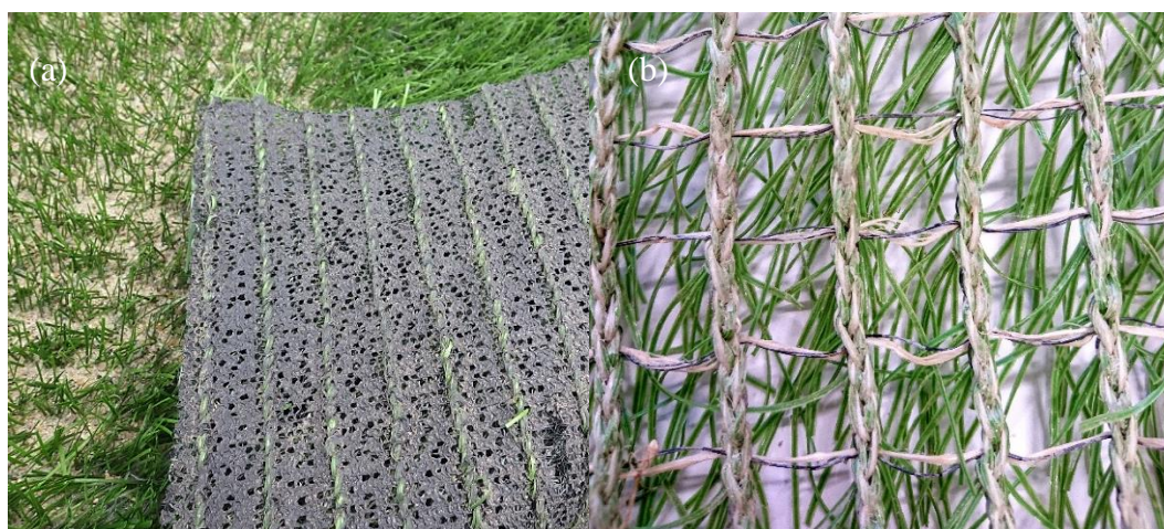
Figure 11 – Examples of (a) backing and (b) woven netted hybrid systems
