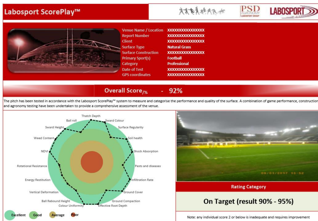
Figure 4 – An example of the Scoreplay™ result sheet showing the individual rating of each variable measured on a scale from poor to excellent and the resulting turf quality percentage
