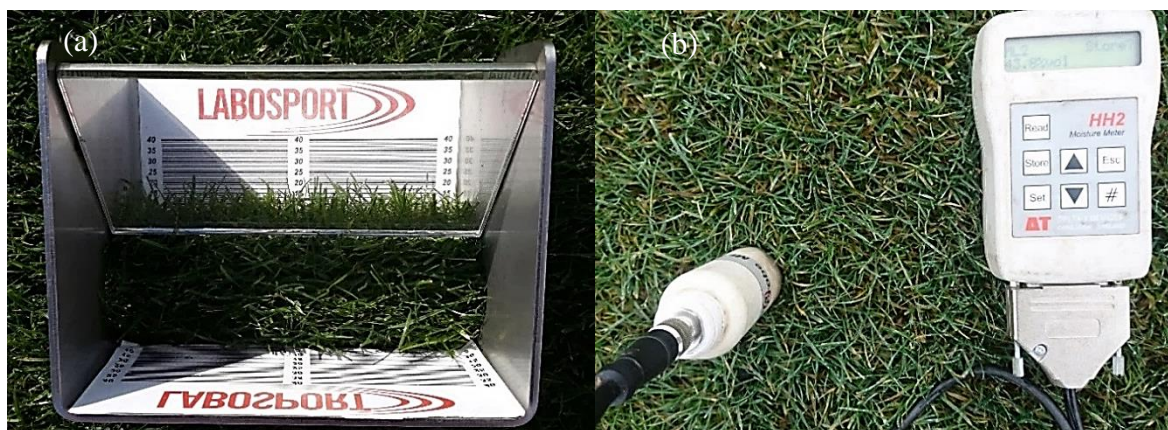
Figure 18 – (a) A mirrored prism to identify grass height and (b) a TDR moisture probe
