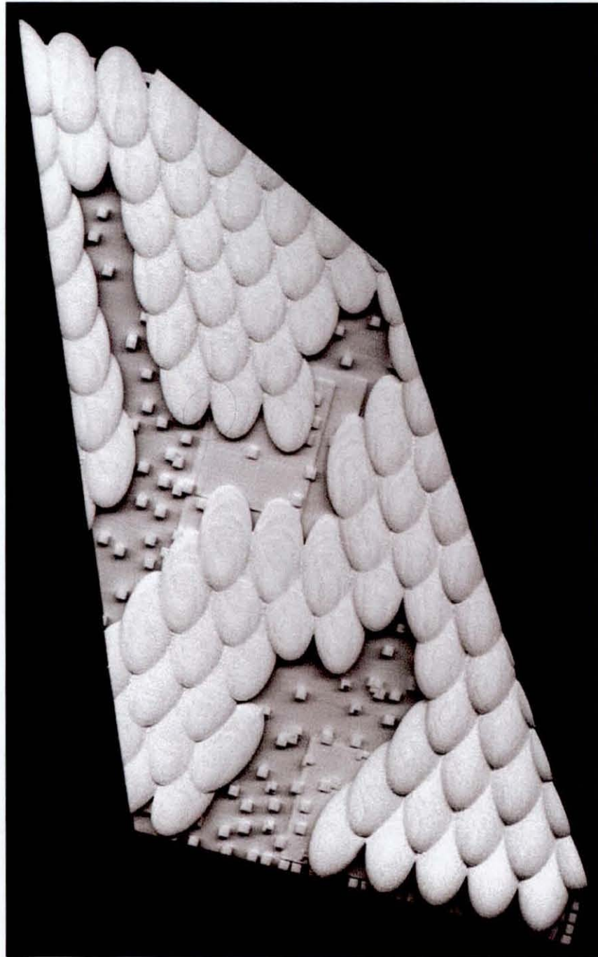
Figure 6.19 A, 'Rhino' modelled, sectioned Selective Laser Sintering (SLS) model of the Tactile Paving, showing an early version of how, by varying the density and distribution of a set of small 'magents' under the scaled top surface, the feel (the buoyancy) of the surface could be varied.
