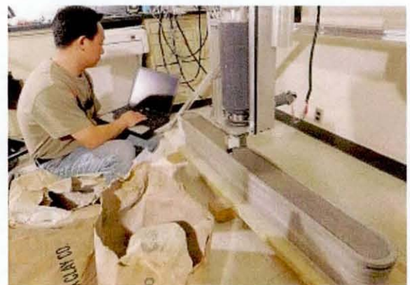
Figure 3.7 The Contour Crafting process by Behrokh Khoshnevis at USC. ( www.contourcrafting.com . Accessed September 2006).
