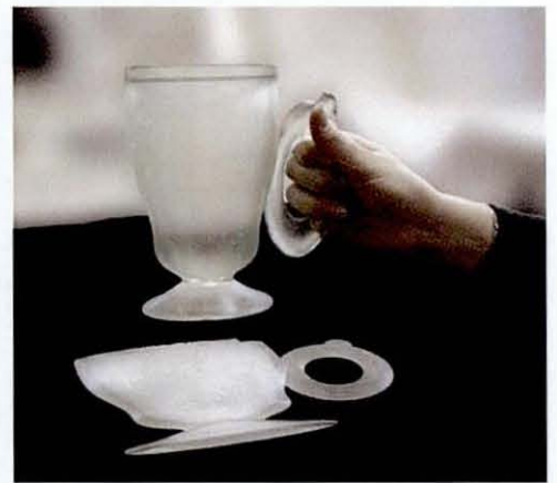
Figure 5.5 Clockwise from top left: Initial Rhino models of the Alice Cup designs; SLA builds of the pitcher and saucer renditions of the cup; FDM builds of the cream-pitcher, cappuccino cup and the espresso cup versions of the Alice Cup.
