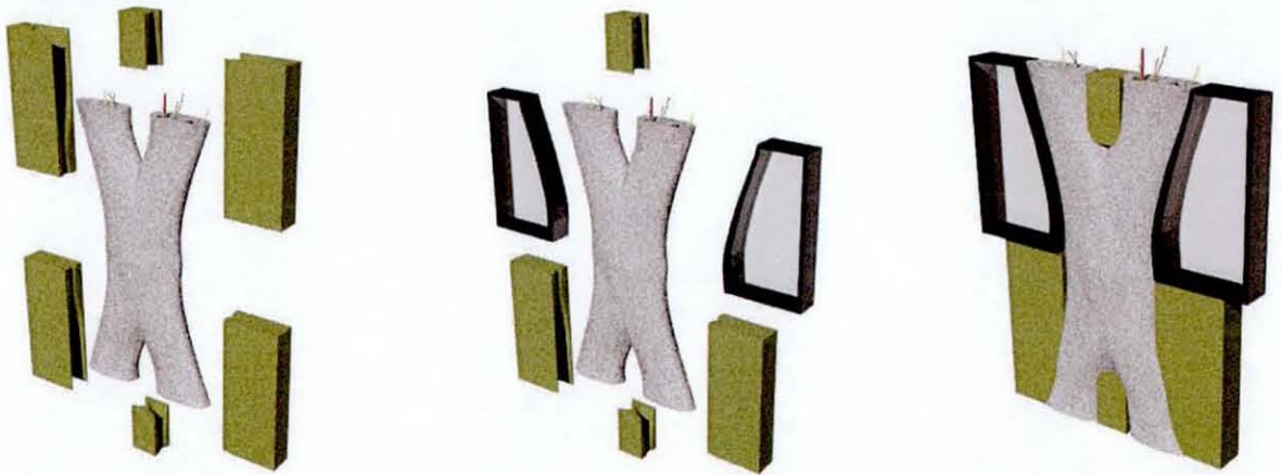
Figure 9.1 Features from the ‘Wonderwall’ project, exploring various hybrid systems that could be combined with the evolving additive (Freeform Construction) processes - a combination of fully bespoke (Layered Freeforming/ Freeform construction), semi-bespoke (transitional/ connective components), and generic (halbzeug/ mass produced) components and fabrication methods...
