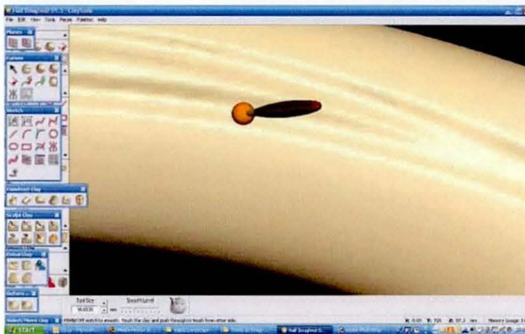
Figures 4.5 The Sensable device, through which one can feel the object displayed on the computer screen. A variety of different stylus heads can be used to shape the digital clay, Ranging from scalable spheres, rods, points, etc. to both 'push' as well as 'pull' (and even add or build) the surface.
