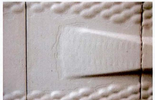
Figures 7.44 Textural close-ups of the Snakeskin 3DP build. Here both the 'stair-stepping' pattern of the fabrication process (3D Printing) as well as the edge 'softening', achieved in the Claytools software, can be observed...
