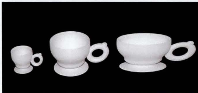
Figure 5.5 Clockwise from top left: Initial Rhino models of the Alice Cup designs; SLA builds of the pitcher and saucer renditions of the cup; FDM builds of the cream-pitcher, cappuccino cup and the espresso cup versions of the Alice Cup.
