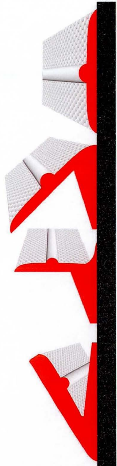
Figure 7.24 Sectional view of various angled positions for the Snakeskin relief strip.
