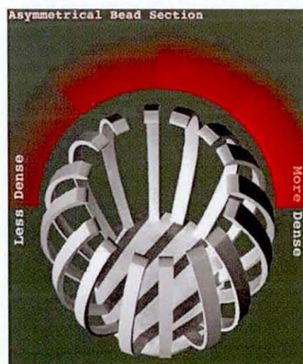
Figures 5.9 Left - A section view through an asymmetrical bead that has thicker ribs on one side, and a bit narrower ribs on the opposite. Right - The 'legend' bead for referencing the illustrations below.
