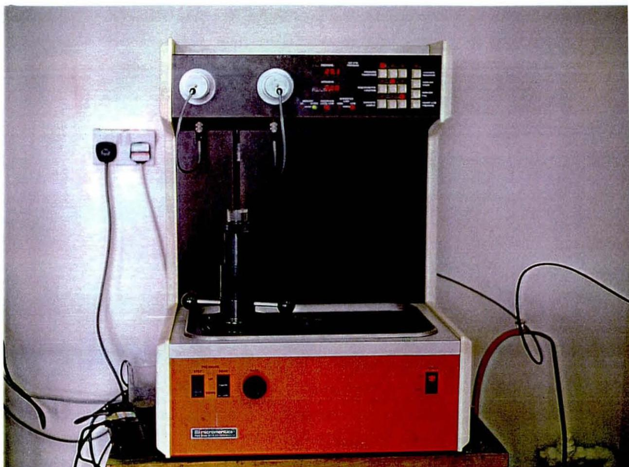
Fig. 4.8 Mercury intrusion porosimeter
