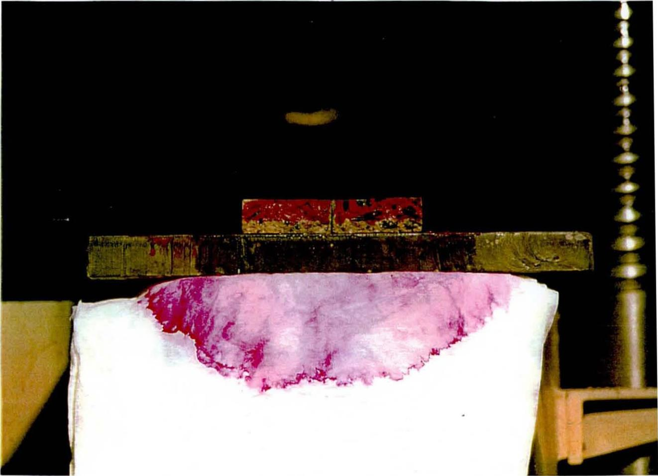
Fig. 4.5 Depth of carbonation by phenolphthalein pH indicator
