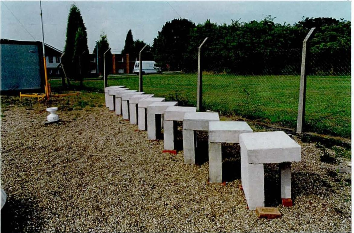
Fig. 3.2 Microclimate exposure arrangement of the blocks at the exposure site
