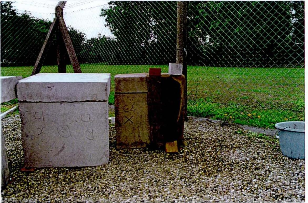
Fig. 3.3 Site curing arrangement of the blocks (2 curing methods per block)
