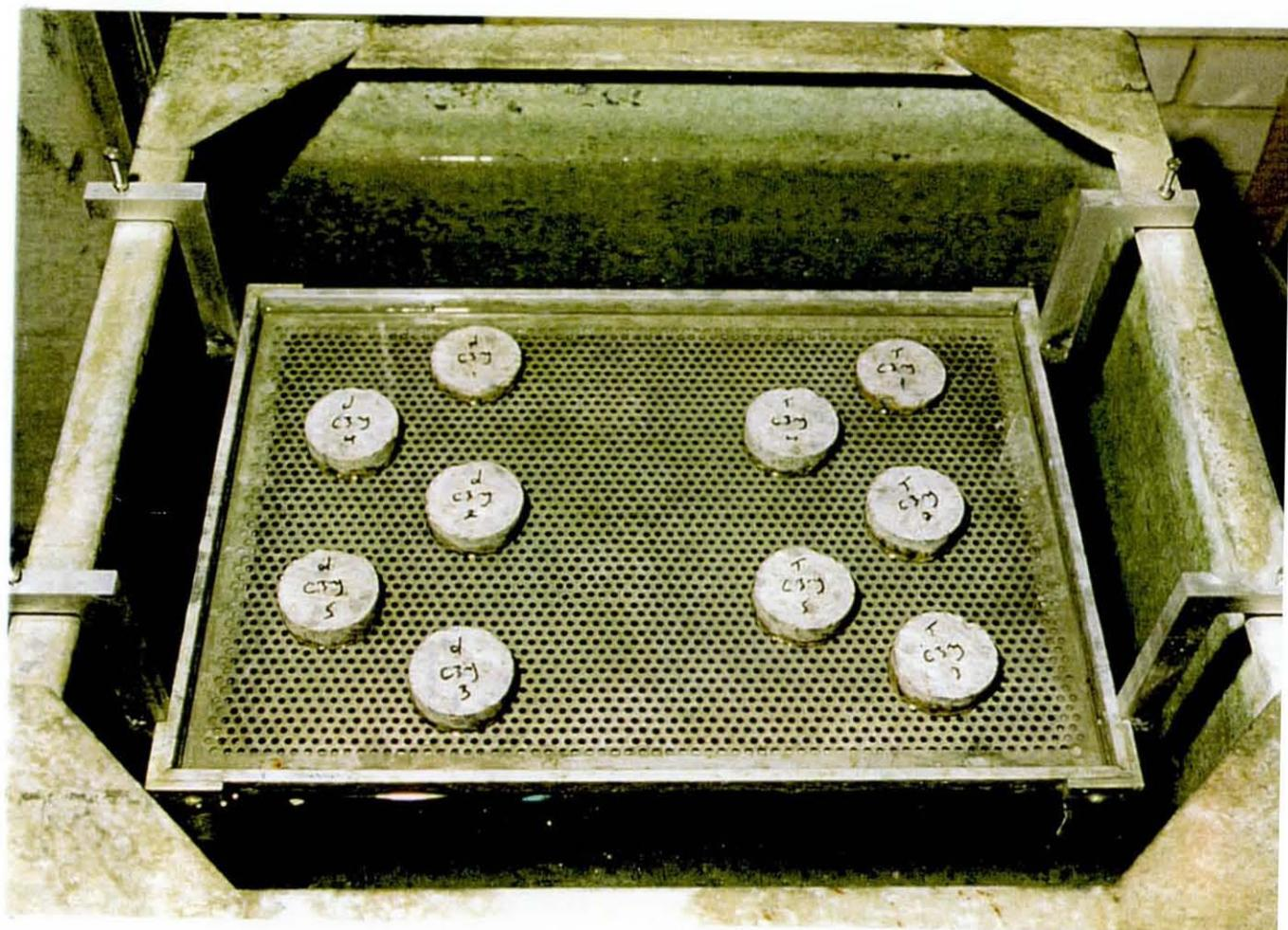
Fig. 4.4 Sorptivity test apparatus
