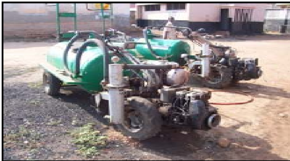
Picture 5.1: Larsen Dung Beetle for Emptying Bucket Latrines in Accra
