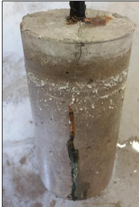
Figure 4.19 Typical cracking of 200mm x 100mm diameter reinforced concrete cylinder
