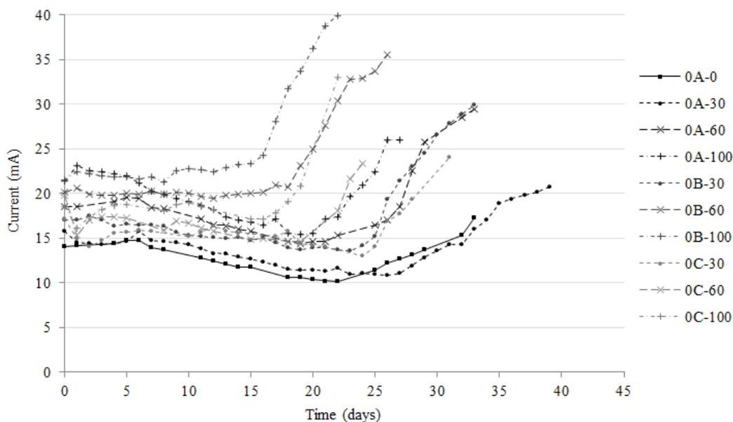
Figure 8 - Time to corrosion initiation and cracking (CEM I, 91 days)
