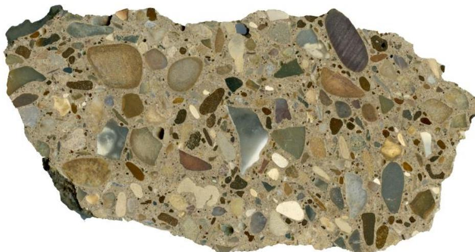
Figure 1 - Thin section of demolition concrete for petrographic analysis [46]
