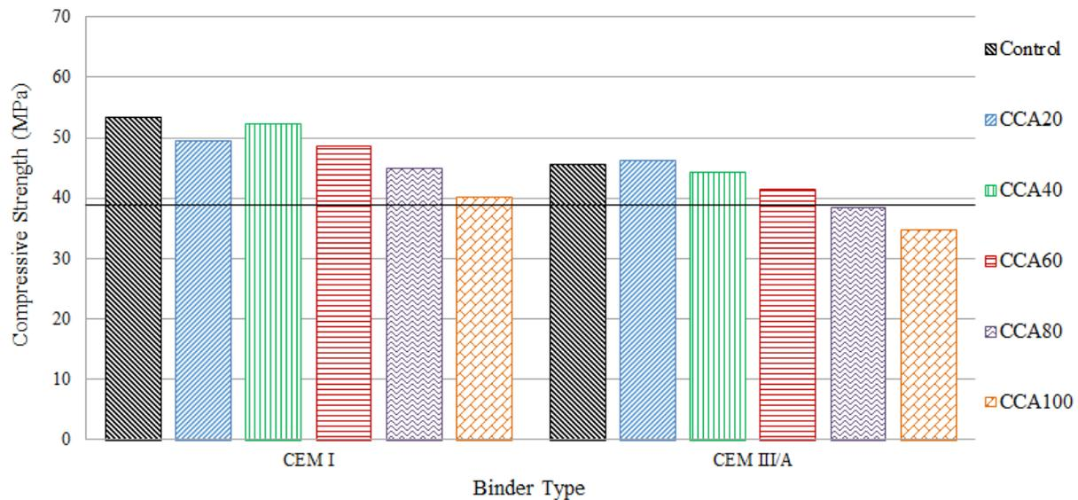
**Figure 4.7 Compressive cube strength at 28 days**
