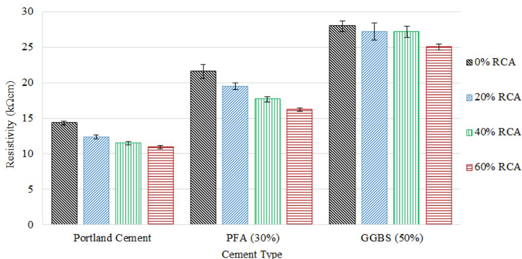
Figure 3 – Concrete surface resistivity at 28 days
