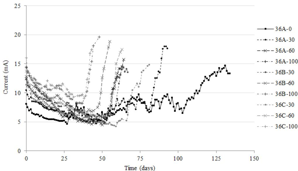
Figure 9 - Time to corrosion initiation and cracking (CEM III/A, 36% GGBS, 28 days)
