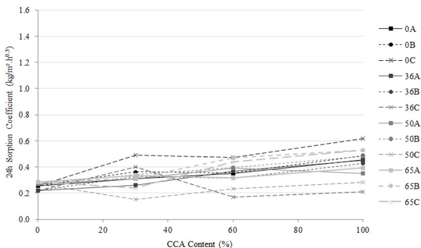
Figure 8 - 24hr Sorption coefficient at 28 days
