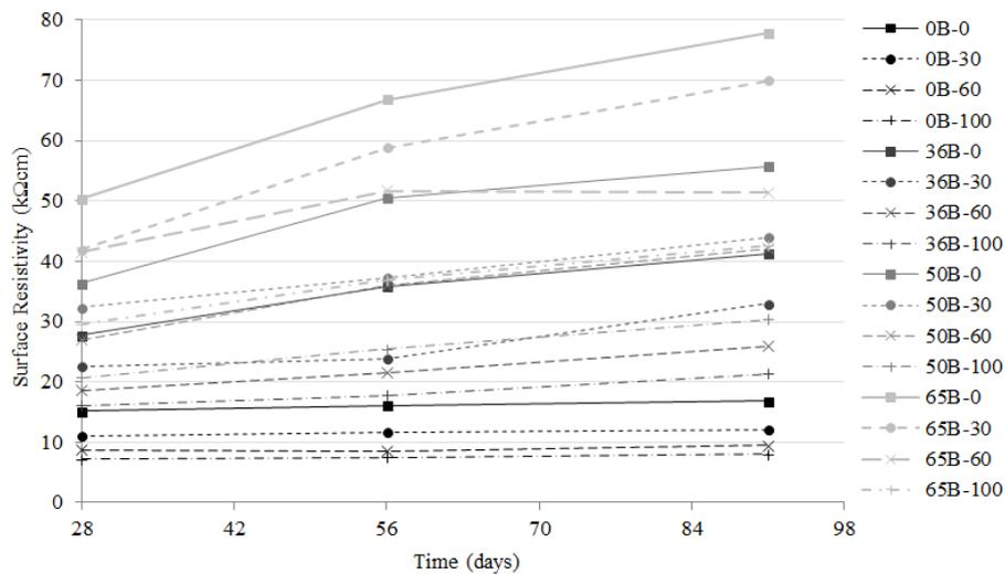
Figure 5 - Surface resistivity for source B concretes
