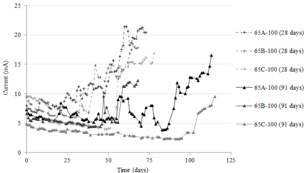
Figure 12 - Time to corrosion initiation and cracking (CEM III/A, 65% GGBS, 28 and 91 days)
