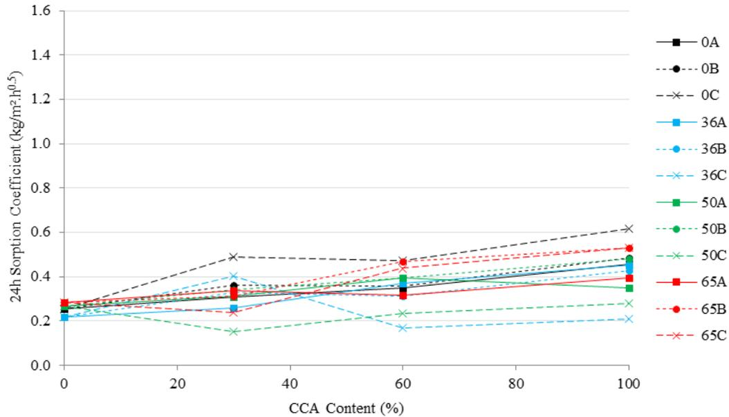
Figure 4.16 24hr Sorption coefficient at 28 days
