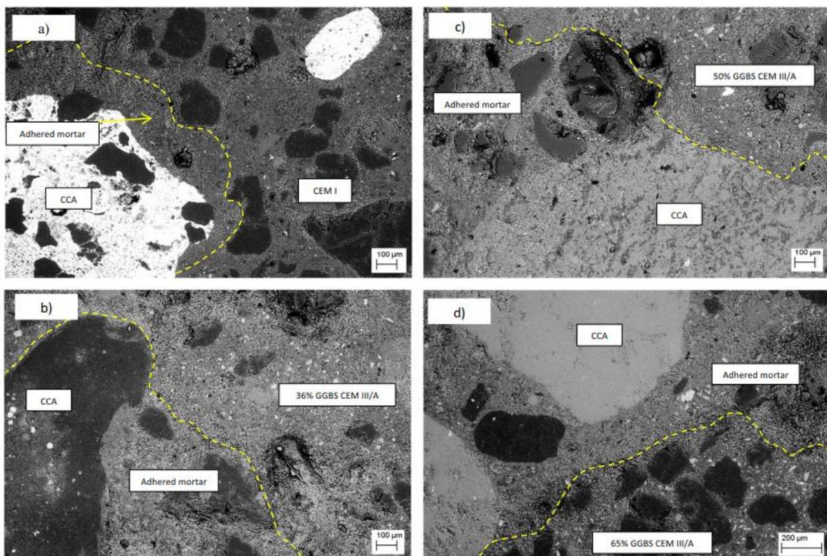
**Figure 4.18 SEM high resolution images for a) CEM I, b) 36% GGBS, c) 50% GGBS and d) 65% GGBS CCA concretes**
