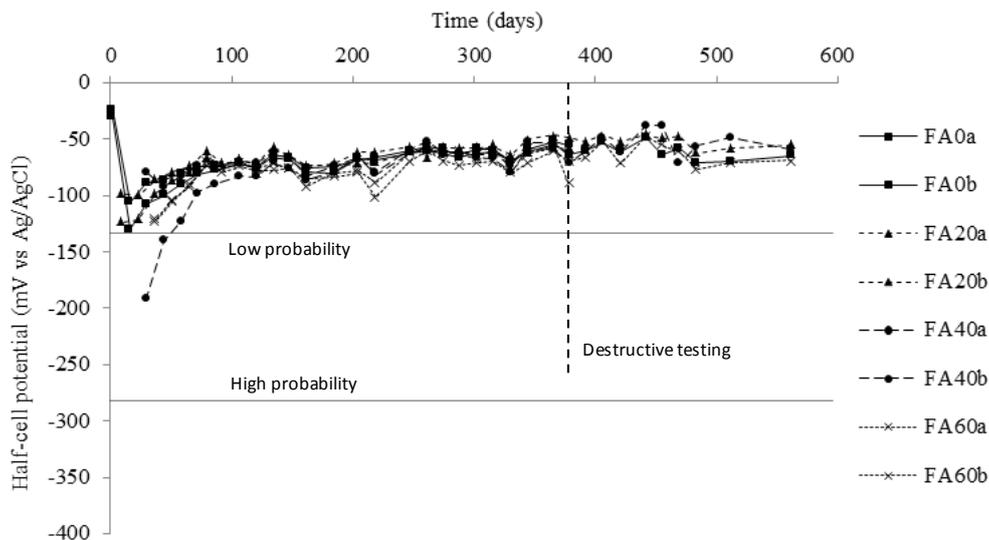
Figure 7 - Development of ‘wet’ half-cell potential over time, CEM II/B-V concrete
