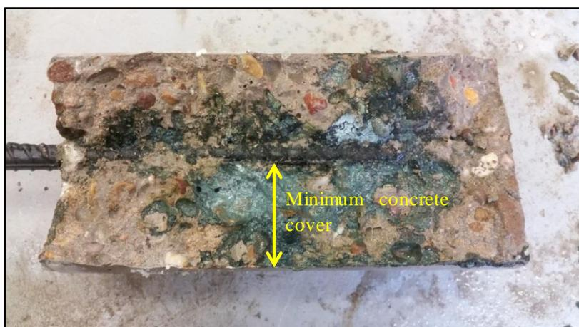
Figure 4 - Measurement of cover depth and development of 'green rust' precipitate
