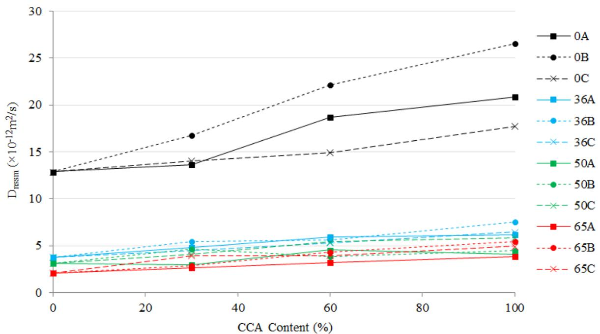
Figure 4.20 Rapid chloride migration coefficient ( $D_{nssm}$ ) at 91 days
