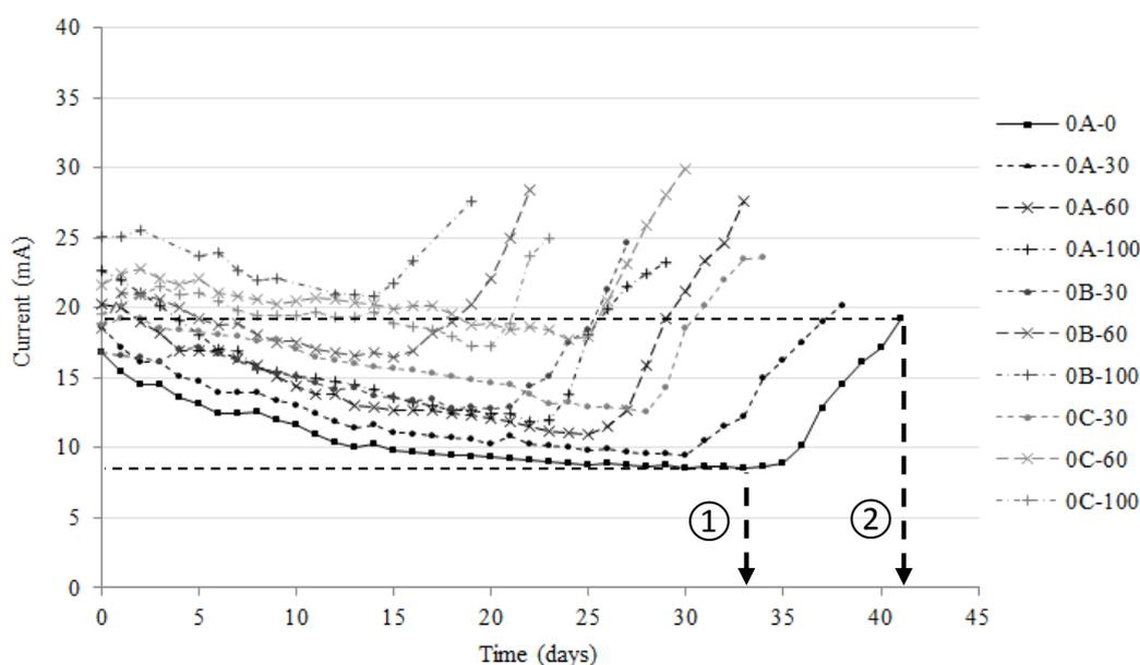
Figure 7 – Time to corrosion initiation and cracking (CEM I, 28 days)
