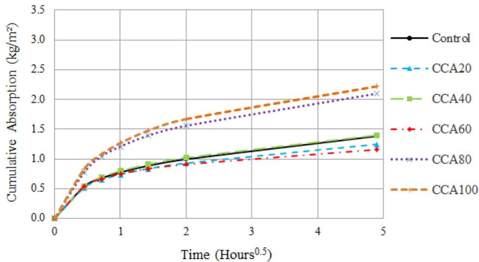
Figure 4.11 Cumulative sorption at 28 days for CEM III/A concrete
