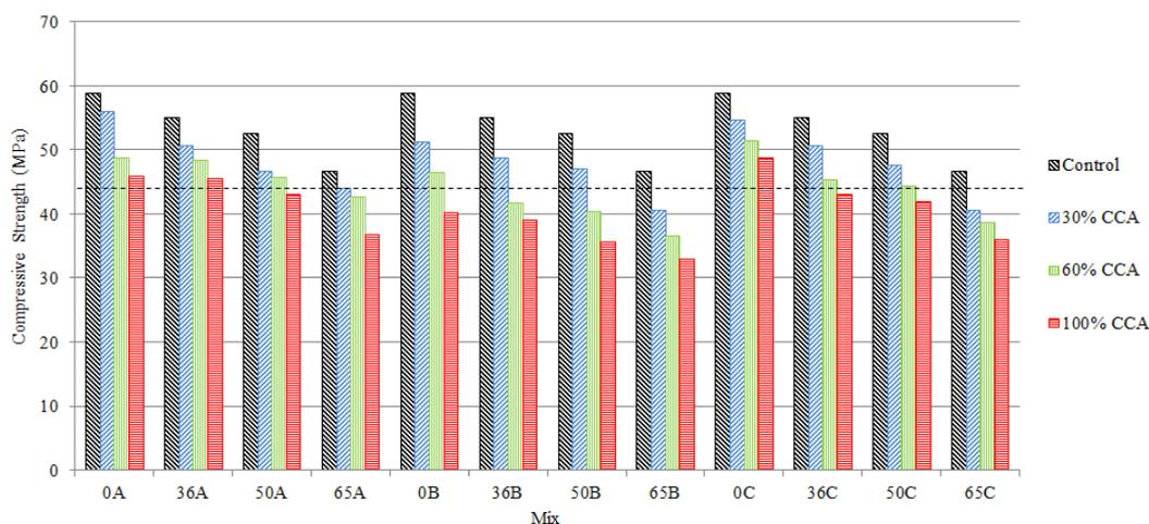
Figure 1 - Compressive cube strength at 28 days
