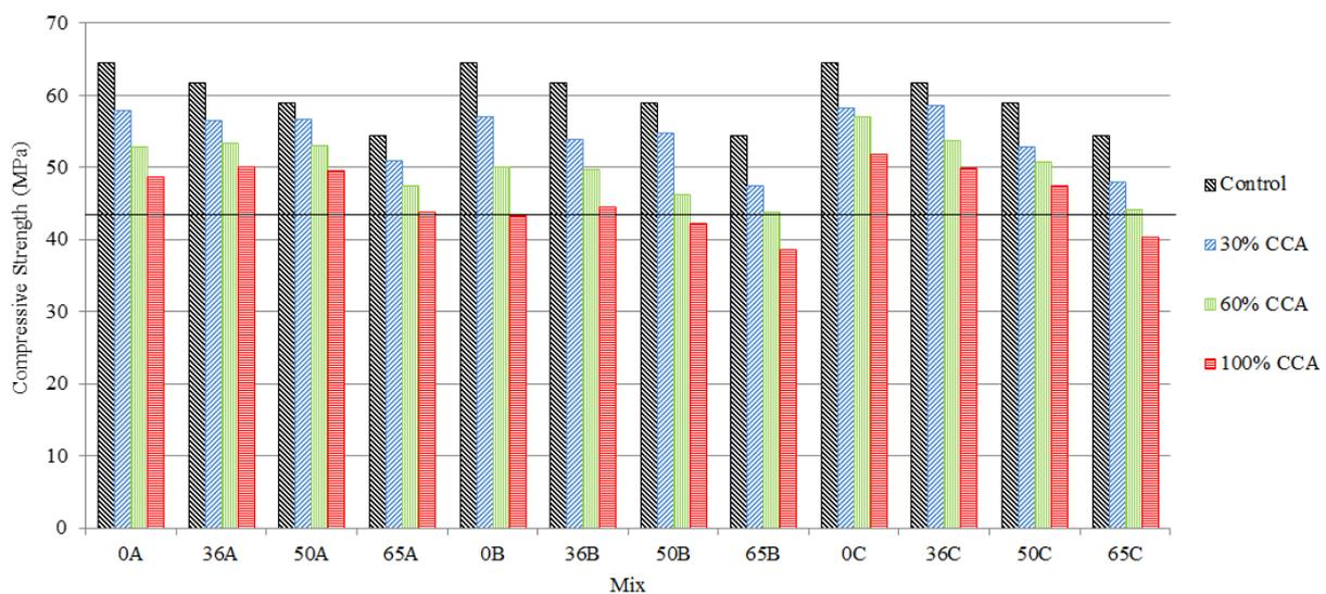
**Figure 4.15 Compressive strength at 91 days**
