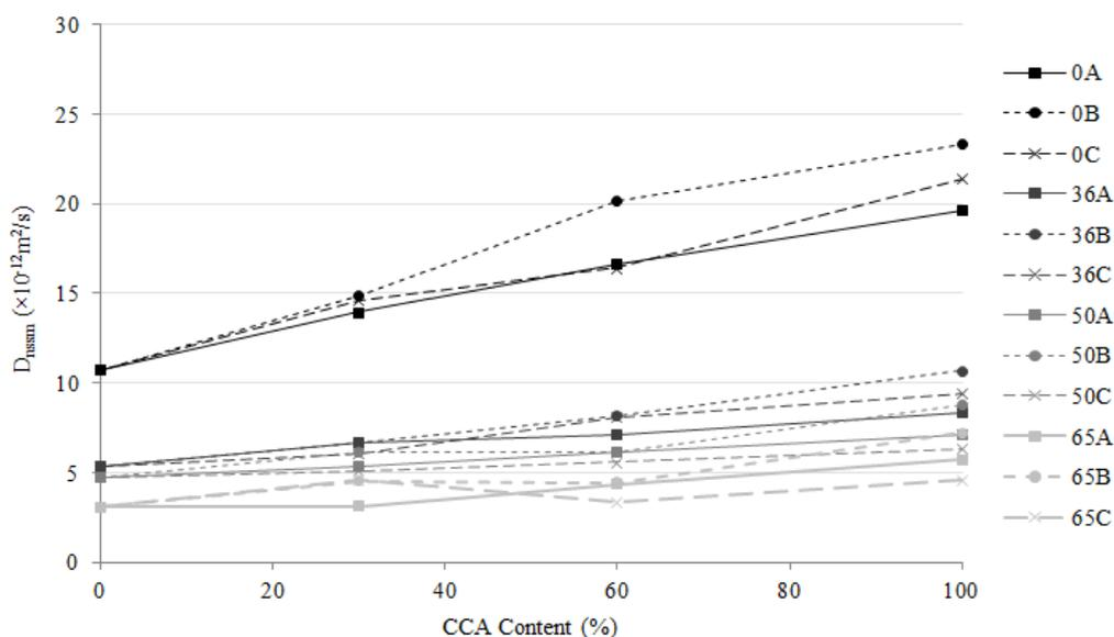
Figure 5 – Rapid chloride migration coefficient ( $D_{nssm}$ ) at 28 days
