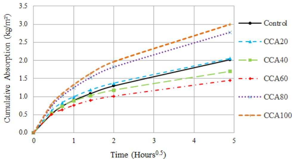
Figure 4.10 Cumulative sorption at 28 days for CEM I concrete
