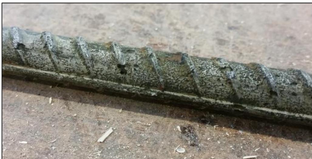
Figure 2 - Chloride induced ‘pitting’ corrosion of reinforcing steel
