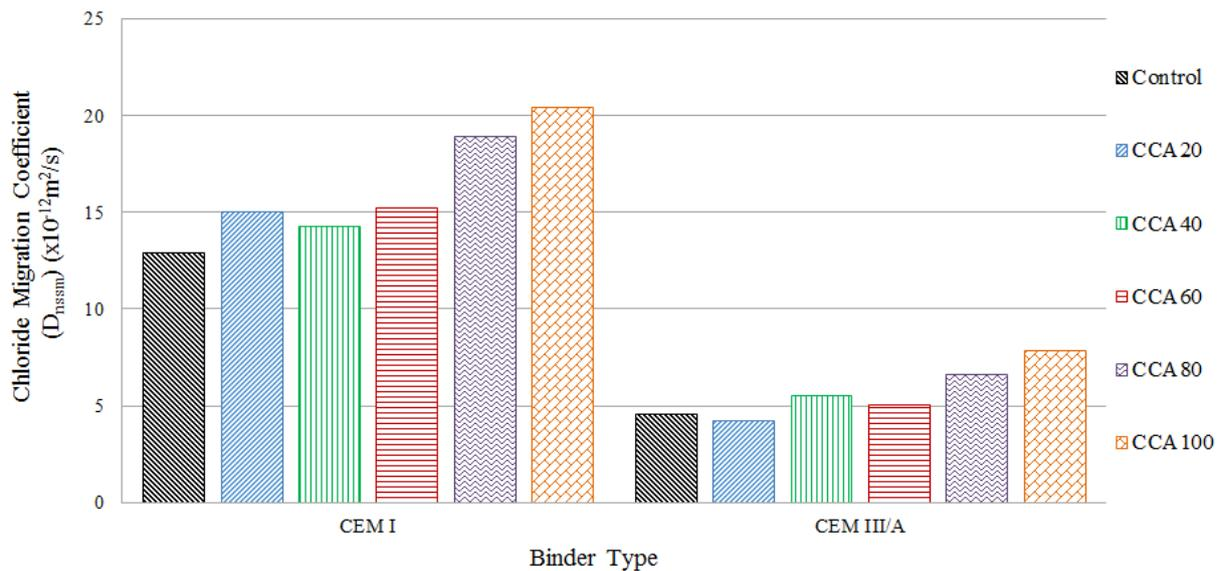
Figure 4.9 Rapid chloride migration coefficient at 28 days
