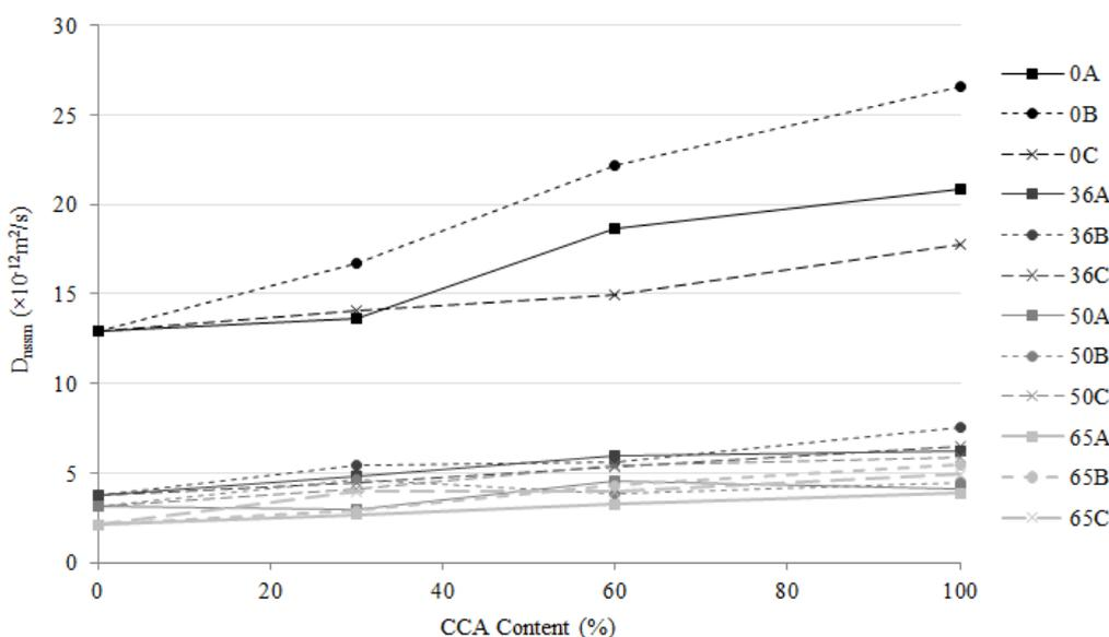
Figure 6 - Rapid chloride migration coefficient ( $D_{nssm}$ ) at 91 days
