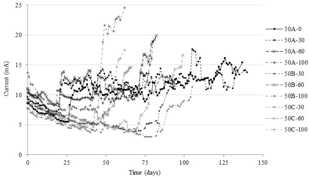
Figure 10 - Time to corrosion initiation and cracking (CEM III/A, 50% GGBS, 28 days)
