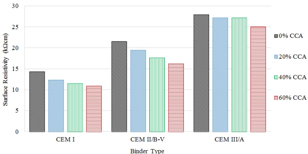
Figure 4.3 Surface resistivity at 28 days
