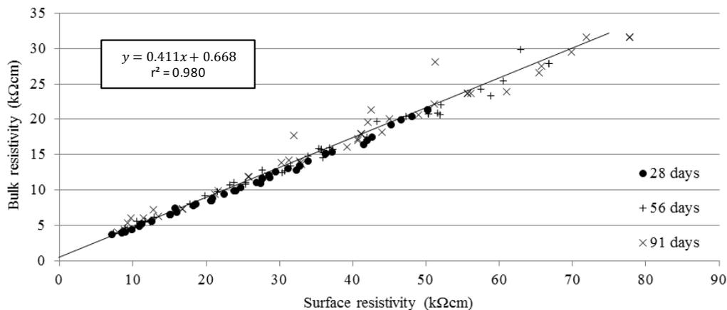
Figure 7 - Correlation between surface and bulk resistivity
