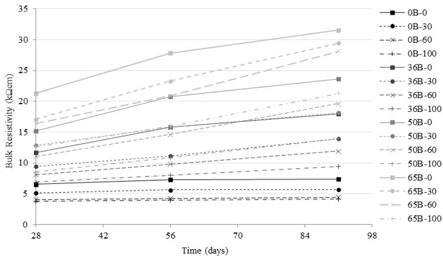
Figure 6 - Bulk resistivity for source B concretes
