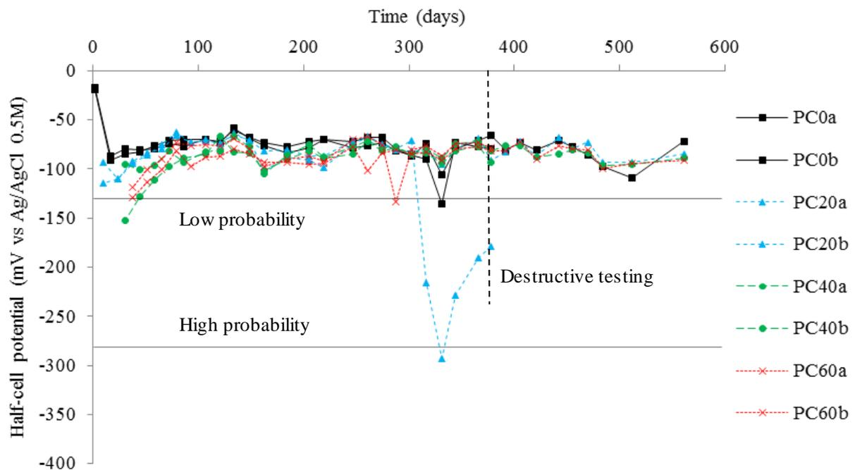
Figure 4.4 Half-cell potential development over time, CEM I concrete
