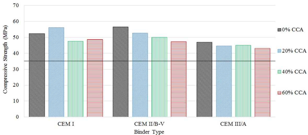
Figure 4.2 Compressive cube strength at 28 days
