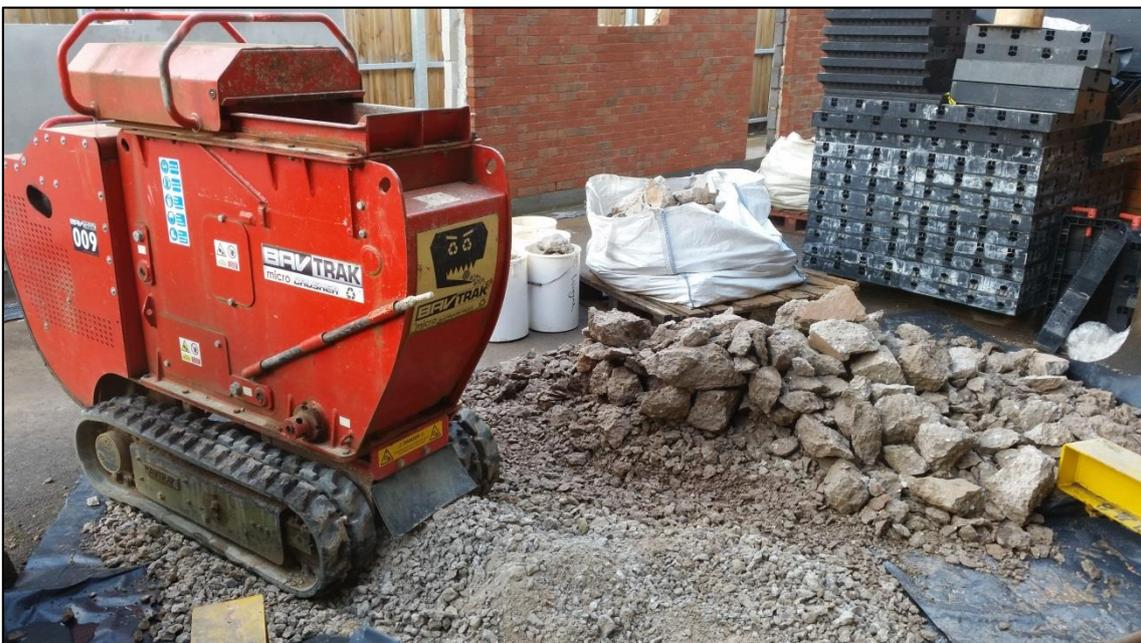
**Figure 4.14 Micro-crusher used to produce a 40mm down product from larger sections**
