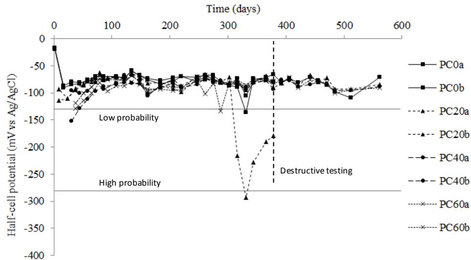
Figure 6 - Development of ‘wet’ half-cell potential over time, CEM I concrete
