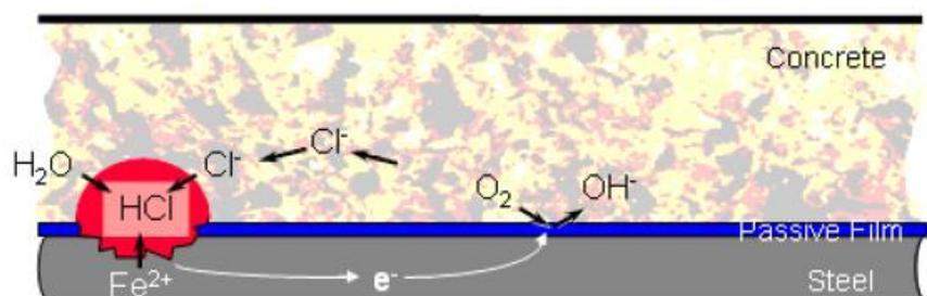
Figure 1 - Electrochemical process of chloride induced corrosion (Glass *et al*, 2006)
