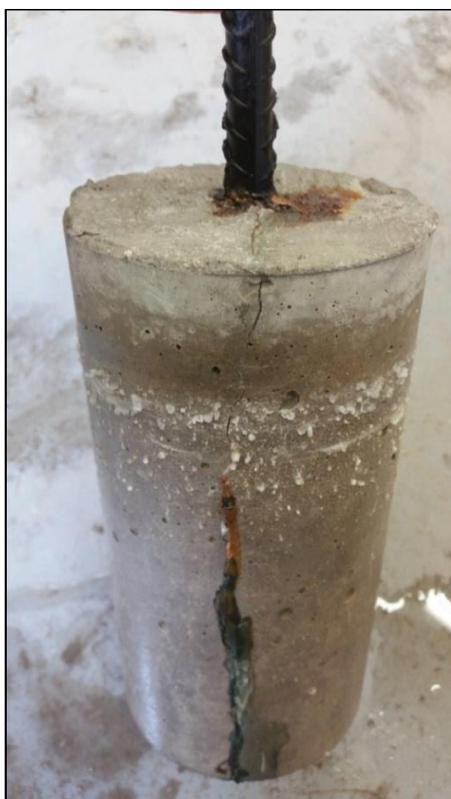
Figure 3 - Typical cracking of 200mm × 100mm diameter reinforced concrete cylinder
