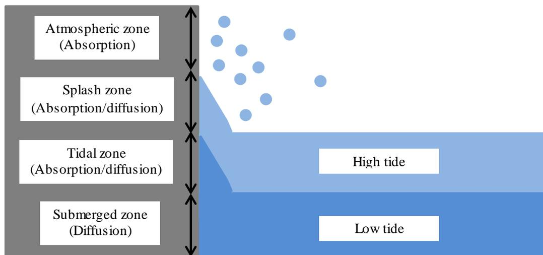
**Figure 1.5 Different zones of exposure for marine structures (Dyer, 2014)**
