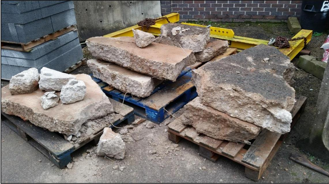
**Figure 4.13 Reinforced concrete ground floor slab sections of CCA**
