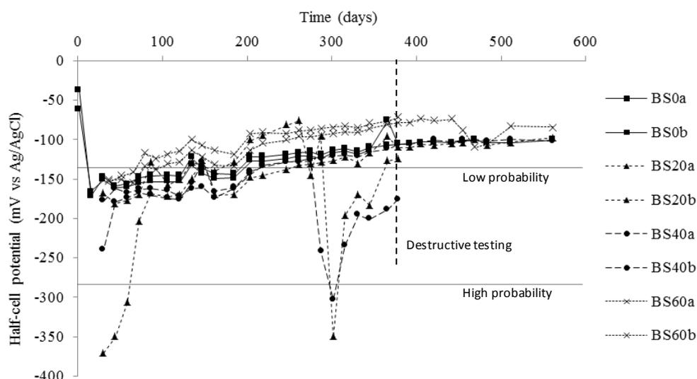
Figure 8 - Development of 'wet' half-cell potential over time, CEM III/A concrete
