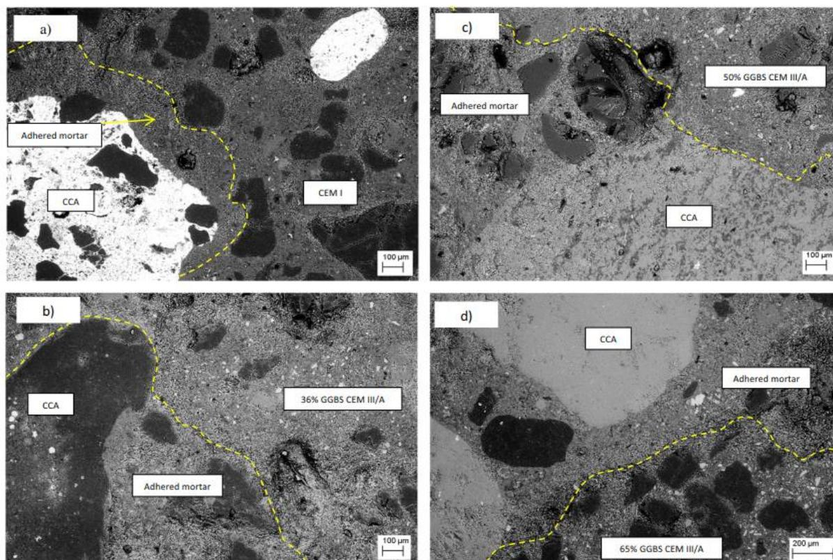
Figure 11 - SEM high resolution images for a) CEM I, b) 36% GGBS, c) 50% GGBS and d) 65% GGBS CCA concretes
