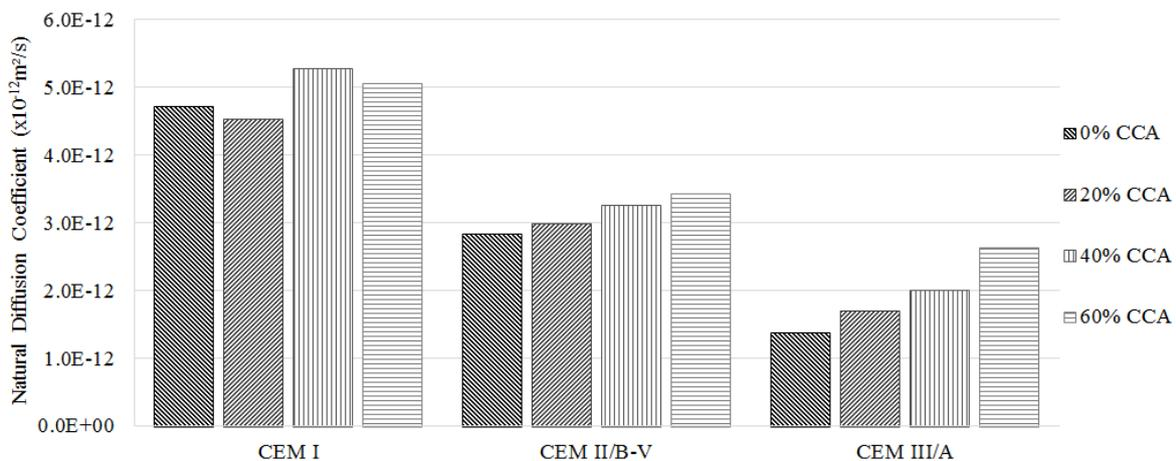
Figure 14 - Natural diffusion coefficients following a 90 day exposure to chloride ion solution
