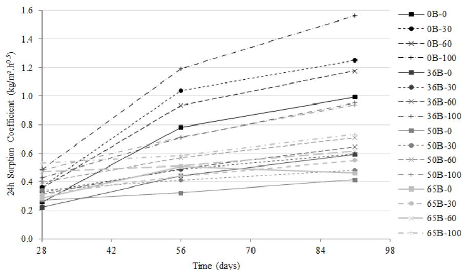
Figure 10 - 24hr Sorptivity coefficient for source B concretes
