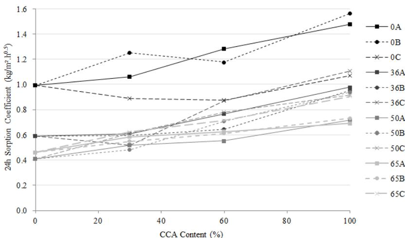
Figure 9 - 24hr Sorption coefficient at 91 days
