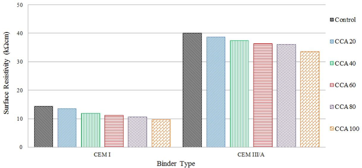
Figure 4.8 Surface resistivity at 28 days
