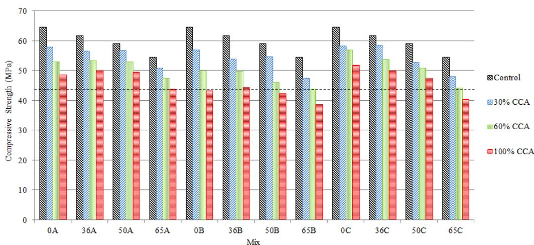
Figure 2 - Compressive cube strength at 91 days
