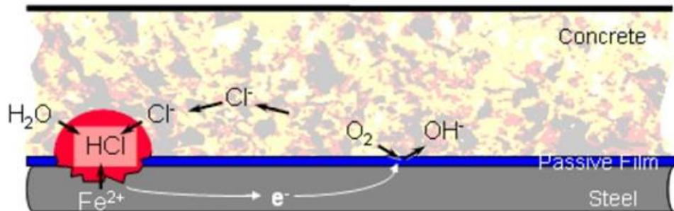
**Figure 1.6 Electrochemical process of chloride-induced corrosion (Glass *et al*, 2006)**
