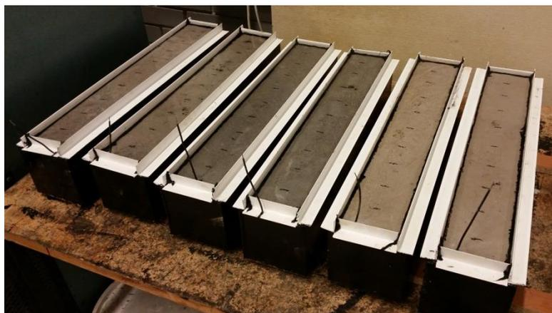
Figure 2 – Reinforced concrete beams prepared for cyclic wetting/drying
