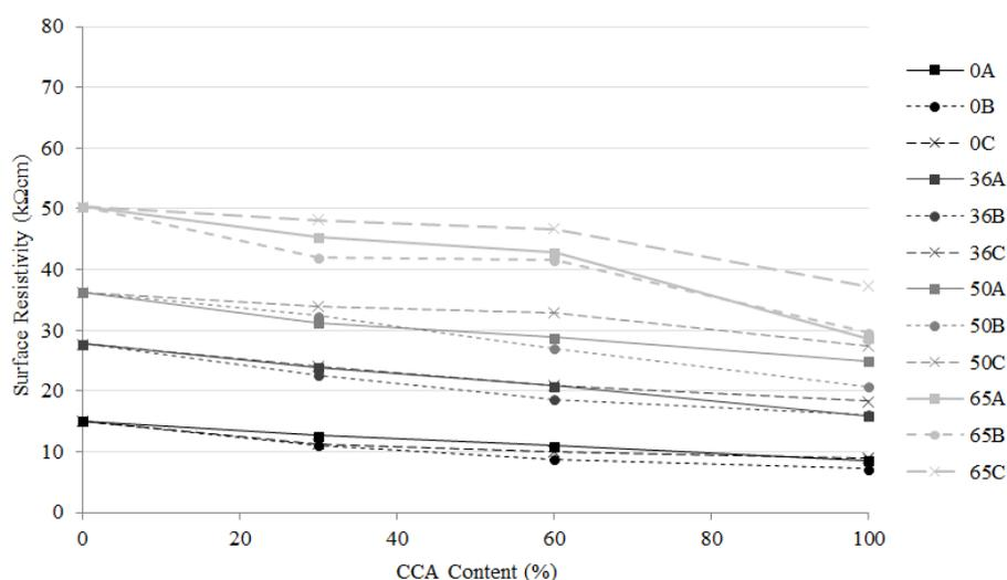
Figure 3 - Surface resistivity at 28 days
