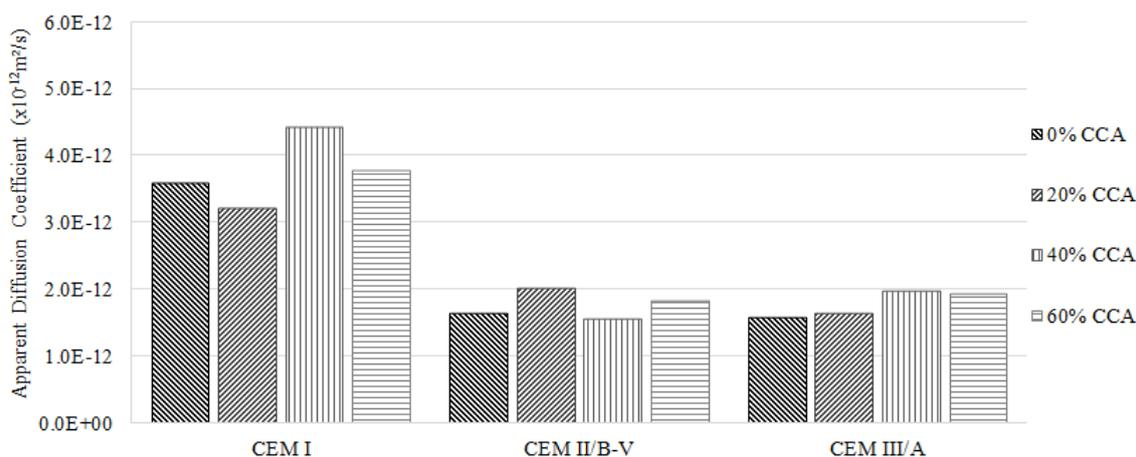
Figure 12 - Apparent diffusion coefficient following 12 month exposure to cyclic wetting/drying
