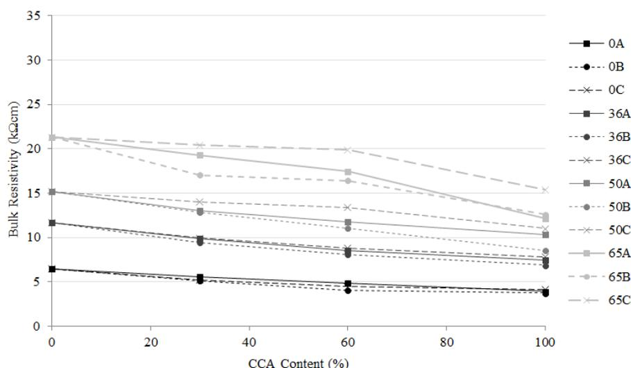
Figure 4 - Bulk resistivity at 28 days
