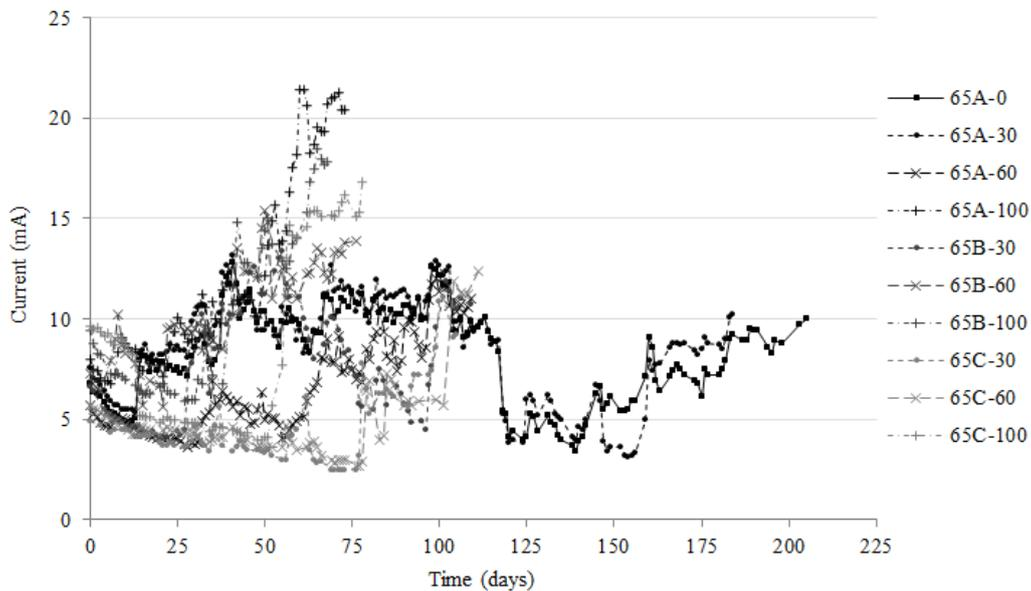
Figure 11 - Time to corrosion initiation and cracking (CEM III/A, 65% GGBS, 28 days)
