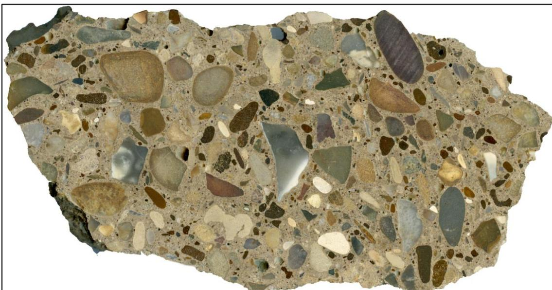
**Figure 4.6 Section of CCA source concrete for petrographic analysis**
