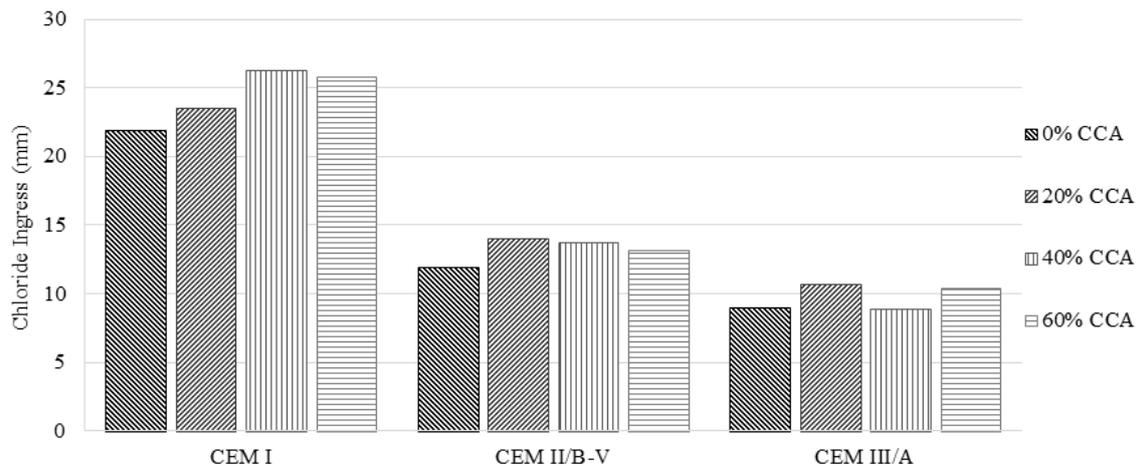
Figure 13 - Chloride ion ingress following 12 month exposure to cyclic wetting/drying
