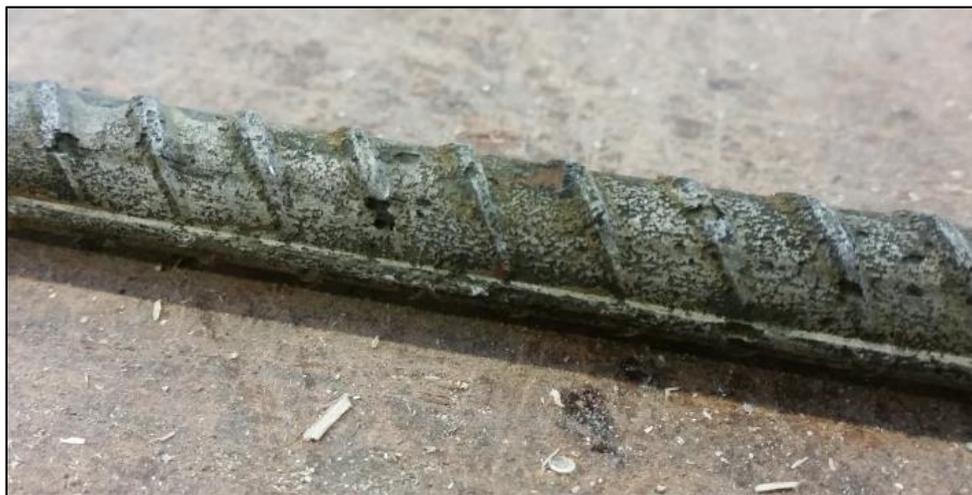
**Figure 1.7 Chloride-induced 'pitting' corrosion of reinforcing steel**
