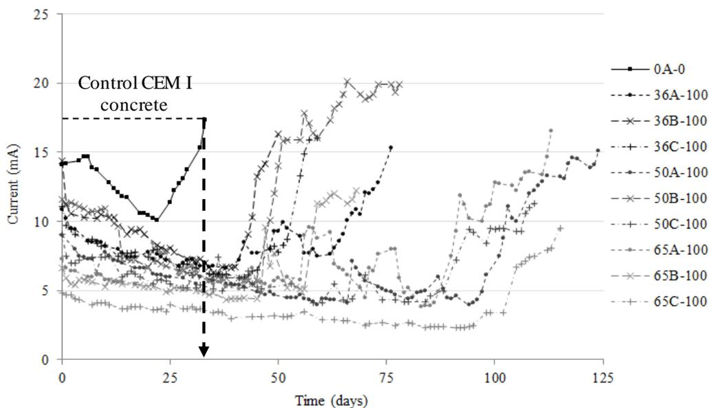
Figure 13 - Time to corrosion initiation and cracking (91 days)
