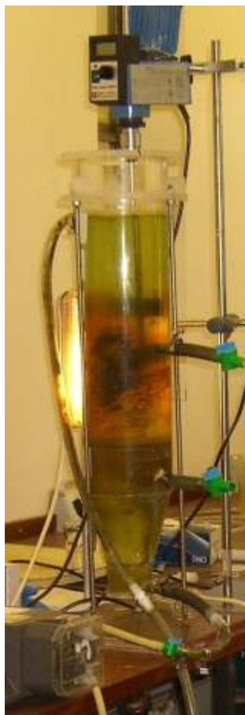
Figure 3 - The bioreactor with light and mechanical stirrer
