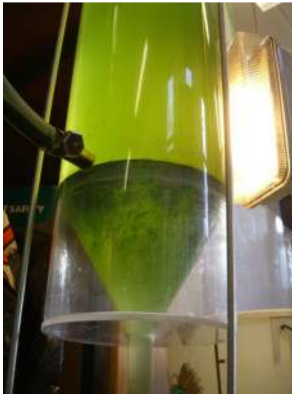
Figure 7 - Detail of the conical base
