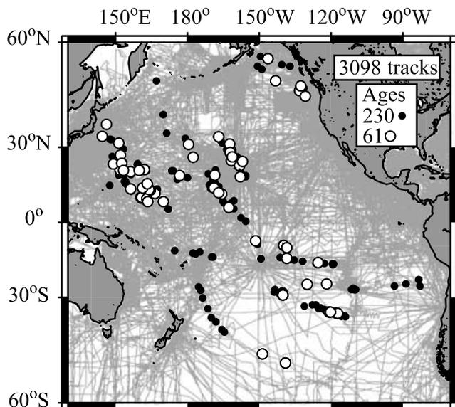
**Figure 1.** Locations of data sets. Grey lines are echo-sounder data, mainly from the GEODAS database (NOAA 2003). 230 black dots are better quality radiometric dates from seamounts: Koppers *et al.* (2003) supplemented by Clouard & Bonneville (2005). 61 white circles overlie some of these where there are also geophysical strength estimates in this study (see Section 2.3).
