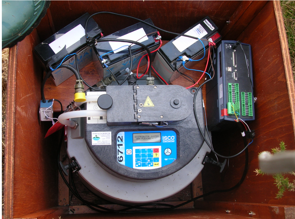
Plate 4.3: ISCO 6712 water sampler (mine station)
