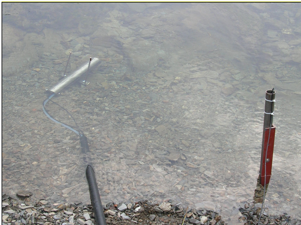
Plate 4.2: Protective probe casing and sample actuator (mine station)
