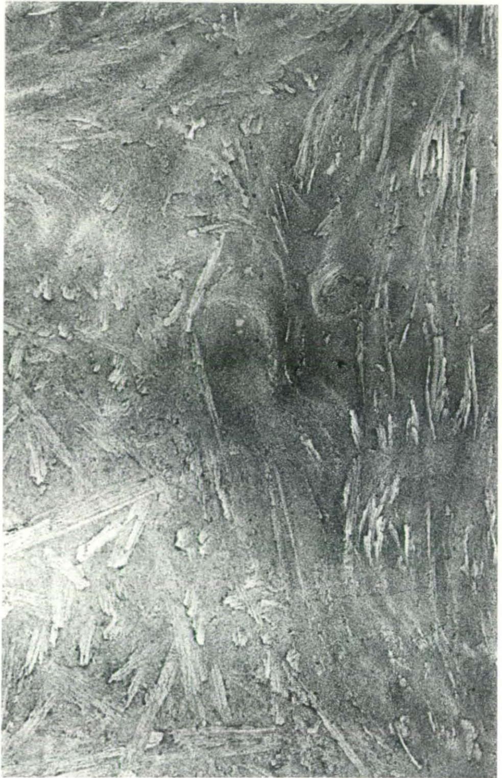
FIGURE 9.21 Weld-line at corner of square plate, moulded with a circular charge shape. Magnification x 6.
