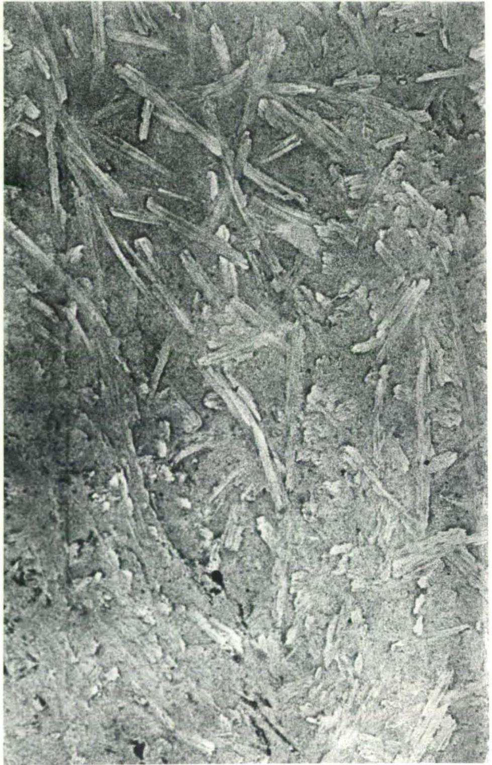
FIGURE 9.22 Fibre distribution for square plate, moulded using calculated charge shape. Magnification x 6.
