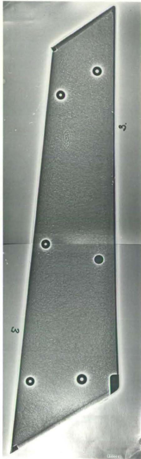
FIGURE 10.6 X-ray photograph of the Teresa grill, moulded using calculated charge shape of 54%
