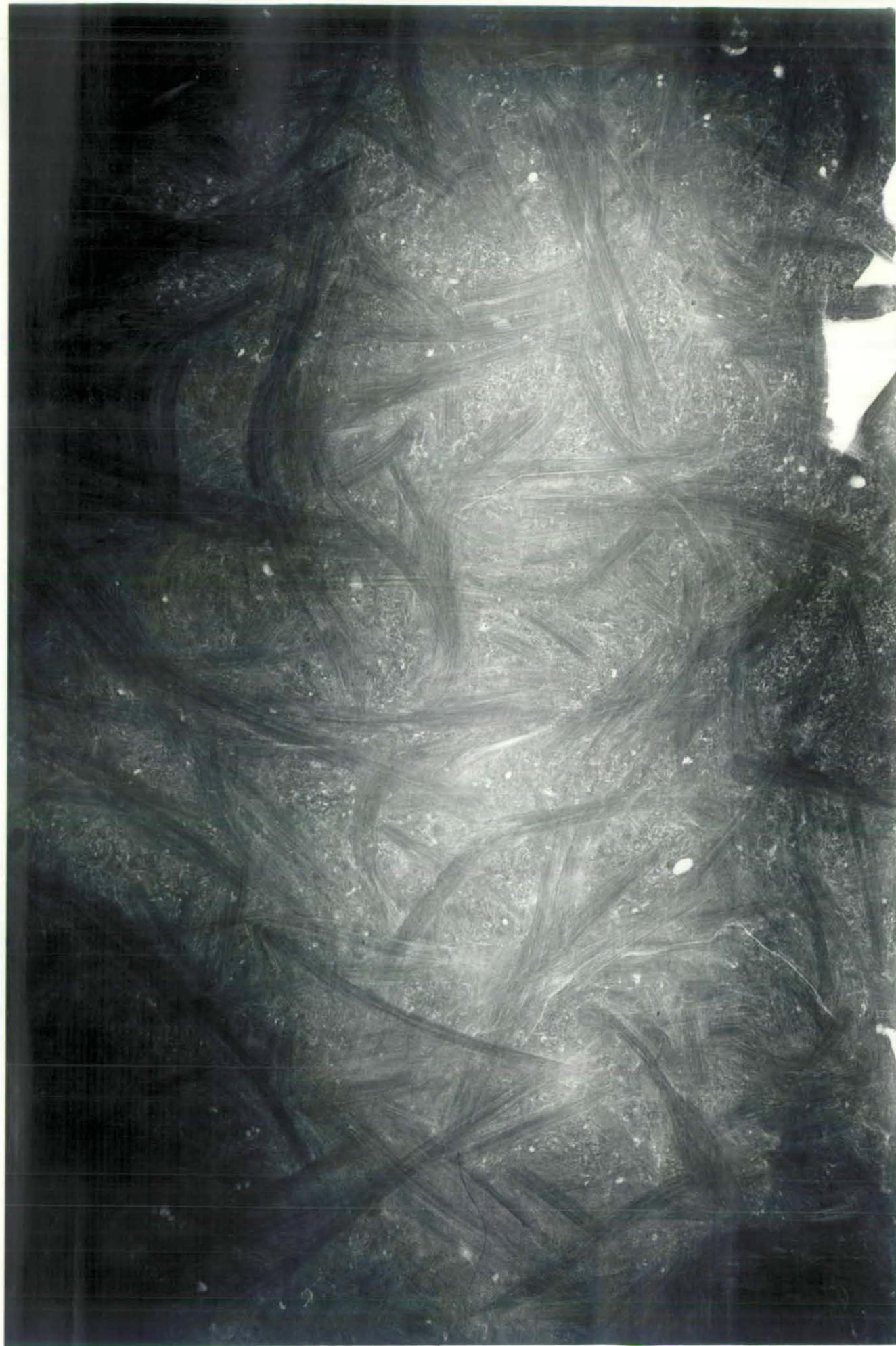
FIGURE 9.4 Fibre distribution in the plane of the SMC sheet (general purpose SMC). Magnification x 6.
