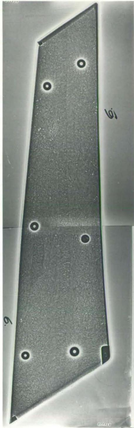
FIGURE 10.5 X-ray photograph of the Teresa grill, moulded with a charge of 107%
