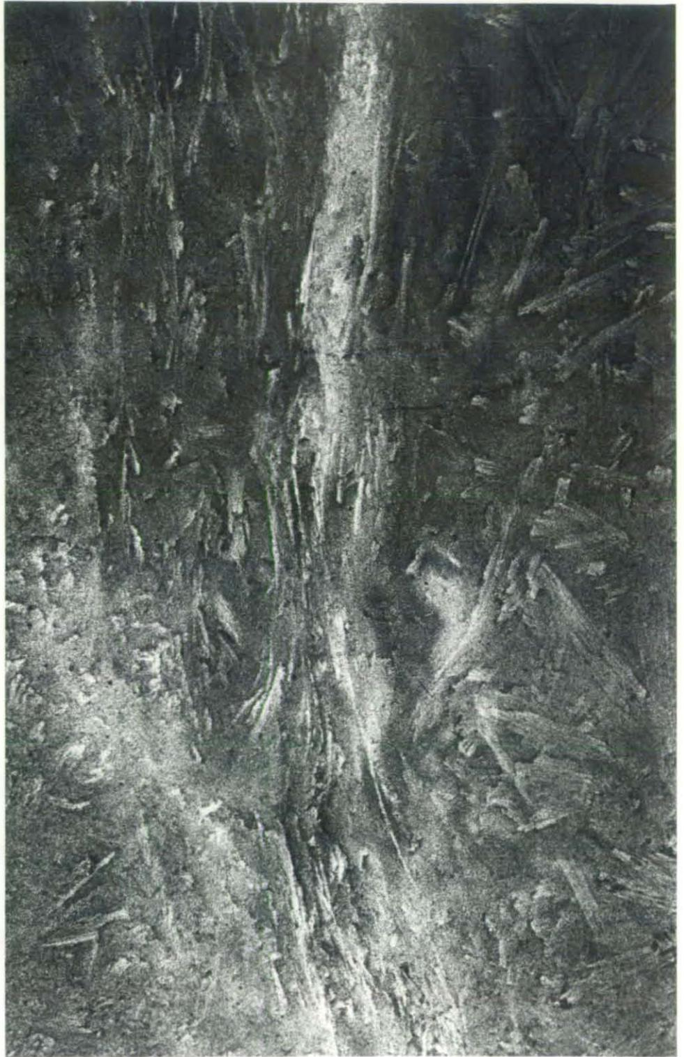
FIGURE 9.20 Weld-line across centre of square plate, moulded with a two rectangle charge shape. Magnification x 6.
