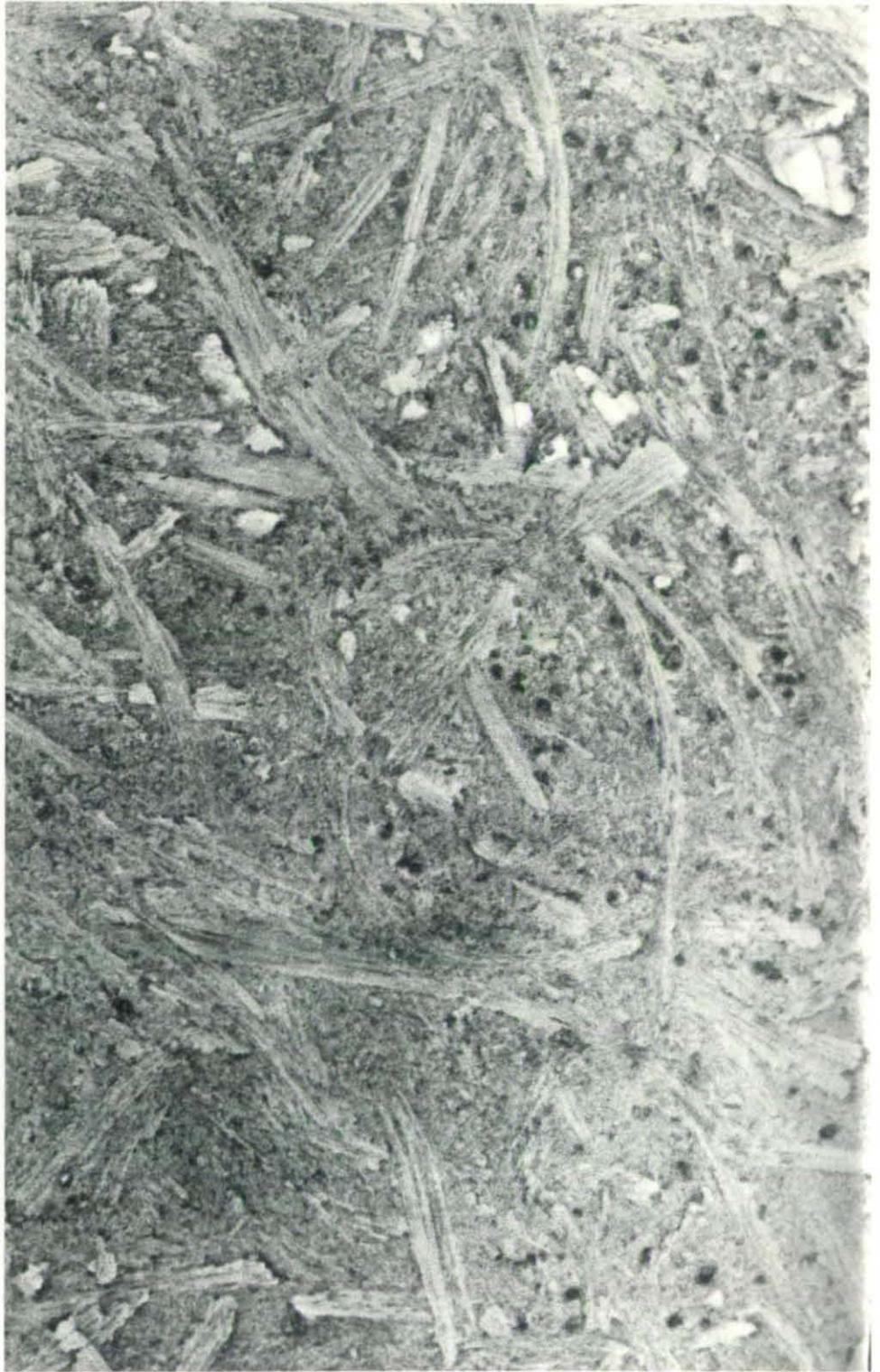
FIGURE 9.6 Fibre distribution in the plane of the SMC sheet (LP-SMC). Magnification x 6.
