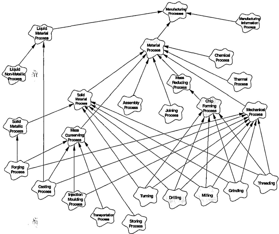
Figure 3.3 – The MOSES Manufacturing Process Representation
