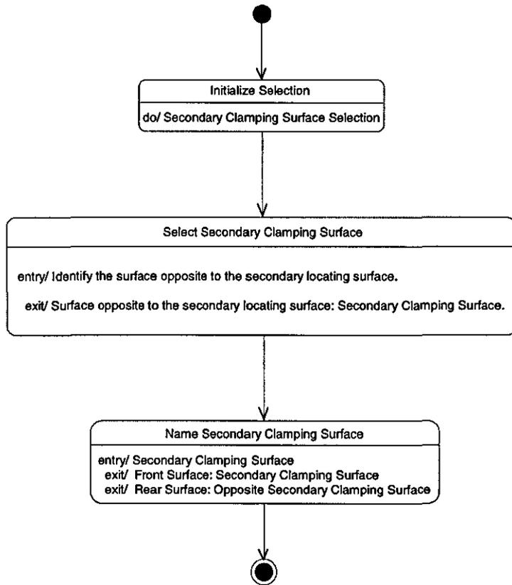
Figure 5.36– Secondary Clamping Surface Selection for 3-2-1 Clamping
