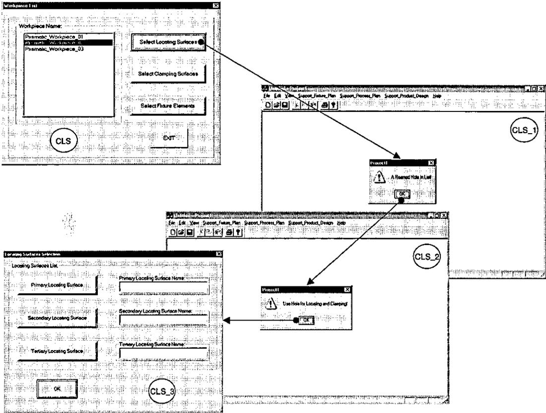
Figure 7.21 – The Dialogs for Selecting Locating Surfaces to Support Fixture Planning Using the Concentric Method
