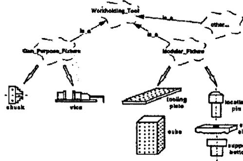
Fig. 8. Populating production resources with particular work-holding tools.
