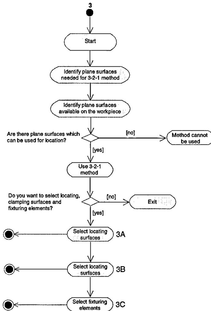
Figure 6.23 – Check the Applicability of 3-2-1 Method in UML Activity Diagram for Support Fixture Planning Application
