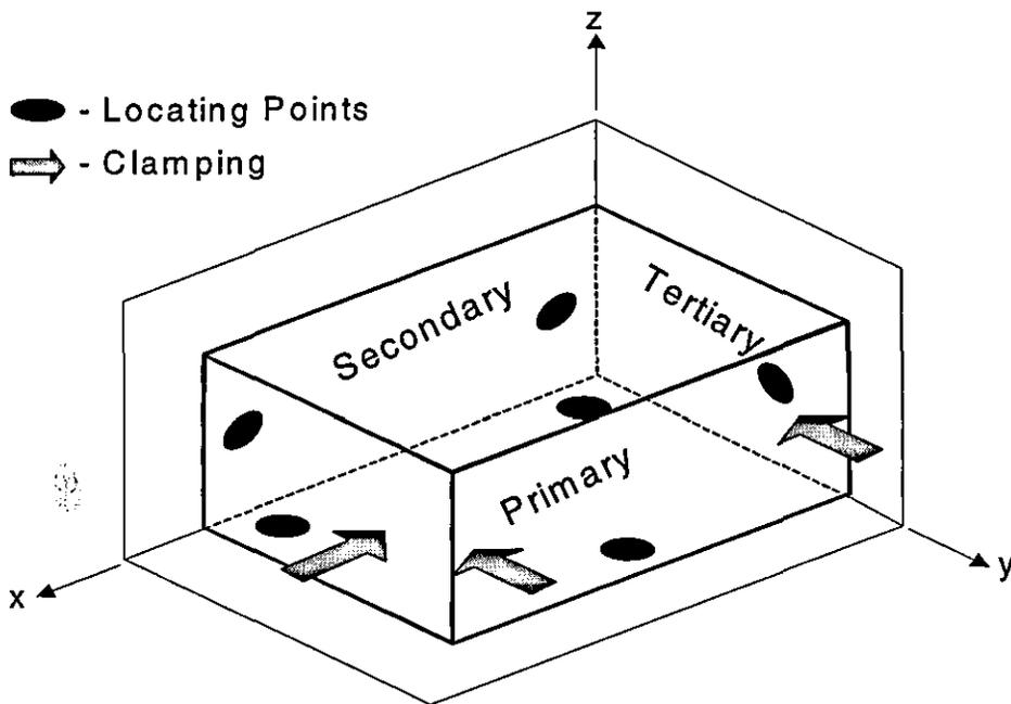
Figure 3.6 – The 3-2-1 Locating Method for a Prismatic Workpiece
