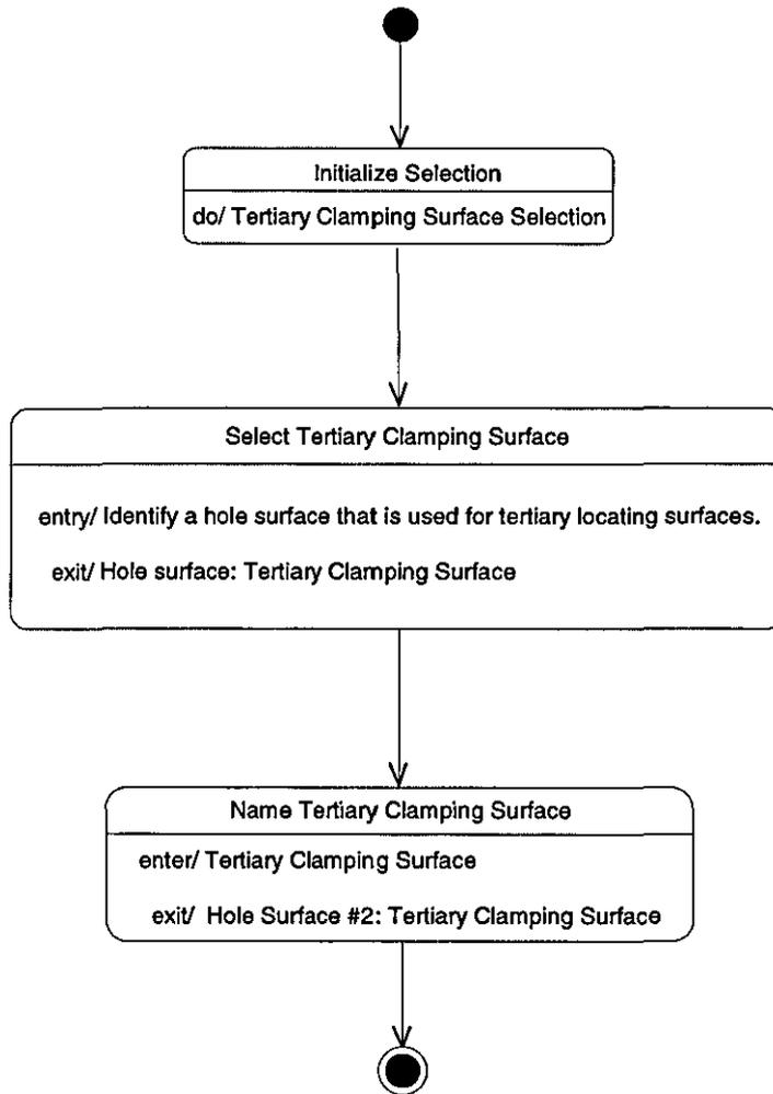
Figure 5.43– Tertiary Clamping Surface Selection for Radial Method
