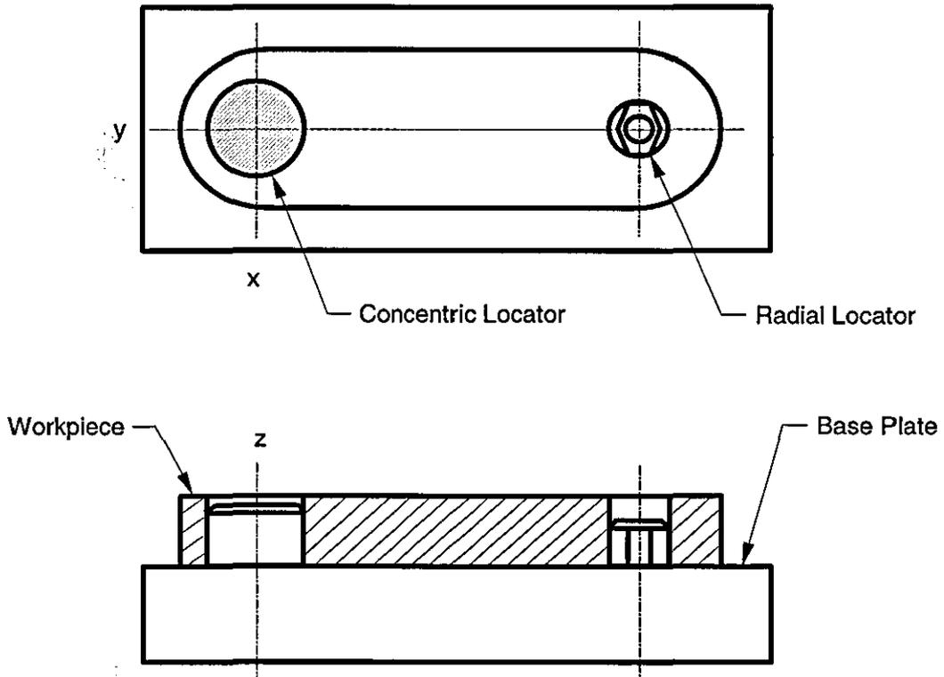
Figure 5.10 – Workpiece Mounted on a Base Plate with Two Locating Pins
