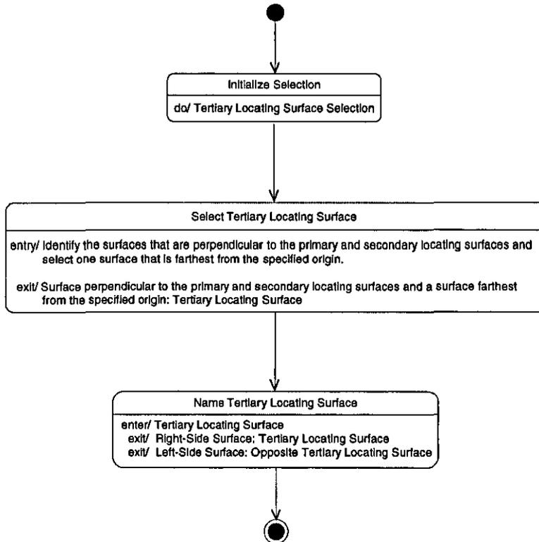
Figure 5.27 – Tertiary Locating Surface Selection for 3-2-1 Locating
