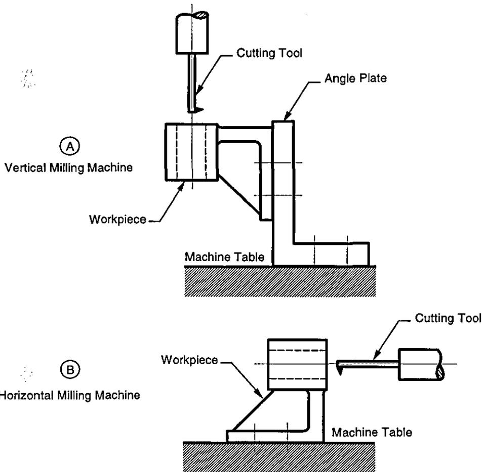
Figure 5.3 – The Vertical and Horizontal Milling Machine Spindle Axes
