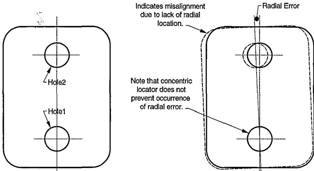
Figure 5.8 – The Radial Locating Method
