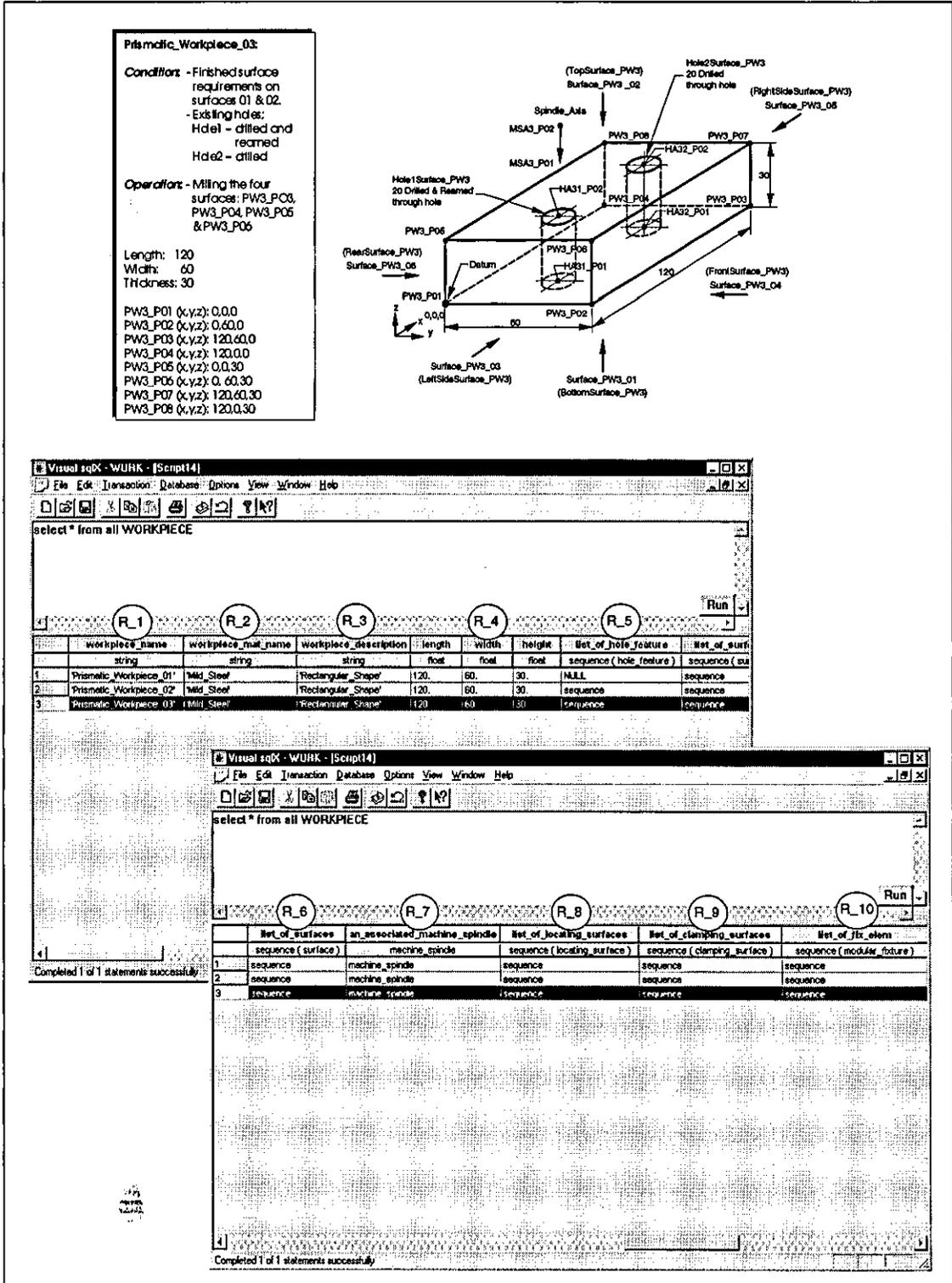
Figure 7.27 – The Prismatic\_Workpiece\_03 Representation Within the Product Model Database
