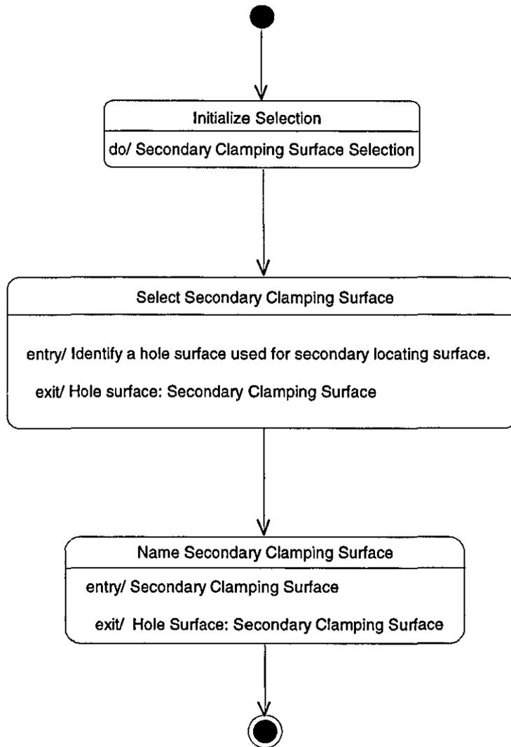
Figure 5.39 – Secondary Clamping Surface Selection for Concentric Method
