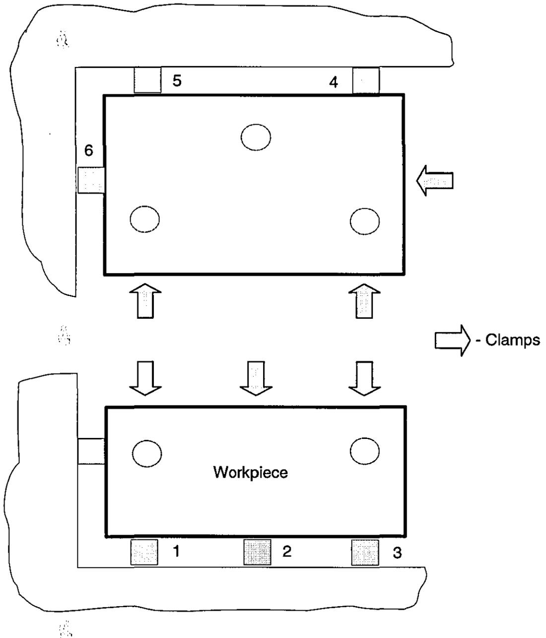
Figure 5.13 – Clamps are Placed on the Surfaces Opposite the Locating Surface
