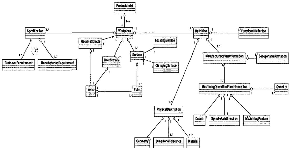
Figure 5.5.1 – The General Structure of the Product Model in UML Class Diagram [Extended from Borja, 1997]
