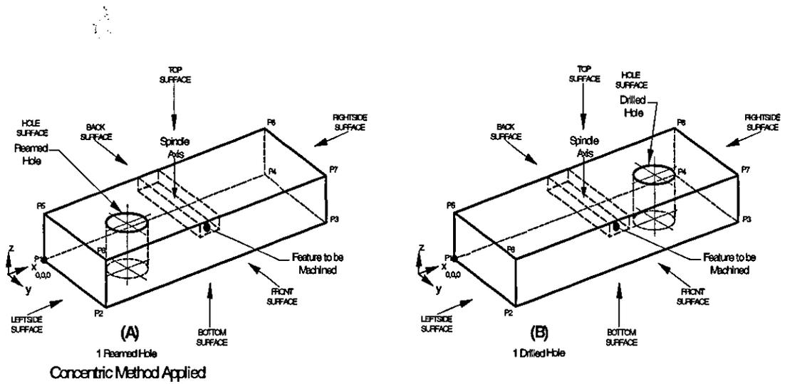
Figure 6.6 – Sample Variations of a Workpiece for the Applicability of Concentric Method
