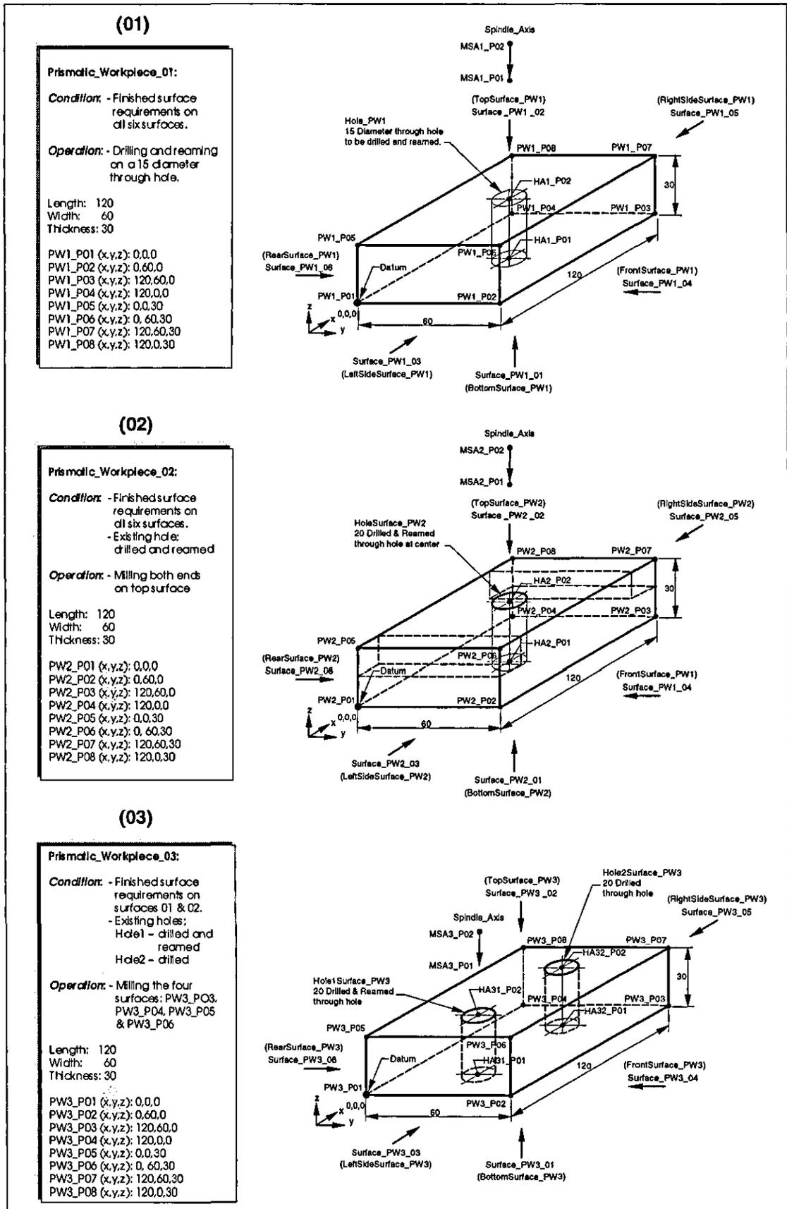
Figure 7.1 – The Prismatic Workpieces
