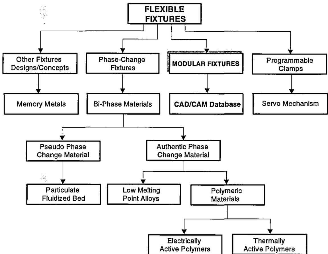
Figure 3.7 – An Overview of Flexible Fixturing Methodologies
