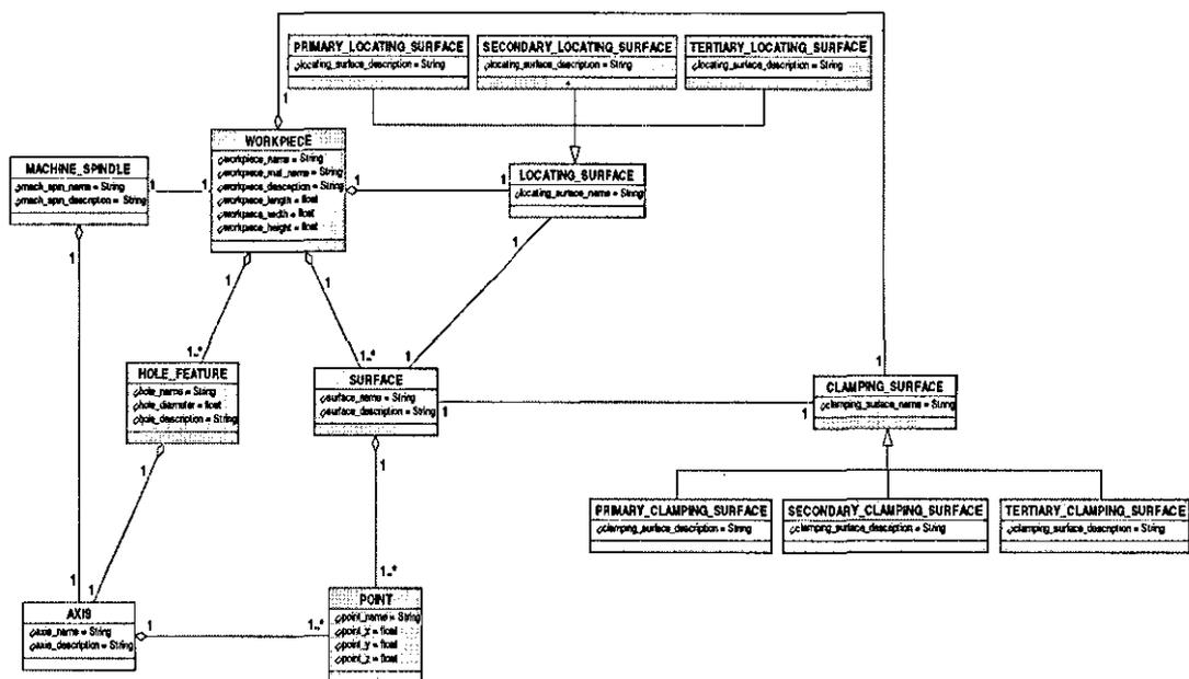
Figure 5.52 – The Structure of the Product Data Model in UML Class Diagram
