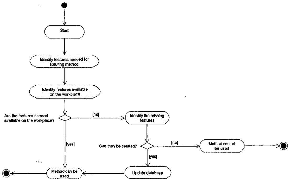
Figure 6.28 – The General Activity Diagram for Checking the Applicability of the Fixturing Methods
