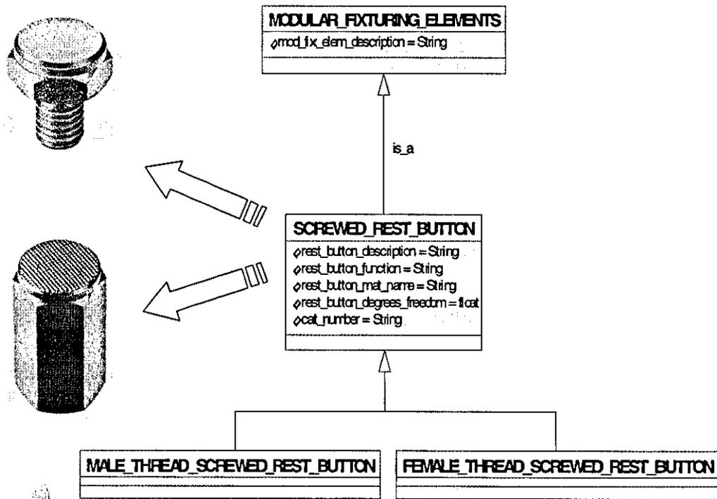
Figure 5.47 – The Representation of Screwed Rest Buttons
