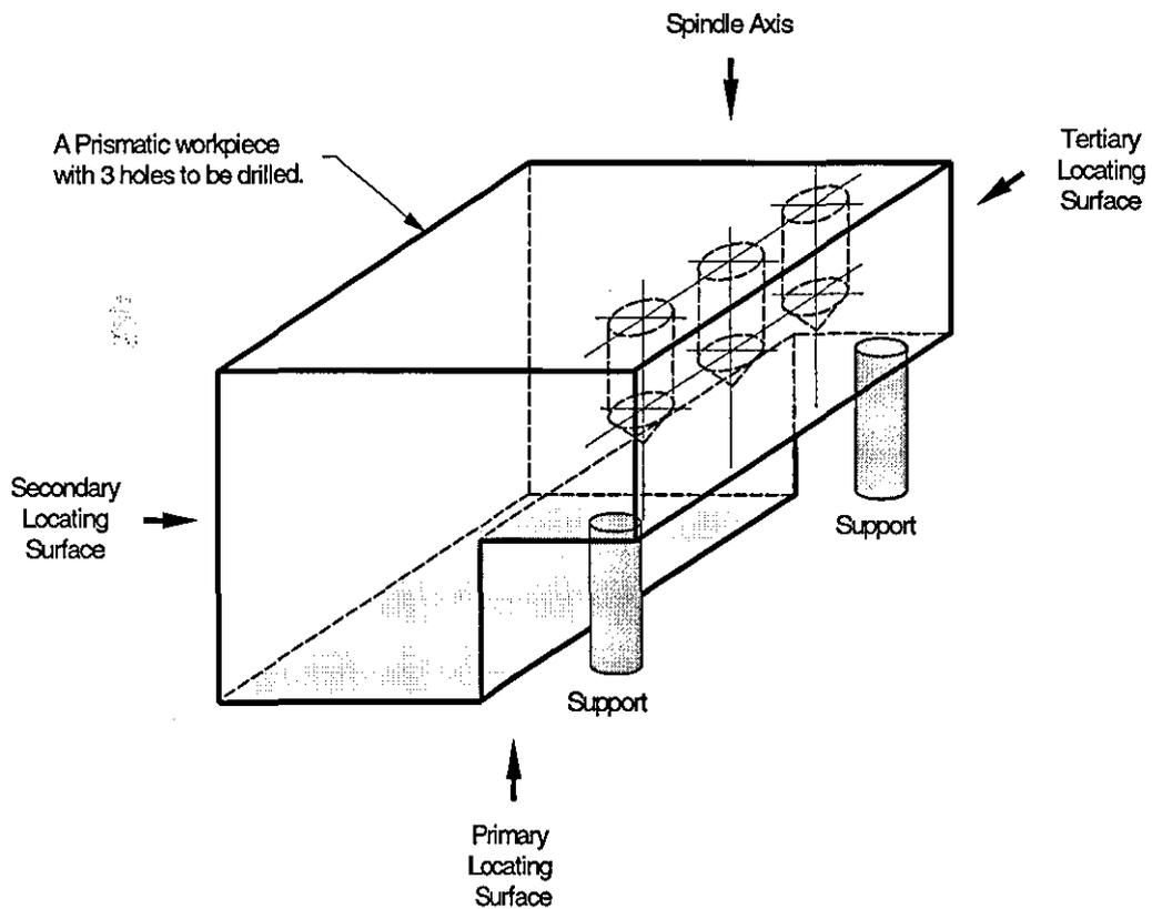
Figure 5.6 – A Prismatic Workpiece with Three Blind Holes Using 3-2-1 Locating Method
