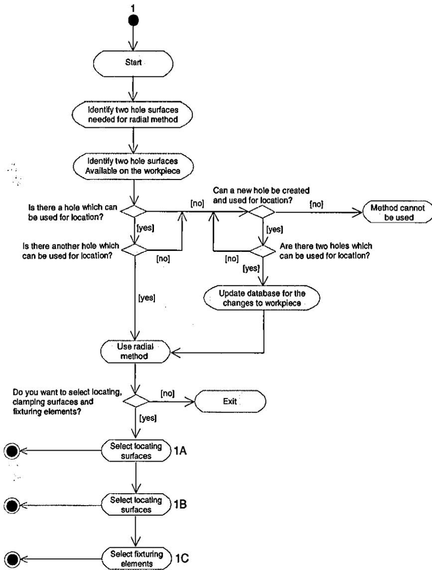
Figure 6.16 – Check the Applicability of Radial Method in UML Activity Diagram for Support Fixture Planning Application
