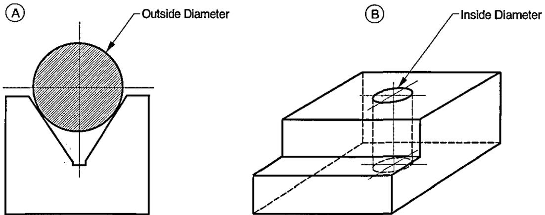
Figure 5.7 – The Concentric Locating Method
