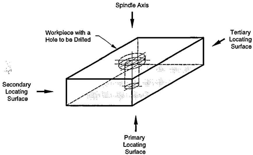
Figure 5.5A – A Prismatic Workpiece Using the 3-2-1 Locating Method
