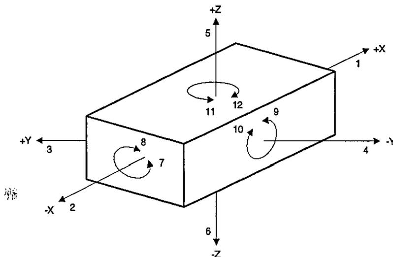
Figure 3.5 – The Degrees of Freedom for a Prismatic Workpiece
