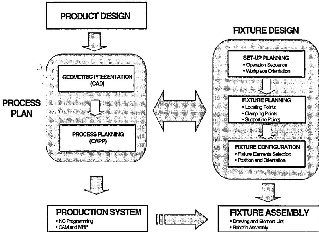
Figure 2.1 - Fixture Design in Manufacturing Systems
