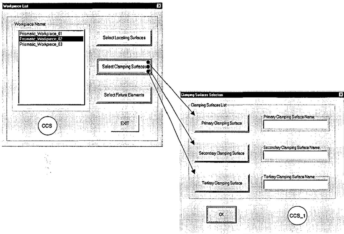
Figure 7.23 – The Dialogs for Selecting Clamping Surfaces to Support Fixture Planning Using the Concentric Method
