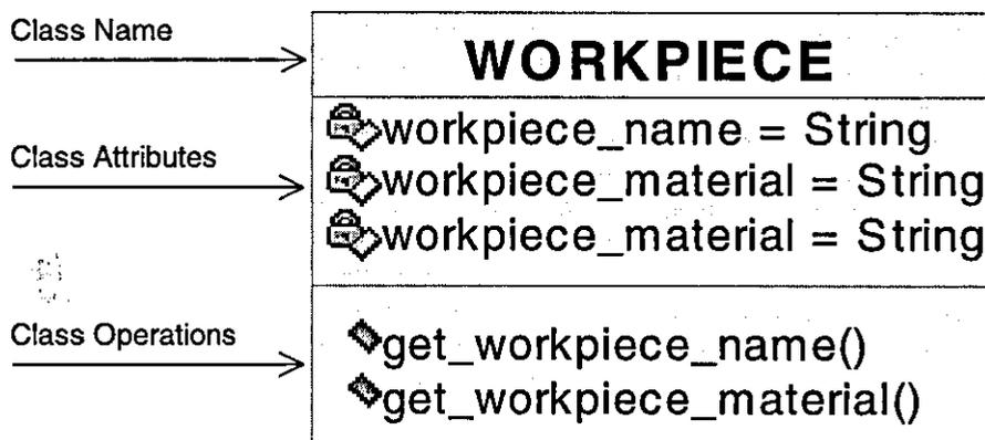
Figure A-B1 – Class Diagram Representation
