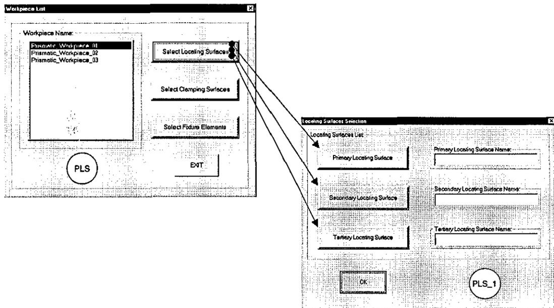
Figure 7.15 – The Dialogs for Selecting Locating Surfaces to Support Fixture Planning Using the 3-2-1 Method
