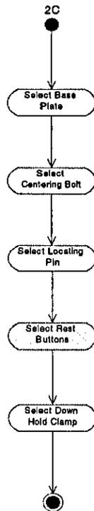
Figure 6.21 – Select Modular Fixturing Elements for Concentric Method
