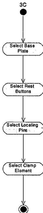
Figure 6.26 – Select Modular Fixturing Elements for 3-2-1 Method
