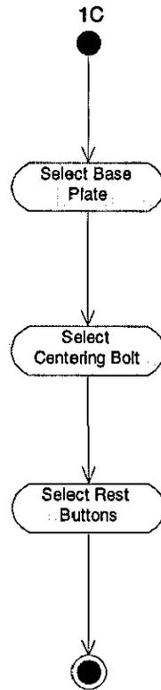
Figure 6.19 – Select Modular Fixturing Elements for Radial Method
