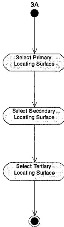
Figure 6.24 – Select Locating Surfaces for 3-2-1 Method
