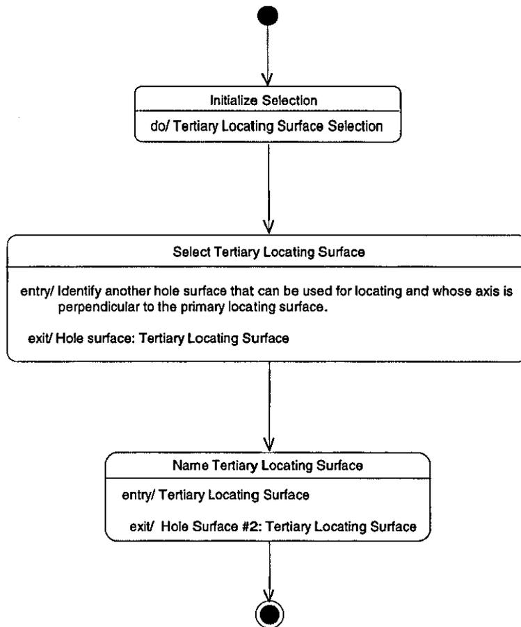
Figure 5-33 – Tertiary Locating Surface Selection for Radial Method
