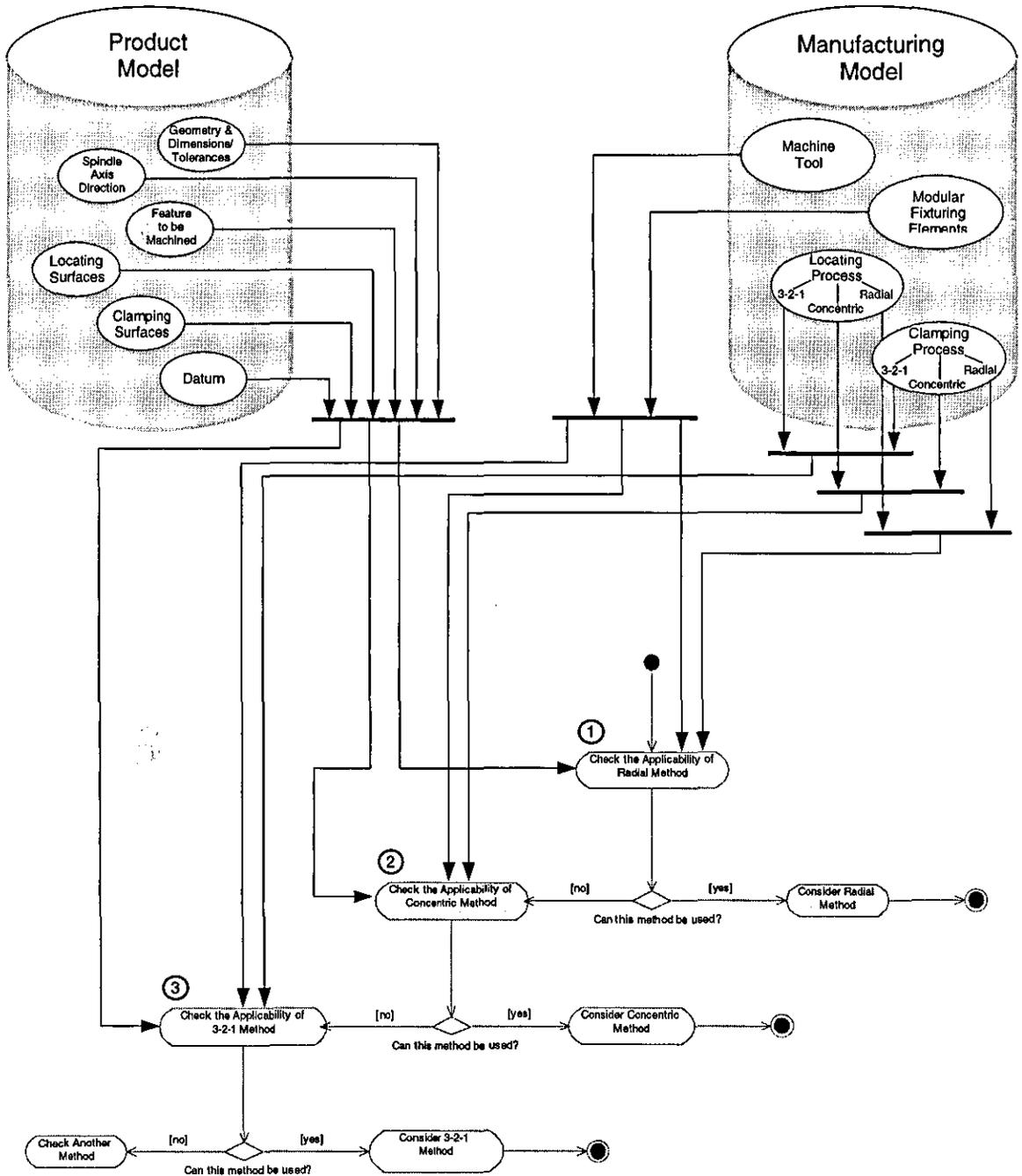
Figure 6.15 – Support Fixture Planning Activities in UML Activity Diagram
