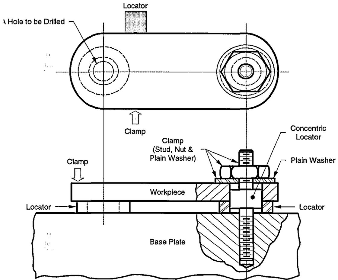
Figure 5.15 – The Clamping for Concentric Method
