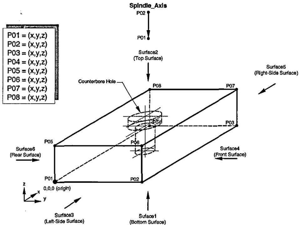
Figure 5.24 – Example of a Prismatic Workpiece as Depicted in the Product Model
