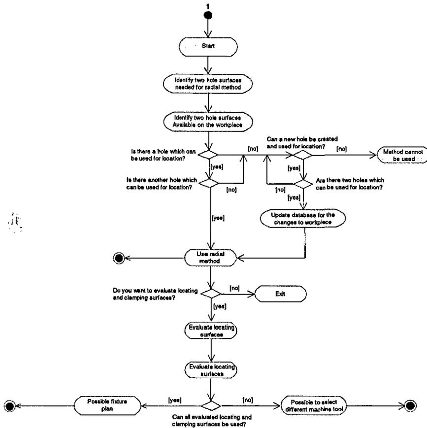
Figure 6.11 – Check the Applicability of Radial Method in UML Activity Diagram for Support Process Planning Application
