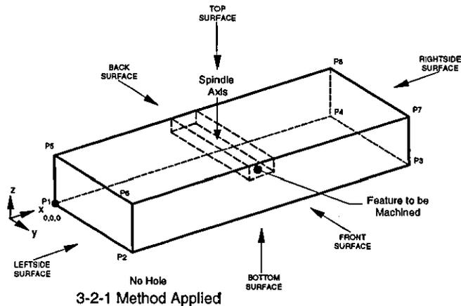
Figure 6.8 – Workpiece for the Applicability of 3-2-1 Method
