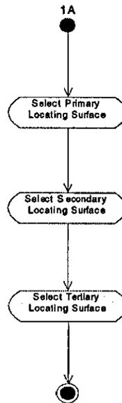
Figure 6.17 – Select Locating Surfaces for Radial Method
