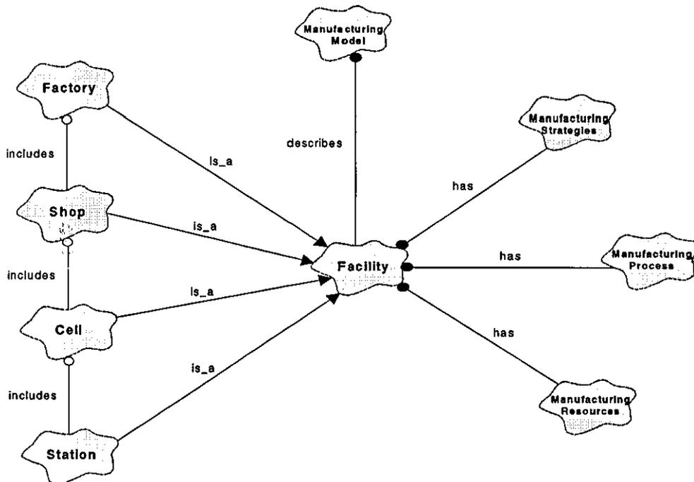
Figure 3.2 – The Framework of the Manufacturing Model
