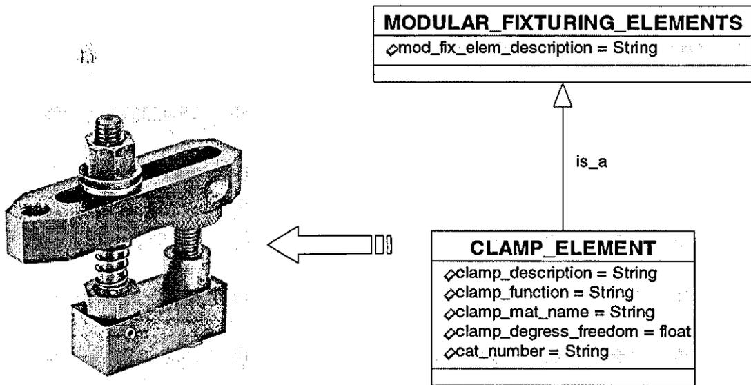
Figure 5.48 – The Representation of Clamp Elements
