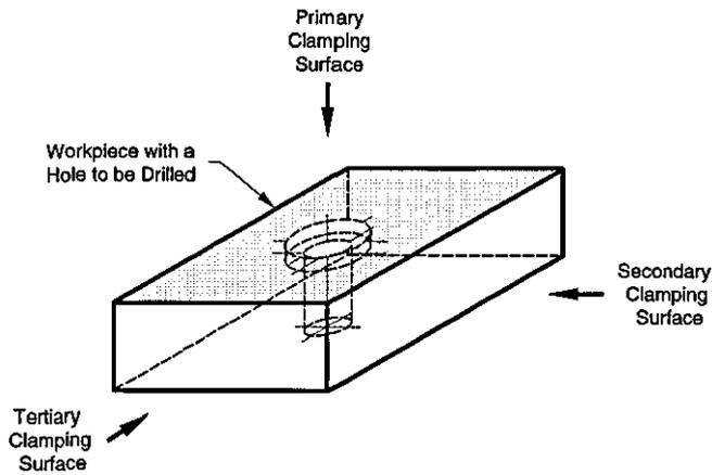
Figure 5.14 – The Clamping for 3-2-1 Method
