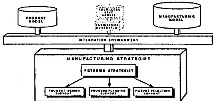
Fig. 2. Fixturing within the MOSES concept.
