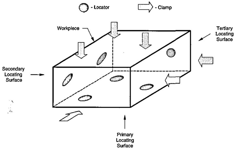
Figure 5.9 – The Clamps are Placed Directly Opposite to the Locators
