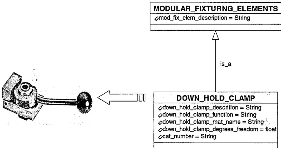
Figure 5.49 – The Representation of Down Hold Clamps
