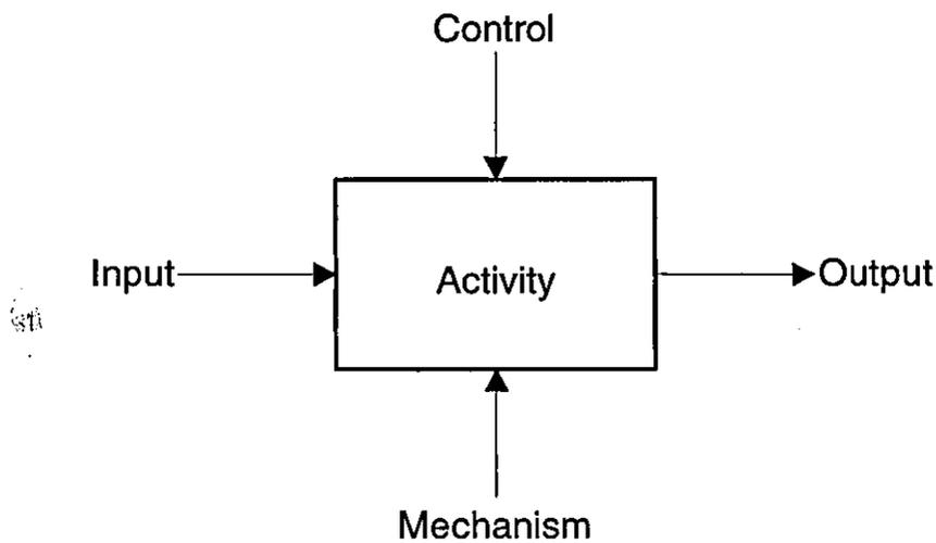
Figure A-A.2 – IDEF0 Function Box and Interface Arrows
