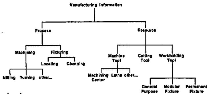
Fig. 5. Manufacturing data structure.
