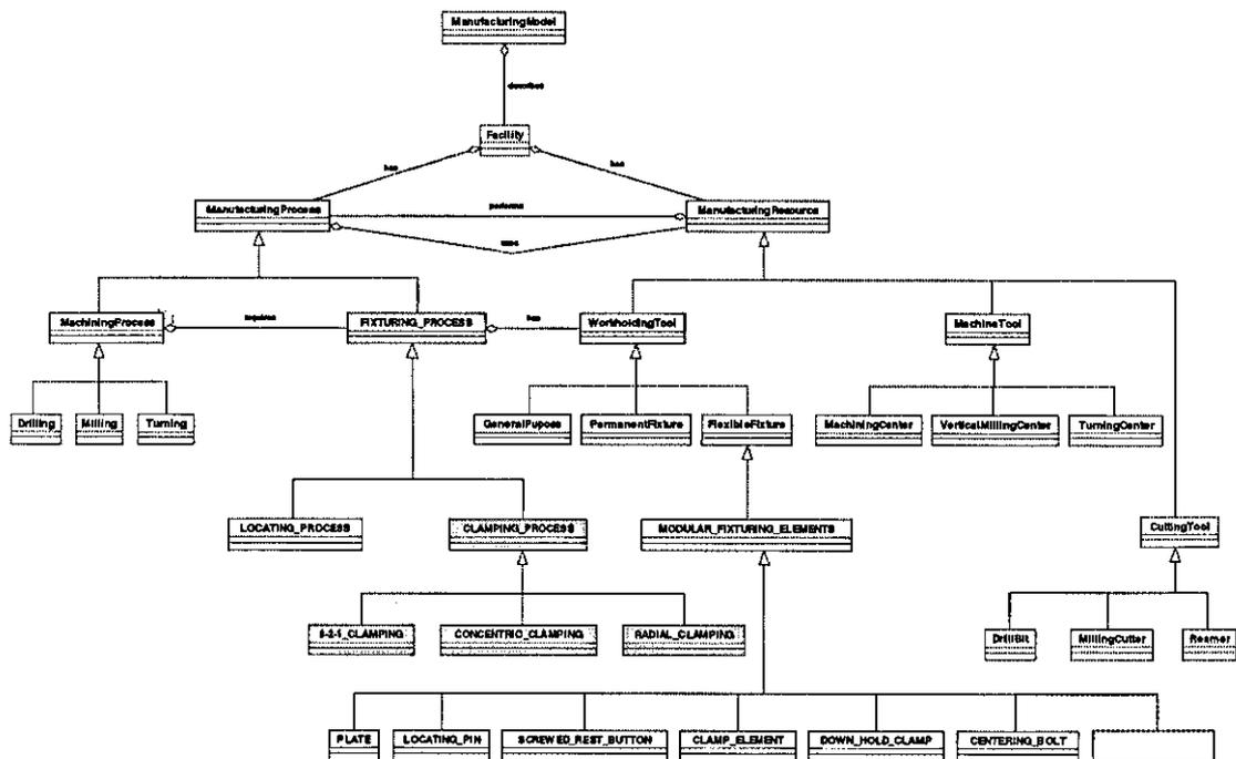
Figure 5.28 – Clamping Process Data Structure in UML Class Diagram
