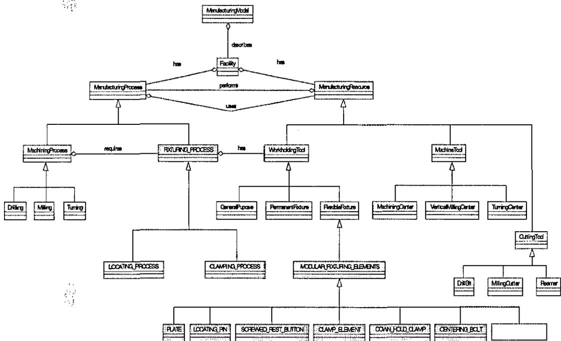
Figure 5.22 – The MOSES Manufacturing Model Structure in UML Class Diagram with the Fixturing Information
