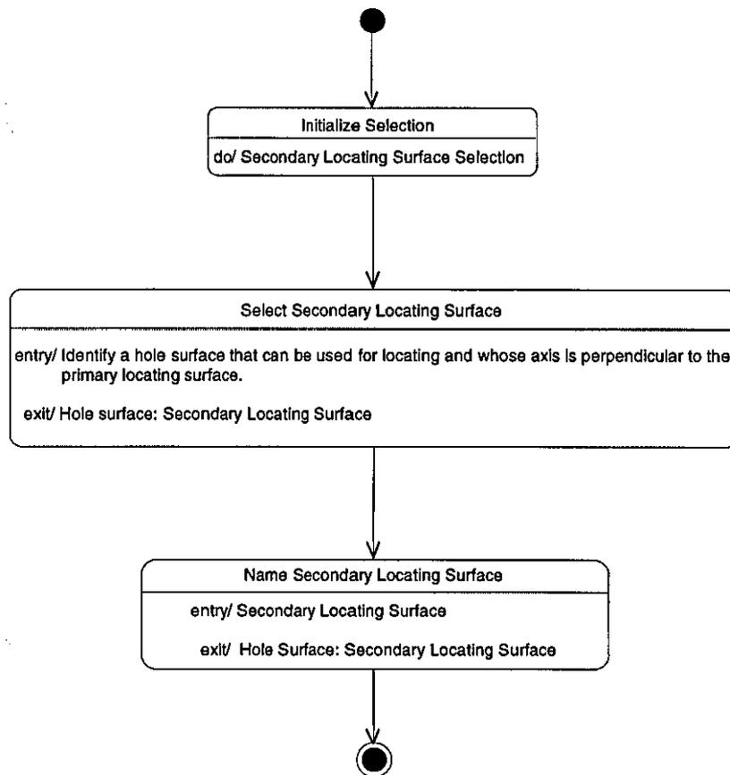
Figure 5.29 – Secondary Locating Surface Selection for Concentric Method
