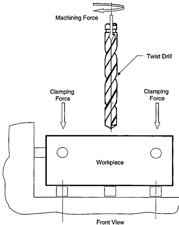
Figure 5.12 – Cutting Forces in a Drilling Operation
