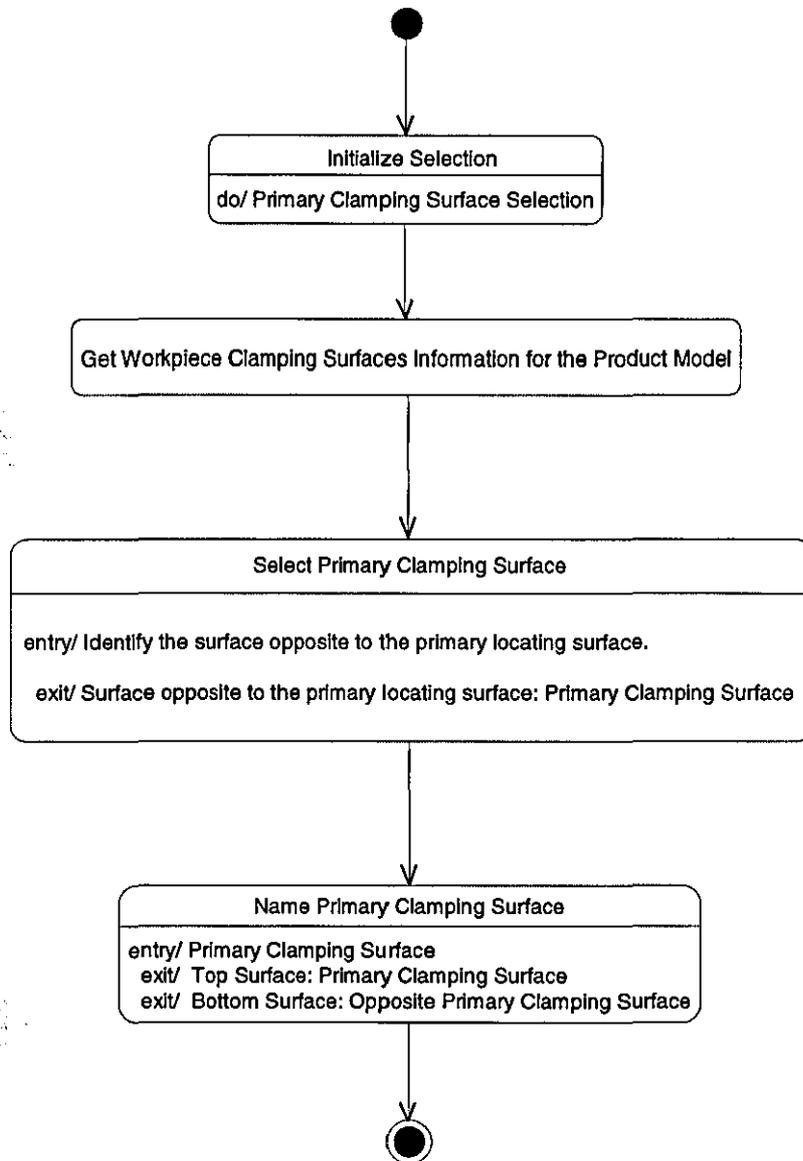
Figure 5.41 – Primary Clamping Surface Selection for Radial Method in UML Activity Diagram
