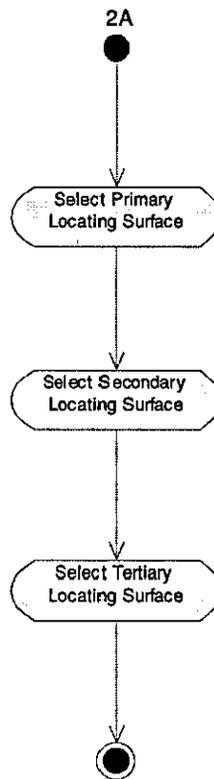
Figure 6.19 – Select Locating Surfaces for Concentric Method
