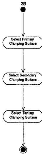
Figure 6.25 – Select Clamping Surfaces for 3-2-1 Method
