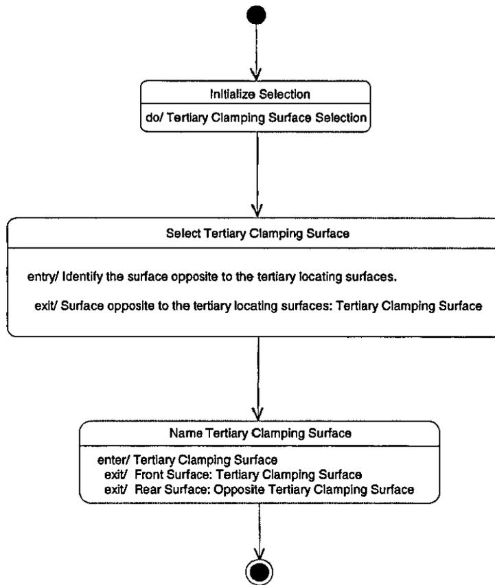
Figure 5.40 – Tertiary Clamping Surface Selection for Concentric Method
