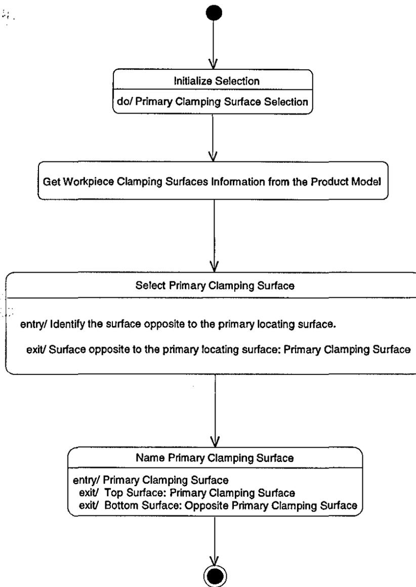
Figure 5.38 – Primary Clamping Surface Selection for Concentric Method in UML Activity Diagram
