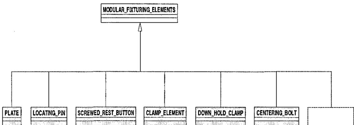
(a) Figure 5.44 – Fixturing Elements Data Structure in UML Class Diagram
