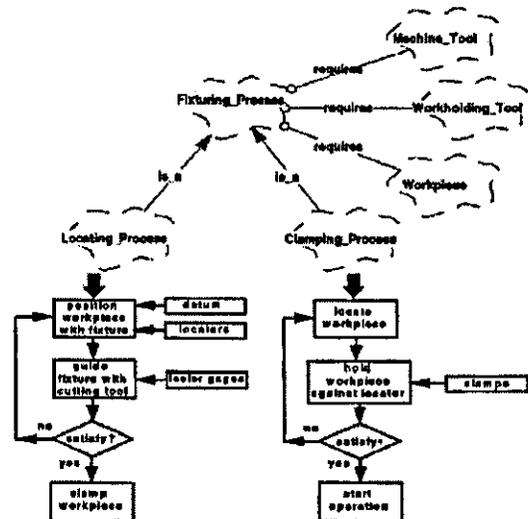
Fig. 9. Fixturing processes within the data structure.
