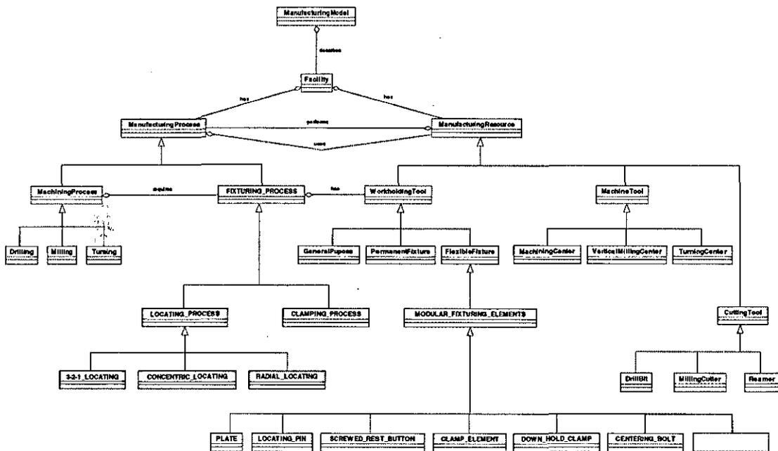
Figure 5.23 – Locating Process Data Structure in UML Class Diagram
