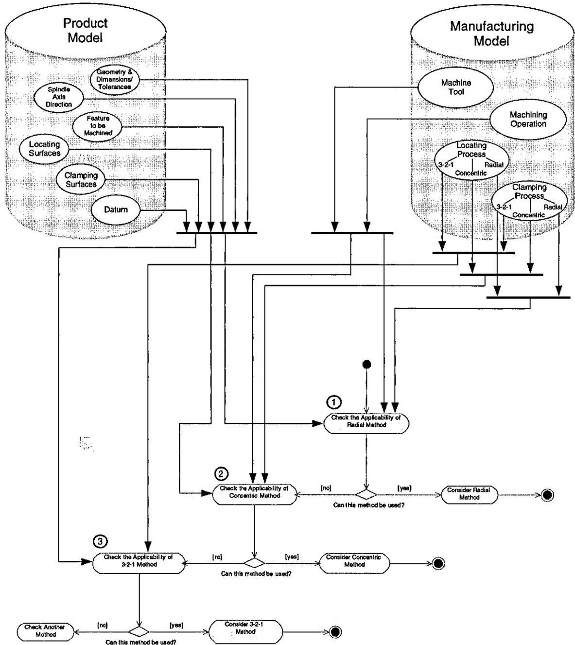
Figure 6.10 – Support Process Planning Activities in UML Activity Diagram
