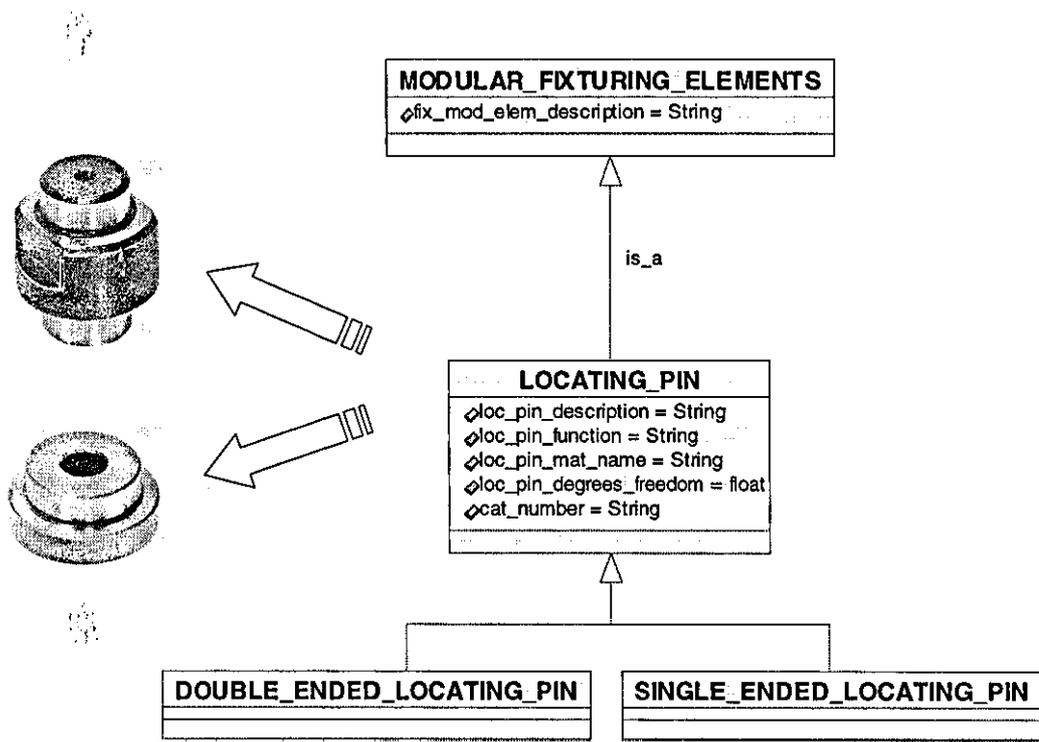
Figure 5.46 – The Representation of Locating Pins
