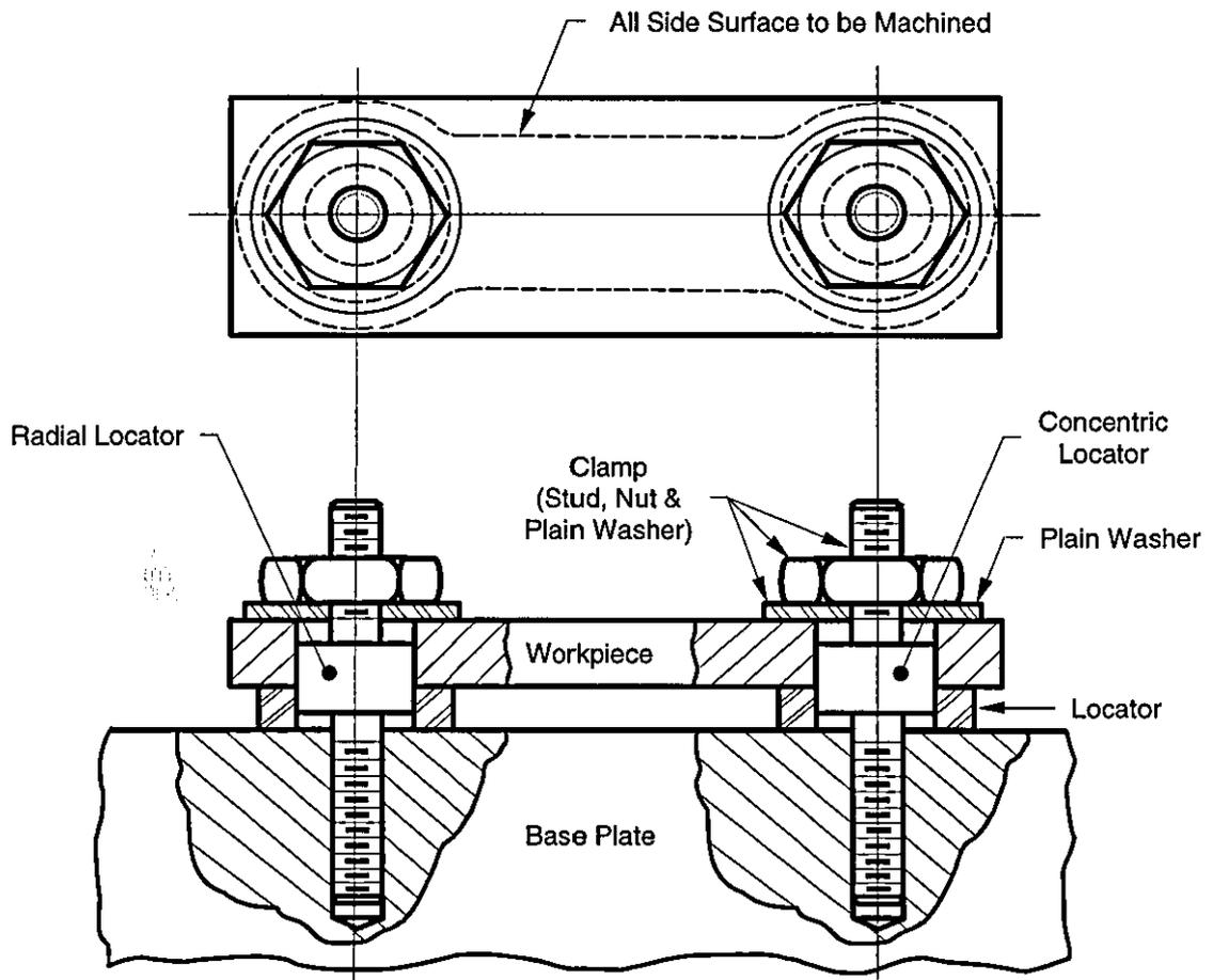
Figure 5.16 – The Clamping for Radial Method
