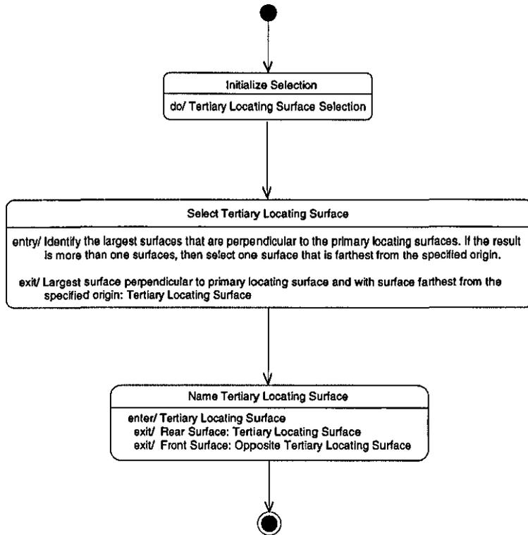
Figure 5.30 – Tertiary Locating Surface Selection for Concentric Method
