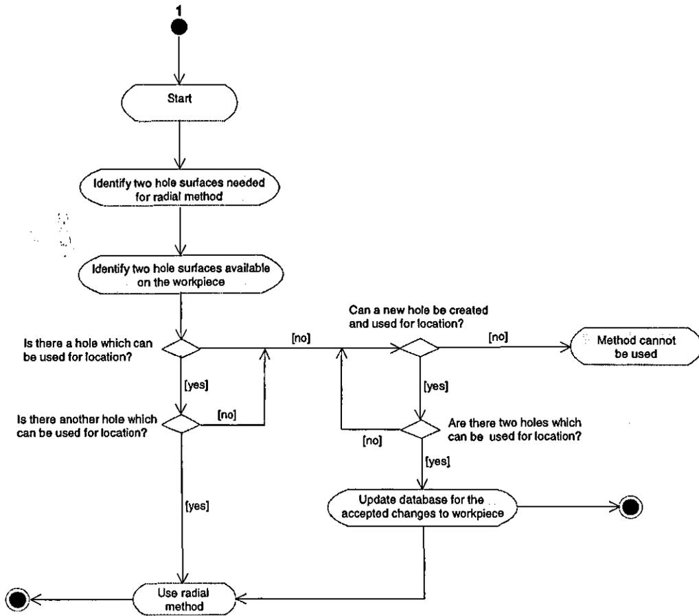
Figure 6.3 – Check the Applicability of Radial Method in UML Activity Diagram for Support Product Design Application
