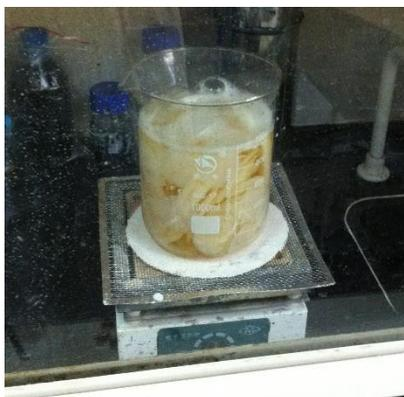
**Figure A.2.** BC membranes in a boiled NaOH solution.
