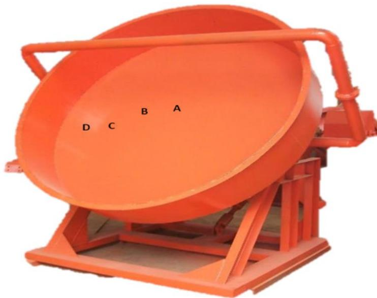
*Figure 2-33 An example pelletizing disc (letters A, B, C and D represent locations of where nozzles are located on this specific pelletizing disc). [101]*
