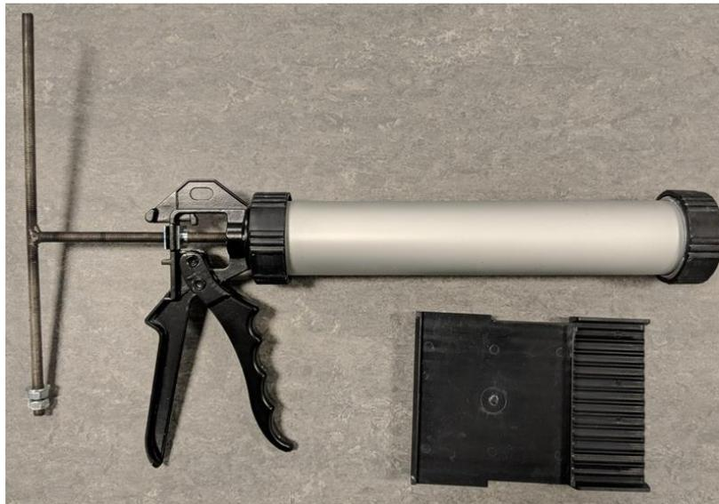
*Figure 5-10 Image of sausage rolling table (left) and sausage gun (right)*
