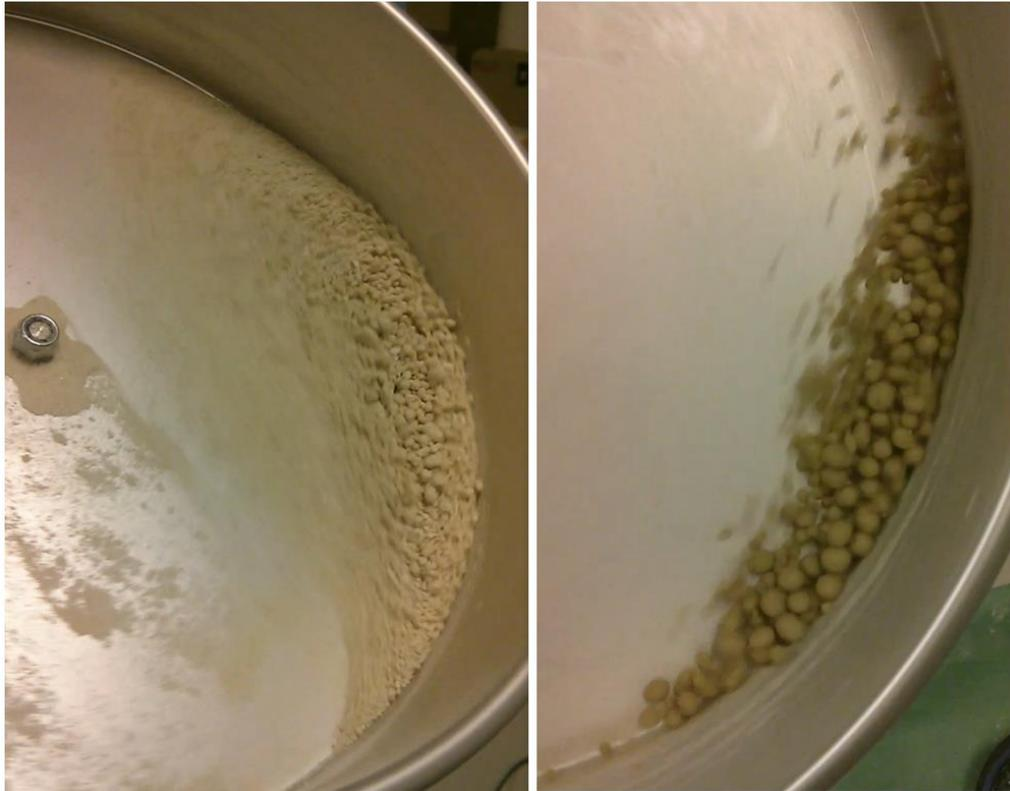
*Figure 5-7 Image of material in pelletizing disc showing the anticlockwise agglomerating motion of particles into beads*
