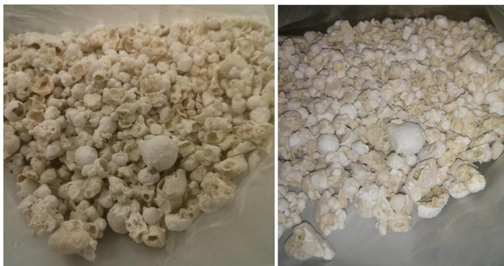
*Figure 5-9 Image of beads created with pelletizing disc after an oven bake at 150°C*
