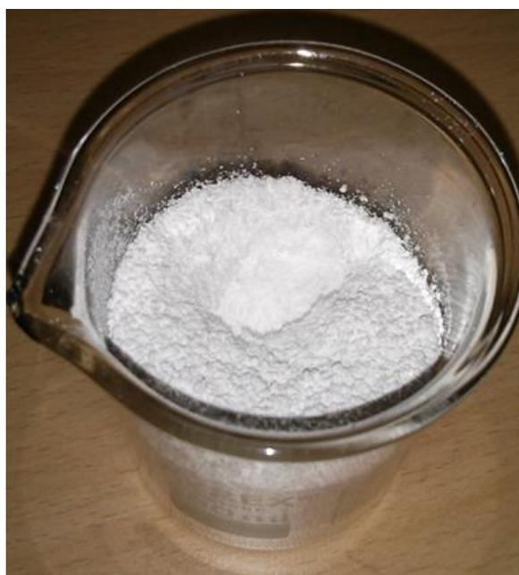
*Figure 5-1 Image of  $\text{MgSO}_4 \cdot 7\text{H}_2\text{O}$  in a beaker after a heating to  $150^\circ\text{C}$ , with a 3h isotherm, showing the solid structure which was formed*
