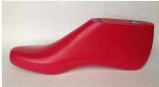
Figure 2-13 – A solid shoe last manufactured from HDPE
