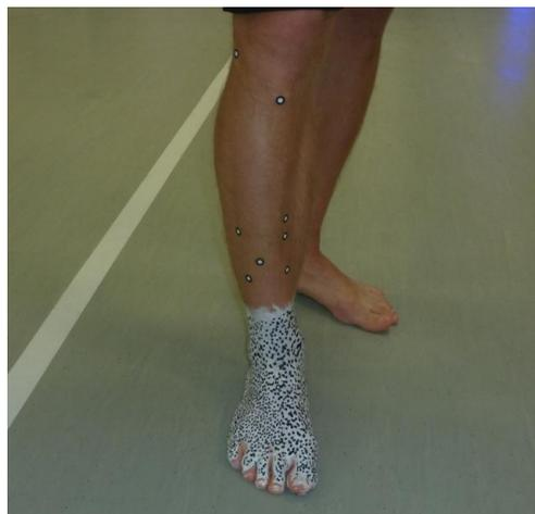
Figure 6-18 - Kinematic adapter reference cluster on anterior tibia surface
