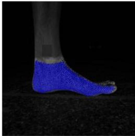
Figure 4-14 - ARAMIS surface measurement results, denoted by blue region, for painted pattern applied to surface of foot.
