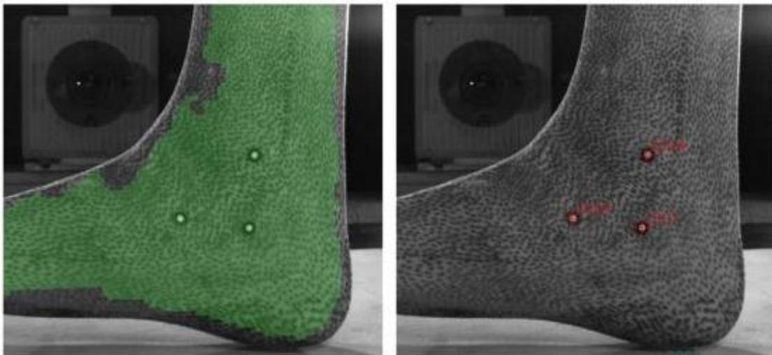
Figure 6-17 – Kinematic markers on the foot, ARAMIS surface measurement (left), PONTOS point measurement (right)
