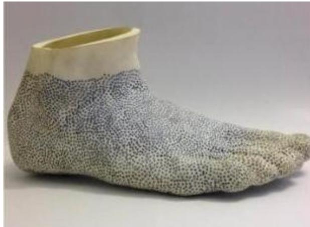
Figure 4-18 - Additive manufactured static foot shape used for repeatability measurements
