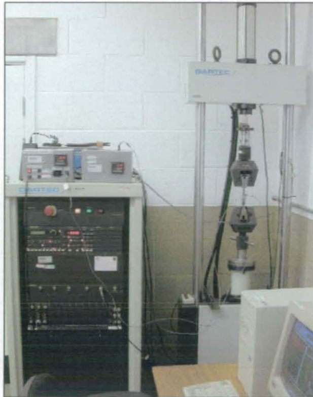
Fig. 8.6 Set-up used for monitoring hysteretic heating.
