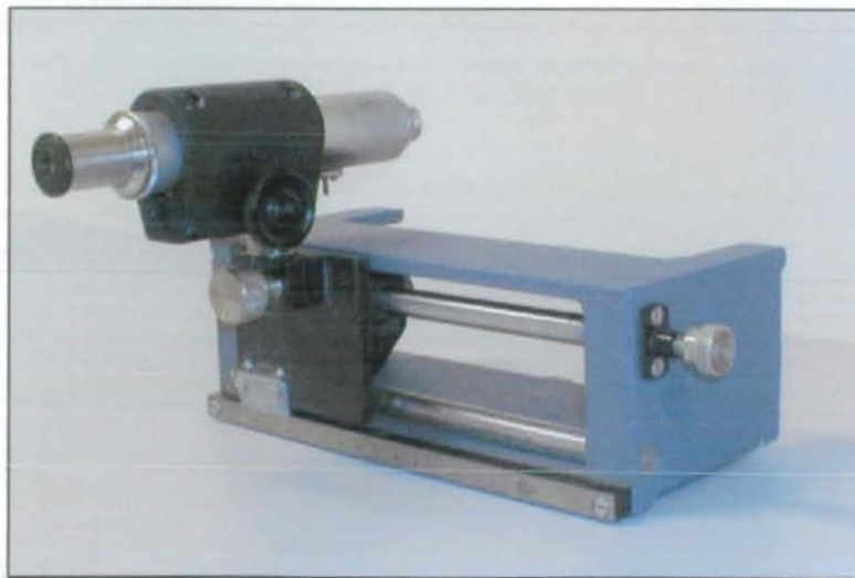
Fig. 8.4 Traveling optical microscope used in this study
