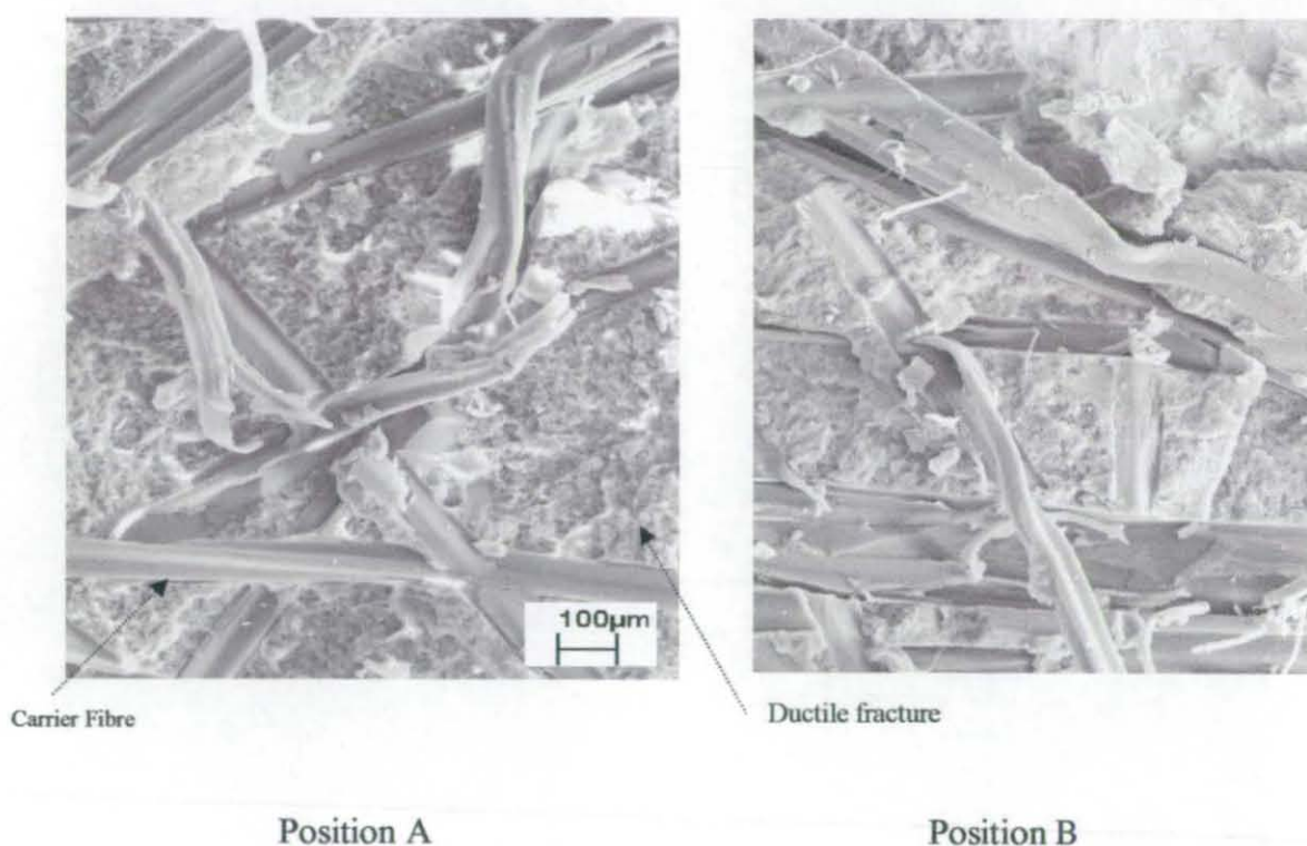
Fig. (9.56) Image of failed test specimen of mild steel joints tested at 90°C
