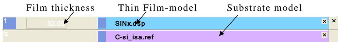
Figure 49 Model of a silicon nitride film deposited on a c-Si wafer
