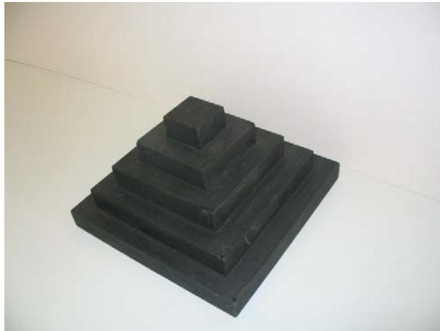
Figure 5-1: Pyramid calibration piece
