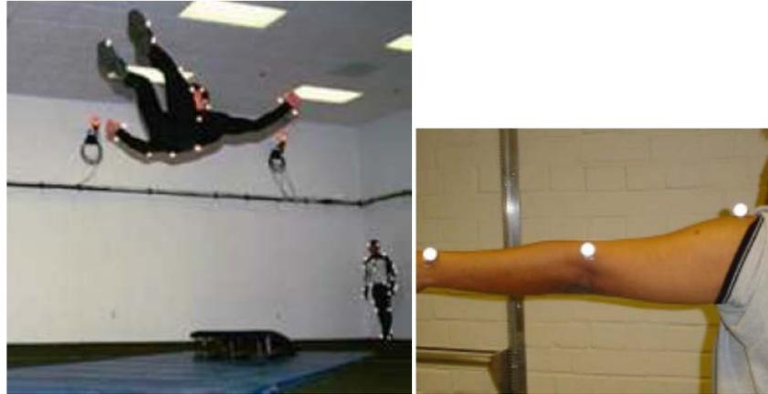
Figure 4-2: Reflective markers used in vision systems (Zhou, *et al.*, 2008)
