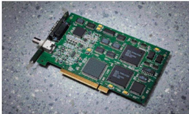
Figure A-9 : The DT3155, monochrome frame grabber for the PCI Bus
