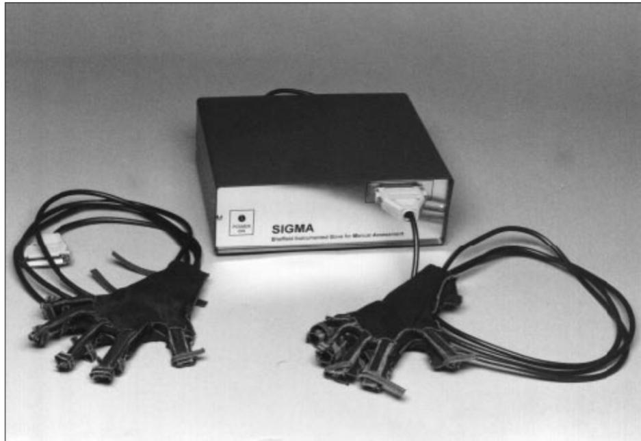
Figure 2-6 : The completed goniometric gloves, small and medium size (William, *et al.*, 2000)
