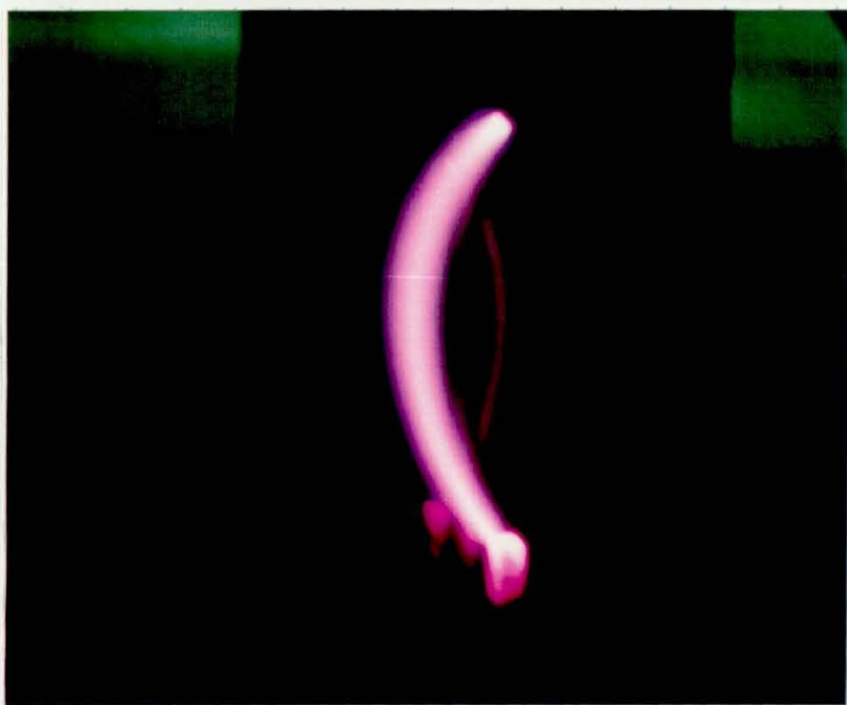
Fig. 5.20 Electric discharge in He at 500 mb parallel to a conductor carrying a current of 100 A (second image is due to reflections).
