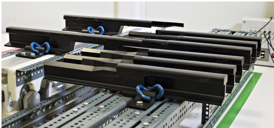
Figure 4.5 Double chamfer interlocking rail end mock-ups as fitted to laboratory demonstrator.
