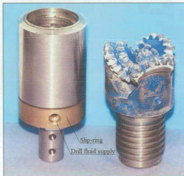
Figure 4.2: Drill hub (left) and Tricone bit (right)
