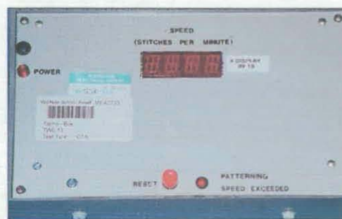
Figure 4.8: Digital display of the actual shaft speed
