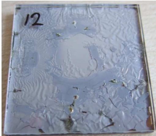
Figure 4-16. PMMA bonded to aluminium
