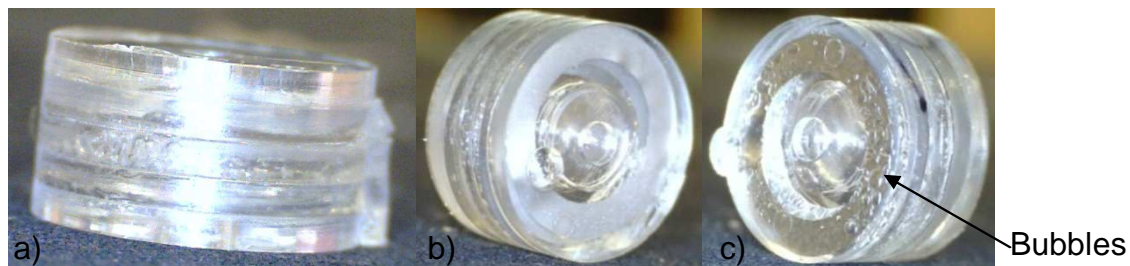
Figure 7-24. Induction bonded stack of polymer discs, a) side, b) top and c) bottom – Stack 3 (3 x 2s heating, 7s cooling)
