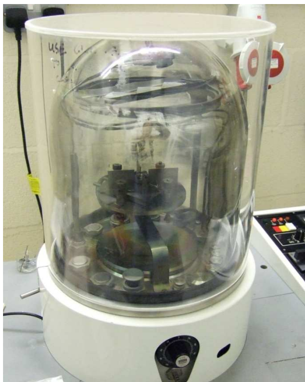
Figure 3-6. Evaporation chamber with jar and protecting cylinder
