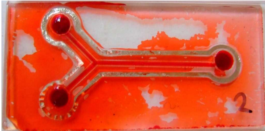
Figure 7-19. Leaking microfluidic device – Sample No. 2 (4 x 6s heating, 5s cooling)
