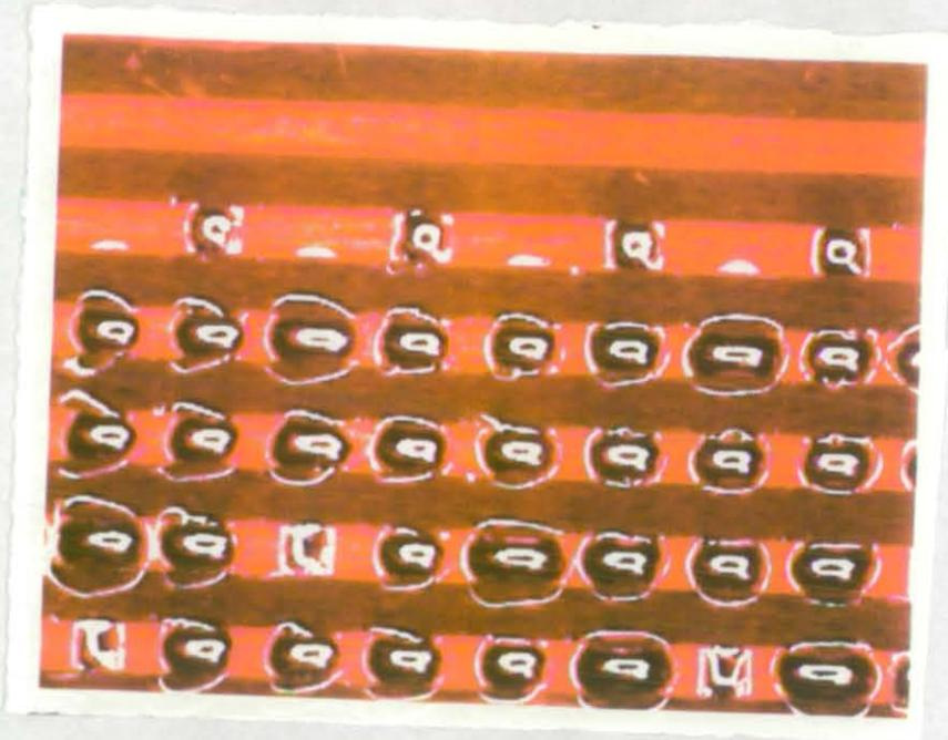
Fig. 6.9 K3 reflow at 213 deg C
