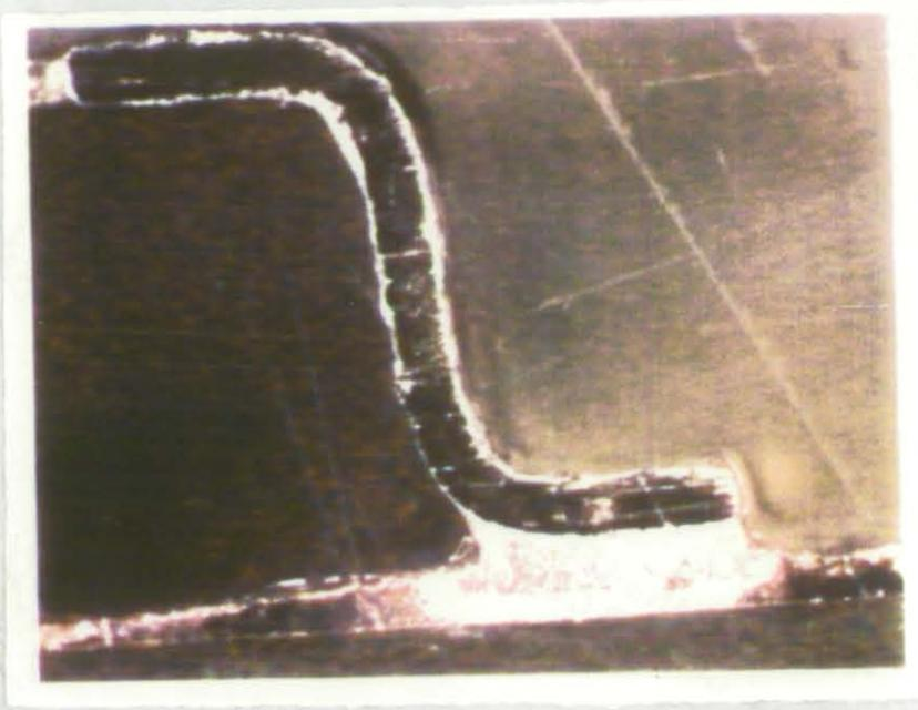
Fig. 6.21 Cross-Section of Lead Joint With Coplanarity Defect Using Kester R244
