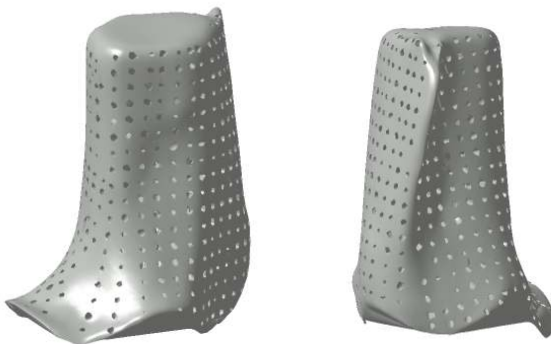
Fig. 4.19 Scaffold geometry for the mouse humerus implant analysed.
