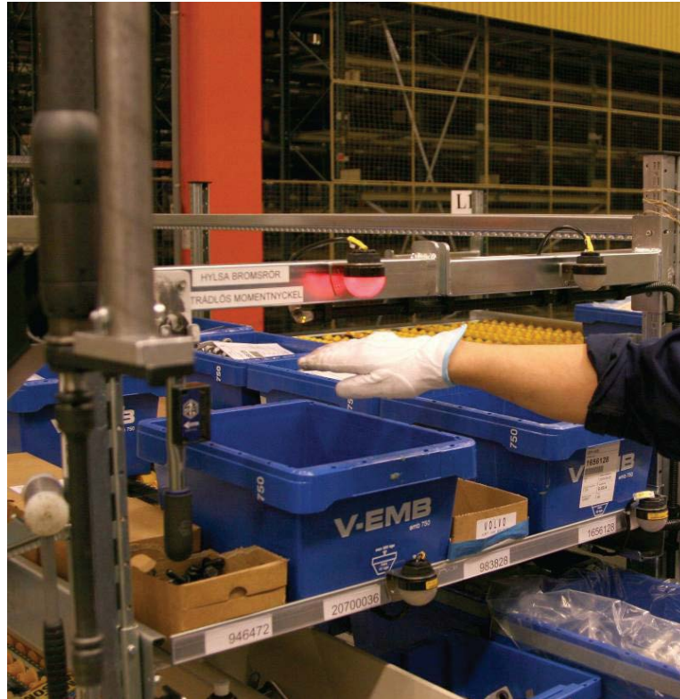
Figure 3.9. An example of pick-by-light system including a photocell verification (Bäckstrand, 2009)
