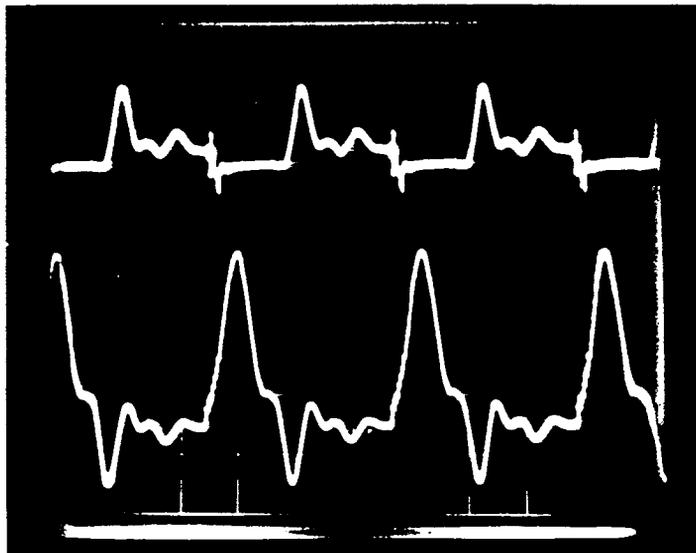
Fig.6.15 Experimental waveforms of the converter.  $V_{in}=190V_{ac}$ ,  $f_s=300kHz$
