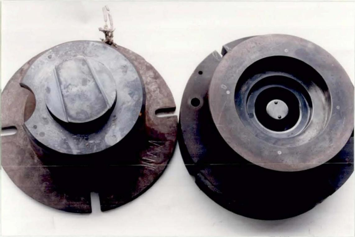
Figure 5.3(a) Die for Shaped Squeeze Casting
