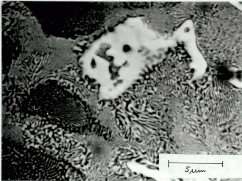
Figure 6.51 ZA27 (SEM) 12mm Section
