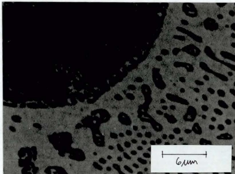
Figure 6.63 ZA12 (SEM) 50mm Section
