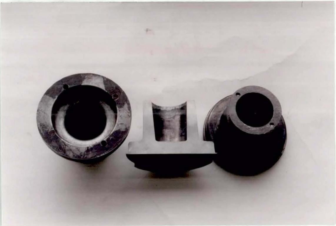
Figure 5.3(b) Squeeze Castings from Shaped Die
