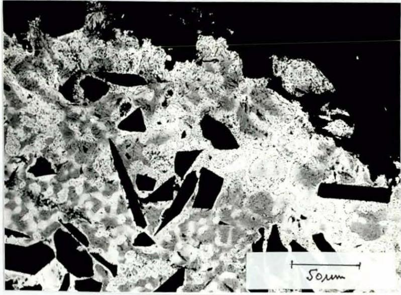
Figure 6.98 ZA27 + 20 vol% SiCp (SEM) 50mm Section
