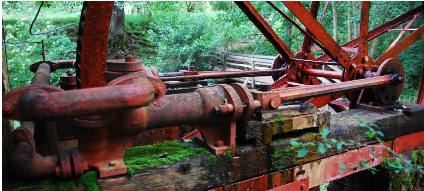
Figure 2.1 - Piston driven water pump with two connecting rods
