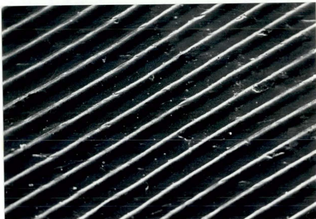
Plate 35. Photomicrograph of the Surface of Embossed Plastic Metal Input 0.58\mu\text{m} - Plastic Groove Depth 0.47\mu\text{m}
