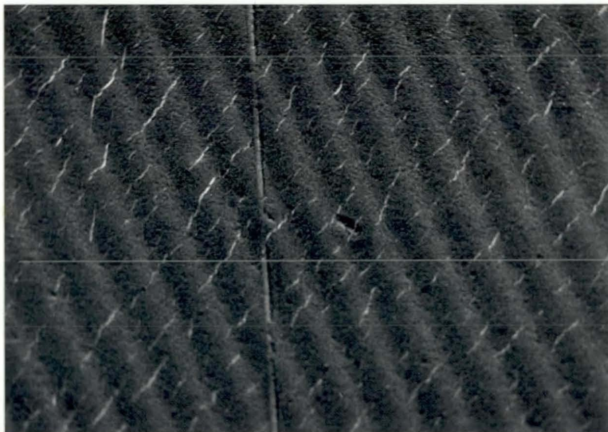
Plate 34. Photomicrograph of the Surface of Embossed Plastic Metal Input 0.16\mu\text{m} - Plastic Groove Depth 0.10\mu\text{m}
