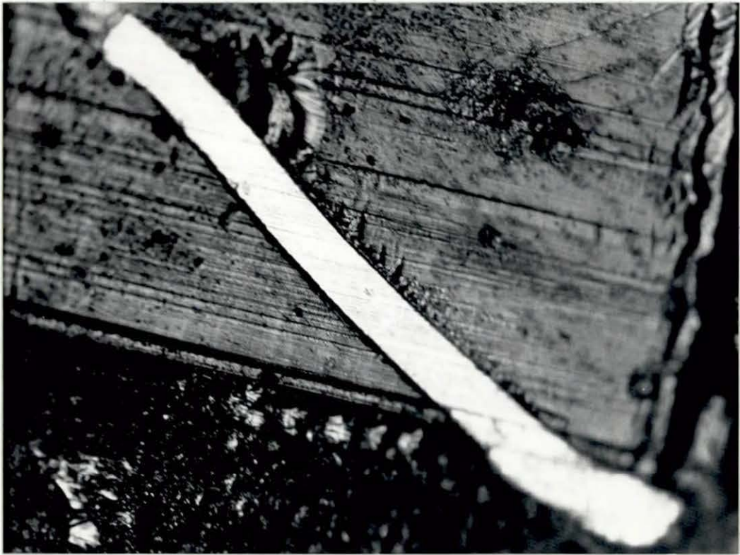
Plate 18. Metal Section Mounted into Epoxy Resin
