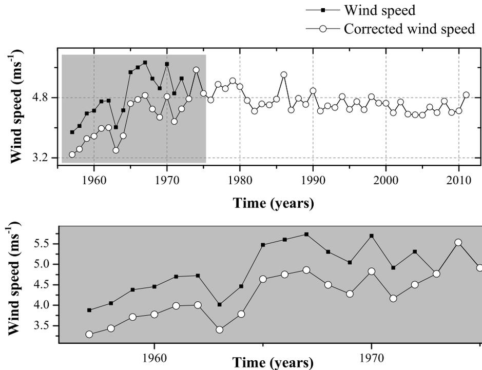
Figure 3.7: Correction in instrumentation's effective height
