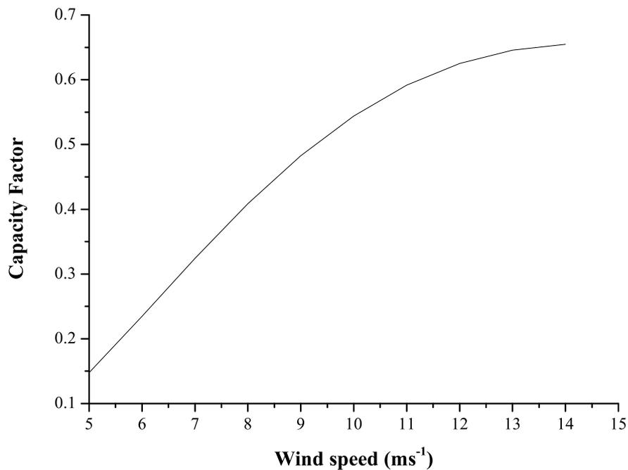
Figure 4.10: Capacity factor of a Vestas V80 2MW turbine as a function of mean wind speed
