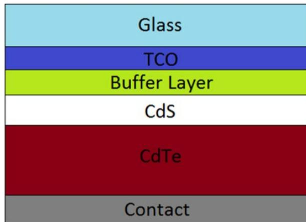
**Figure 7.1:** A schematic diagram of the CdTe solar cell structure showing the position of (from bottom to the top), the back contact, the CdTe absorber, the CdS window layer, the buffer layer, the TCO layer, and the glass substrate.
