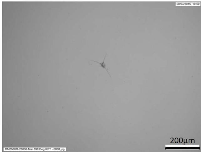
**Figure 6.6: Optical microscope images of a sputtered SiO<sub>2</sub>/ZrO<sub>2</sub> MAR sample exposed to 590°C for 30 min, showing an isolated fissure in the surface of the coating.**
