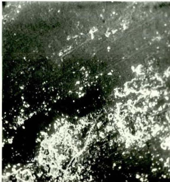
Fig.129 - SEM Micrograph for Compocast Worn Surface
