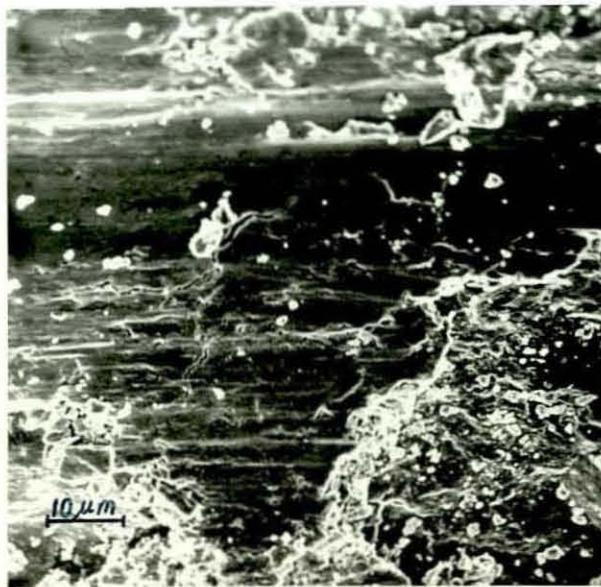
Fig.117 - SEM Micrograph for Gravity Die Cast Worn Surface (Dry Friction)
