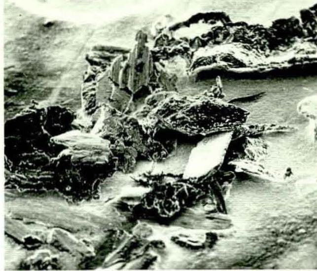
Fig.124 - Debris of the Base Alloy (No Graphite Addition)
