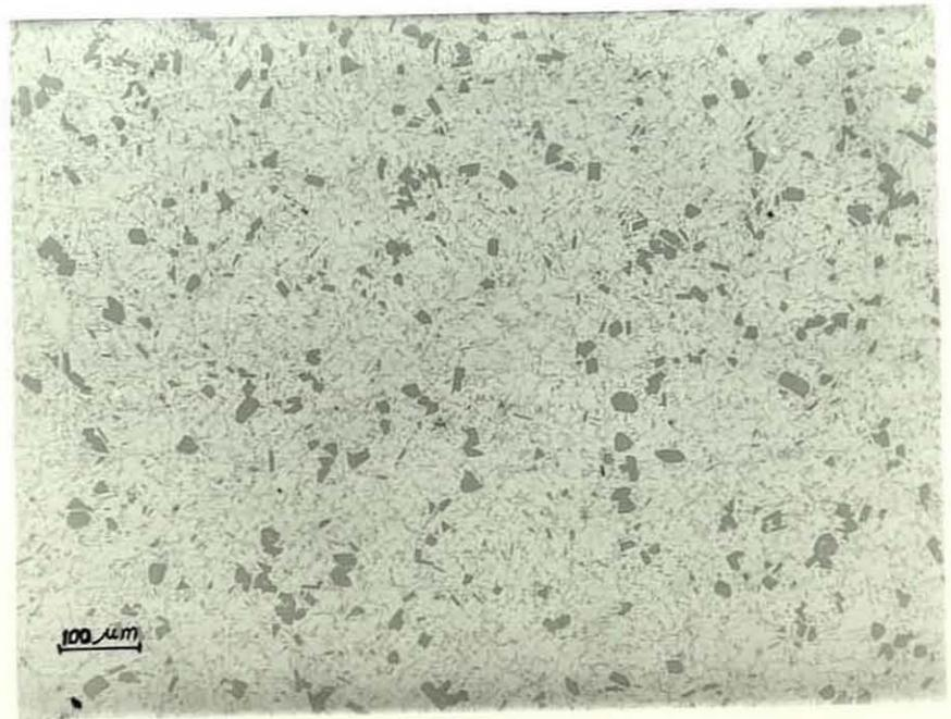
Fig.39 - LM30 - Gravity Diecast Structure
