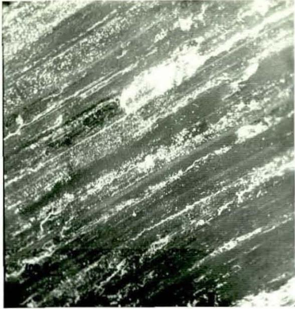
Fig.128 - SEM Micrograph for Compocast Worn Surface
