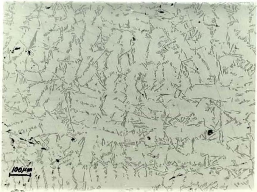
Fig. 30 - Aluminium - 8% silicon alloy
