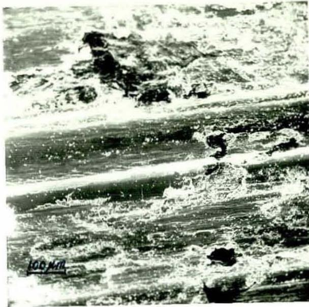
Fig.132 - SEM Micrograph for Compocast Worn Surface
