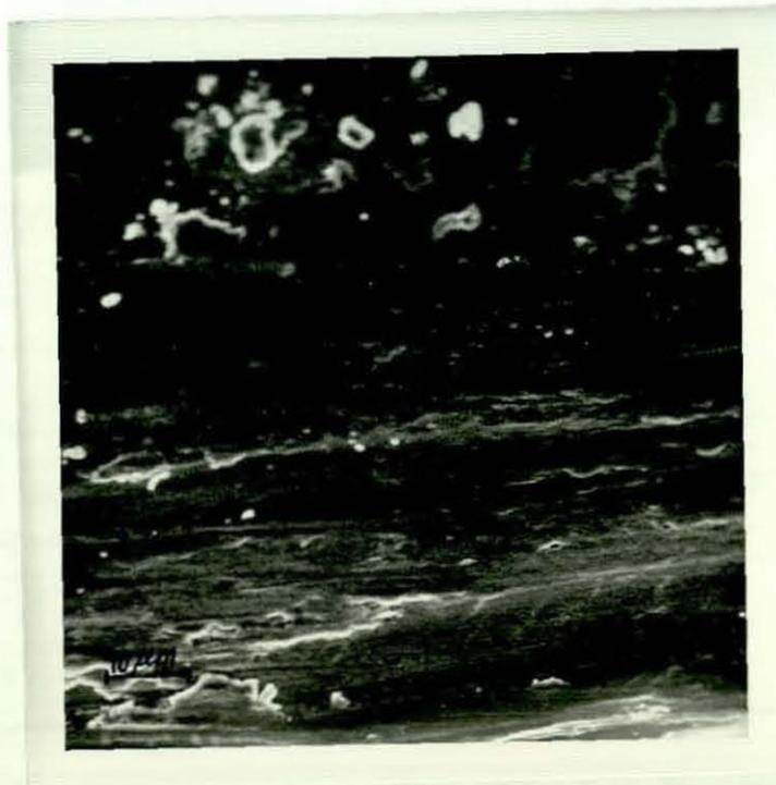
Fig.133 - SEM Micrograph for Compocast Worn Surface
