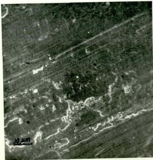
Fig.137 - SEM Micrograph for Compocast Worn Surface
