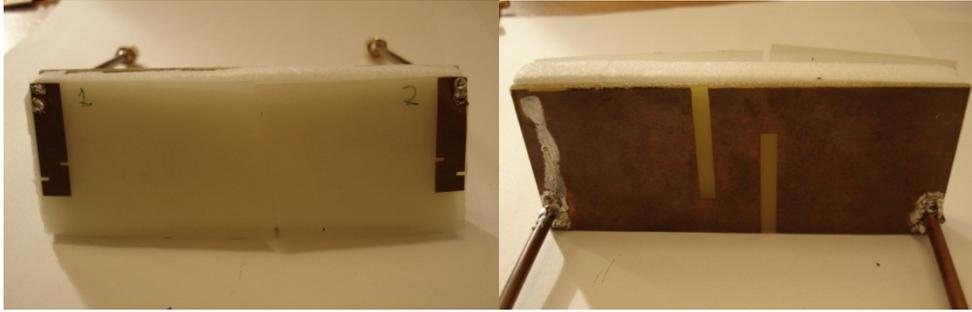
Figure 3.20 Prototype system using the proposed slitted ground plane
