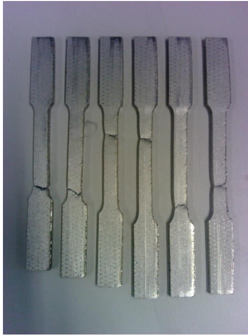
Figure 5-25 Break specimens built for dark particles effect study
