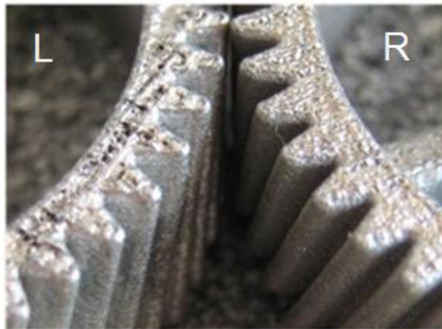
Figure 5-14 Top surface improvement through re-melting process, L is the original part, R has been re-melted on the top surface
