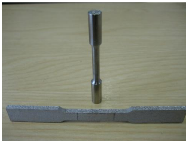
Figure 5-15 Tensile test specimens built for build directions study
