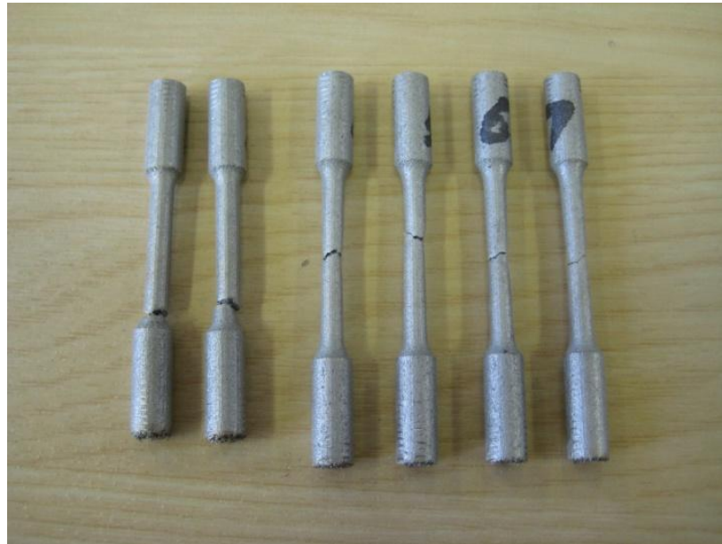
Figure 5-17 Tensile test specimens with/without topping up delay during the process have been pulled
