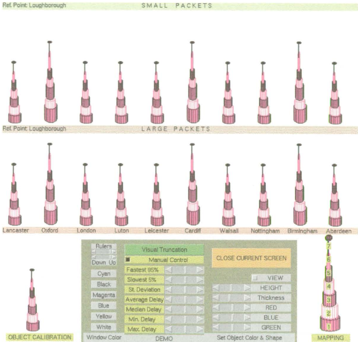
Figure 20: An FD-Interface using a telescopic-antenna to accommodate 7 parameters.
