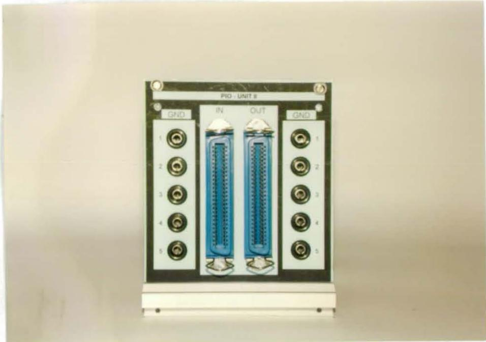
**Photo D14:** Front view of the PIO Unit module II
