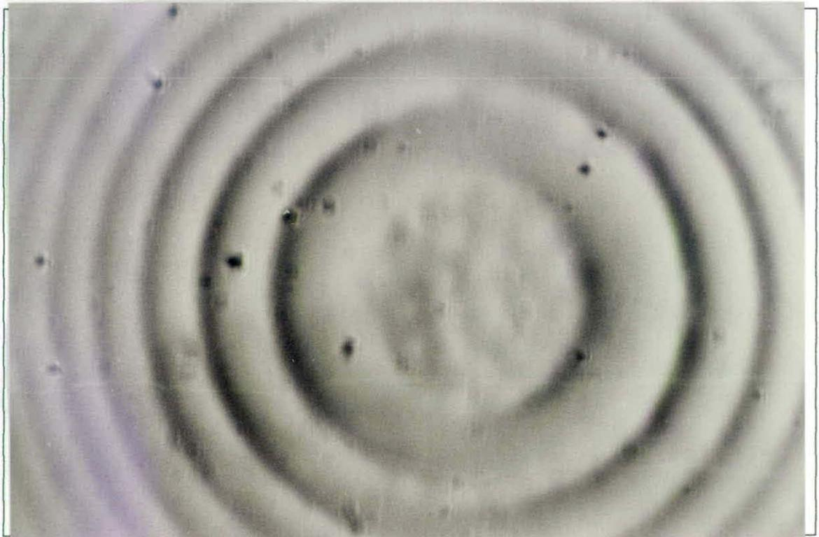
**Fig. 63:** Continuous ring structure produced by post melting
