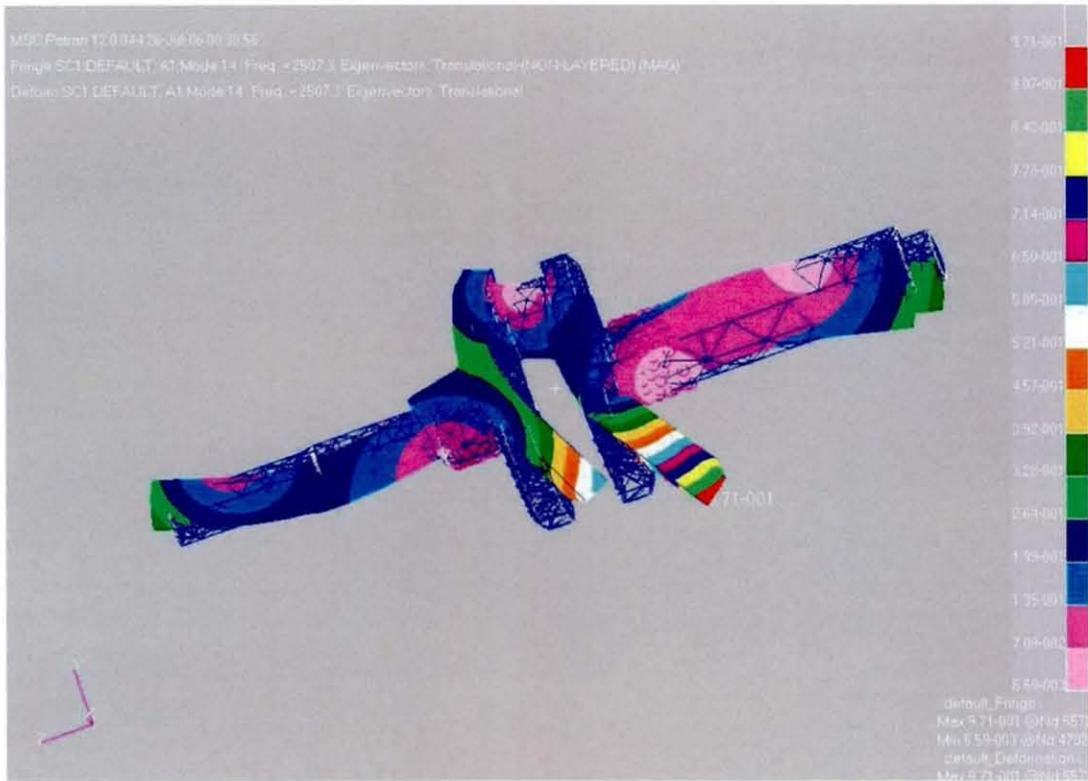
**Figure 3.7 Super-element Crankshaft – Mode shape for the frequency of 2704Hz (created using MSC/Nastran)**
