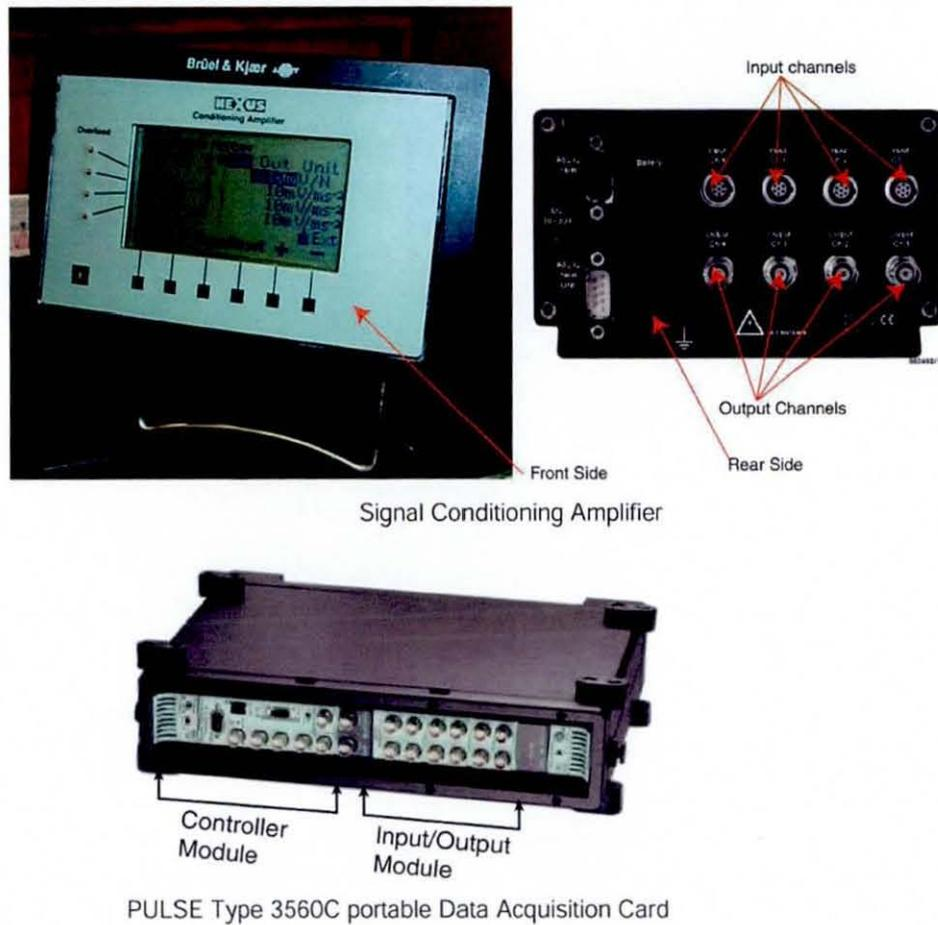
Figure 6.13 Bruel & Kjaer Conditioning Amplifier and DAC system
