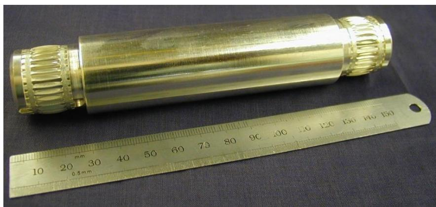
Figure 6.11 HV electrode bar of spark gap
