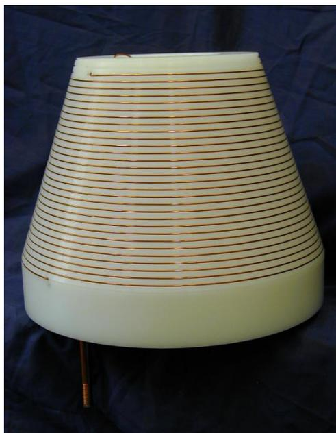
Figure 2.5 Secondary winding of Tesla transformer
