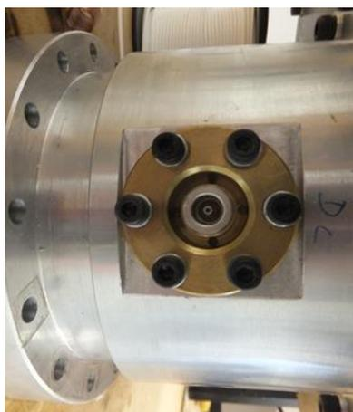
Figure 5.4 Voltage sensor mounted on coaxial load
