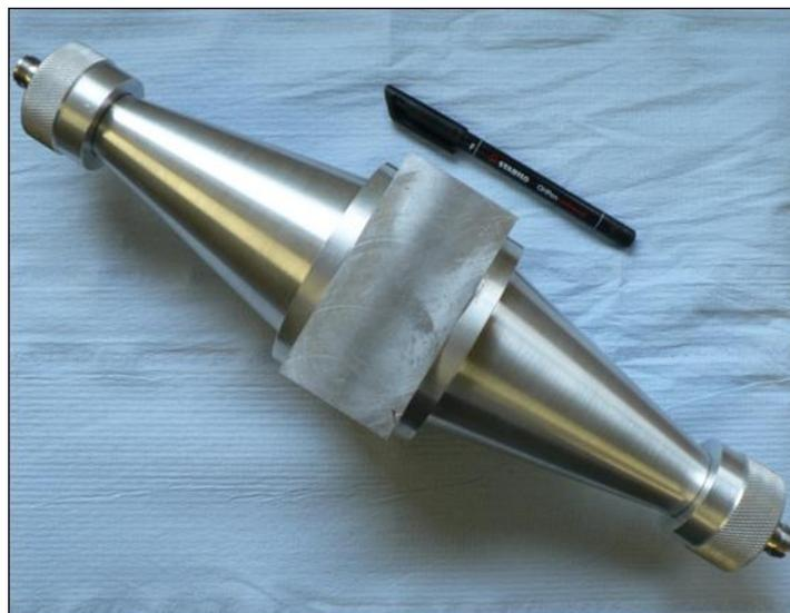
Figure 5.23 Biconical transmission line arrangement
