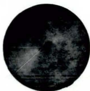
Figure 7. Microphotographs of the near field patterns observed when a 40 cm. length of single fibre was illuminated by white light.
