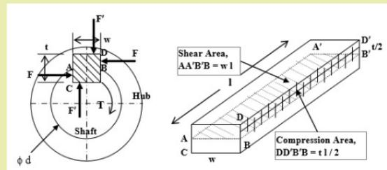
Figure 2.2: Forces acting on keys and stress areas.
