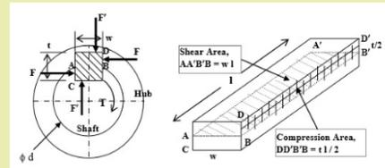
Figure 2.2: Forces acting on keys and stress areas.
