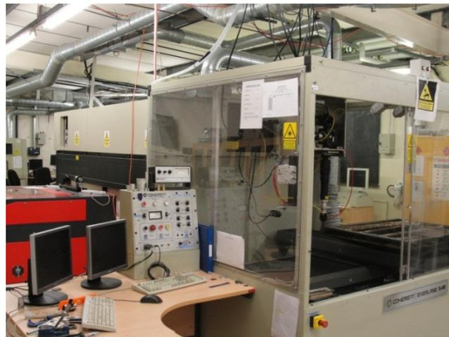
Figure 3-3 1.2kW Carbon dioxide (CO<sub>2</sub>) coherent S48 laser systems
