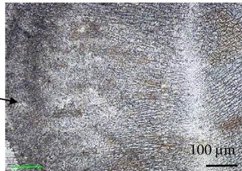
(d) Magnified image showing growth of columnar dendrites perpendicular to the weld boundary
