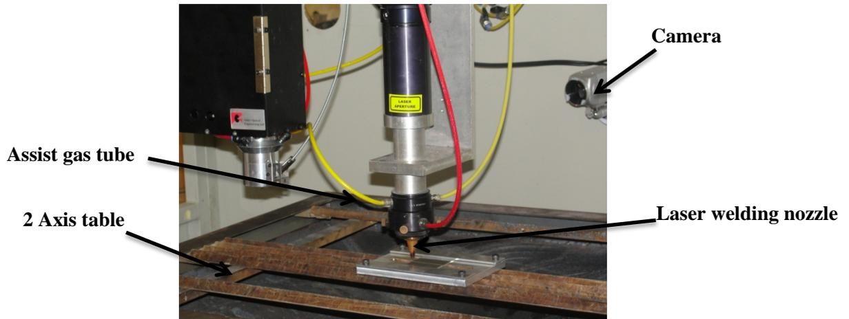
Figure 4-1 Experimental setup used for laser welding
