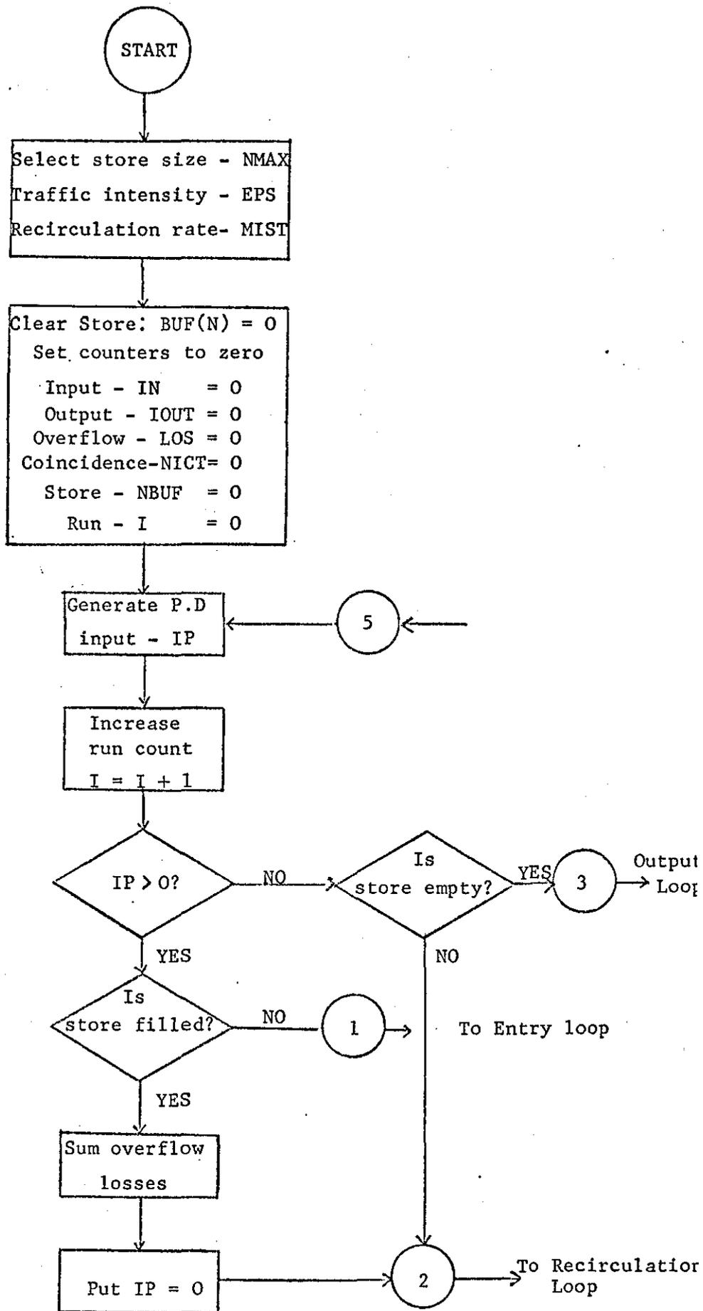
Figure A.5(1): Simulation of a single channel recirculating store with Poisson input.
