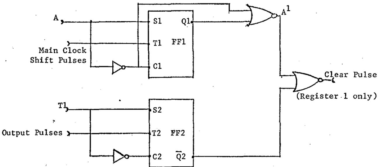
Figure 5.14C: Circuit implementation of Clear Pulse process.
