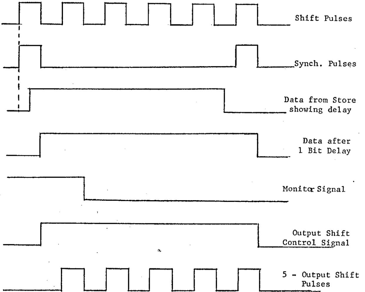
Figure 5.13B: Waveforms showing the production of the 5 - Output Shift Pulses.
