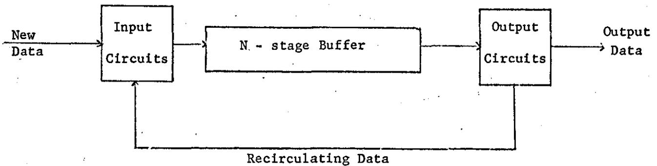
Figure 3.3 The recirculating storage system
