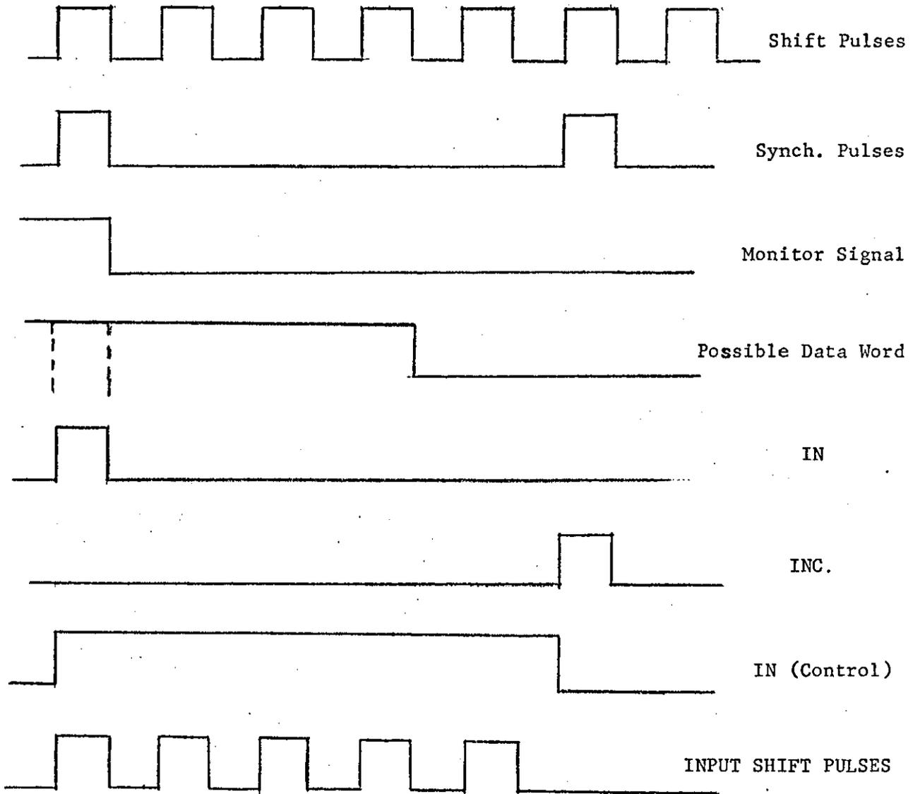
Figure 5.11A: Waveform Diagram for Input-Output Decision Circuits.
