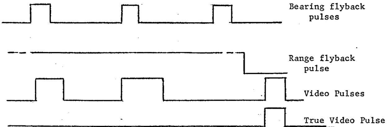
Figure 5.4B: Waveform diagram for flyback blanking.
