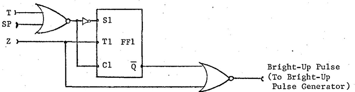
Figure 5.17C: Bright-Up pulse circuit.
