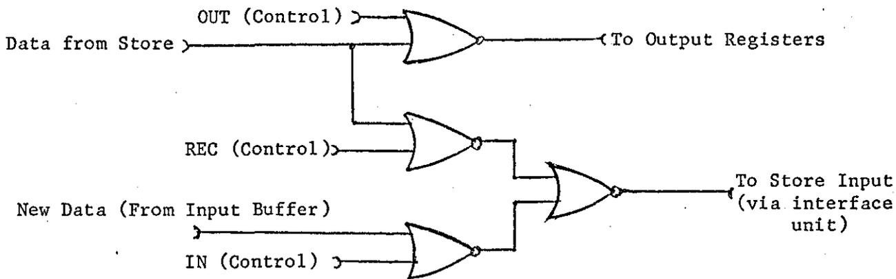
Figure 5.11C: Steering Circuit.
