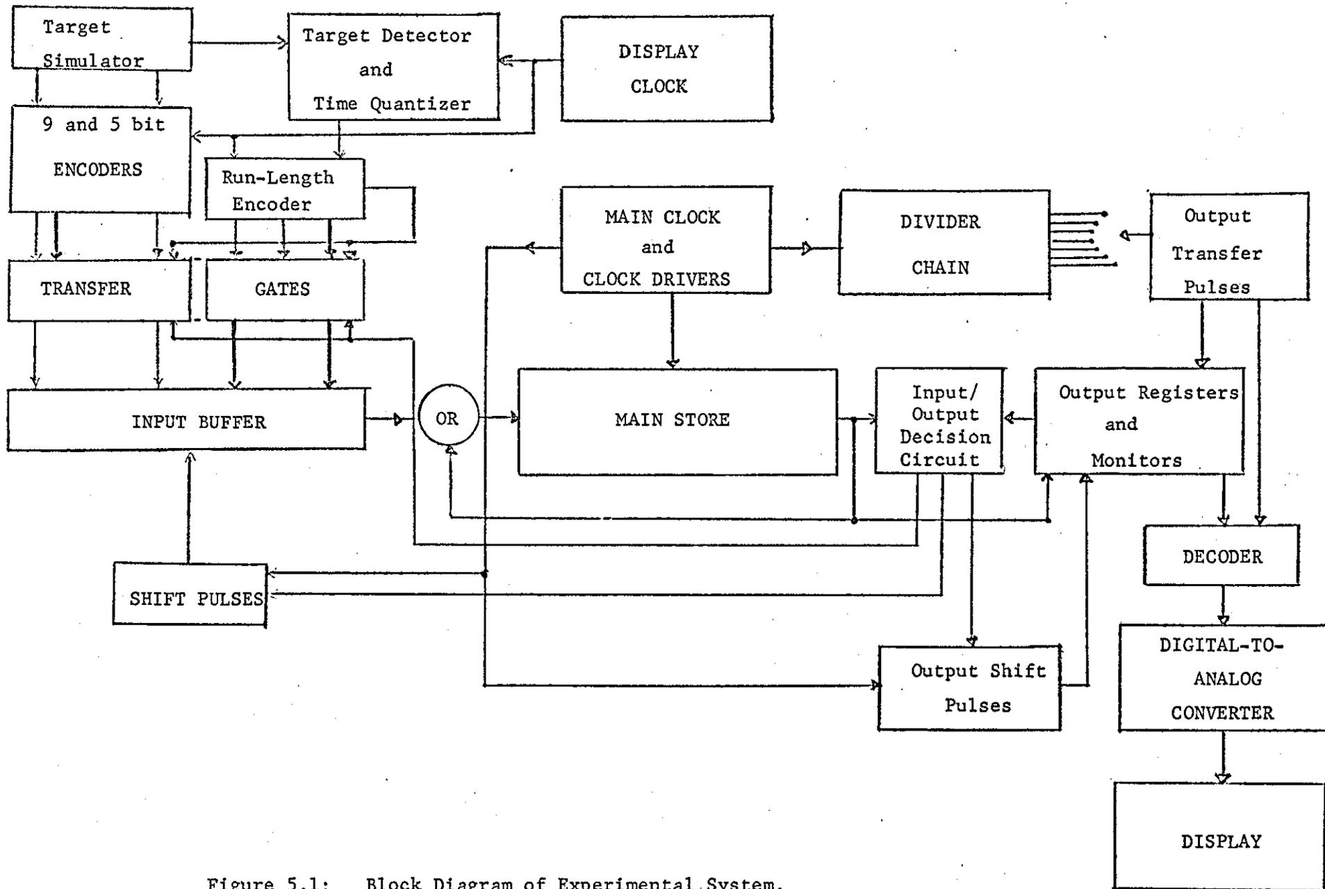
Figure 5.1: Block Diagram of Experimental System.
