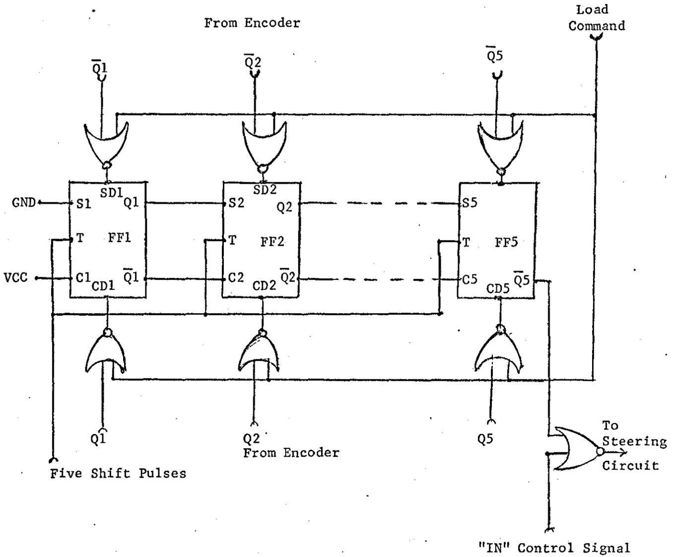
Figure 5.9: Circuit Diagram of Input Register.
