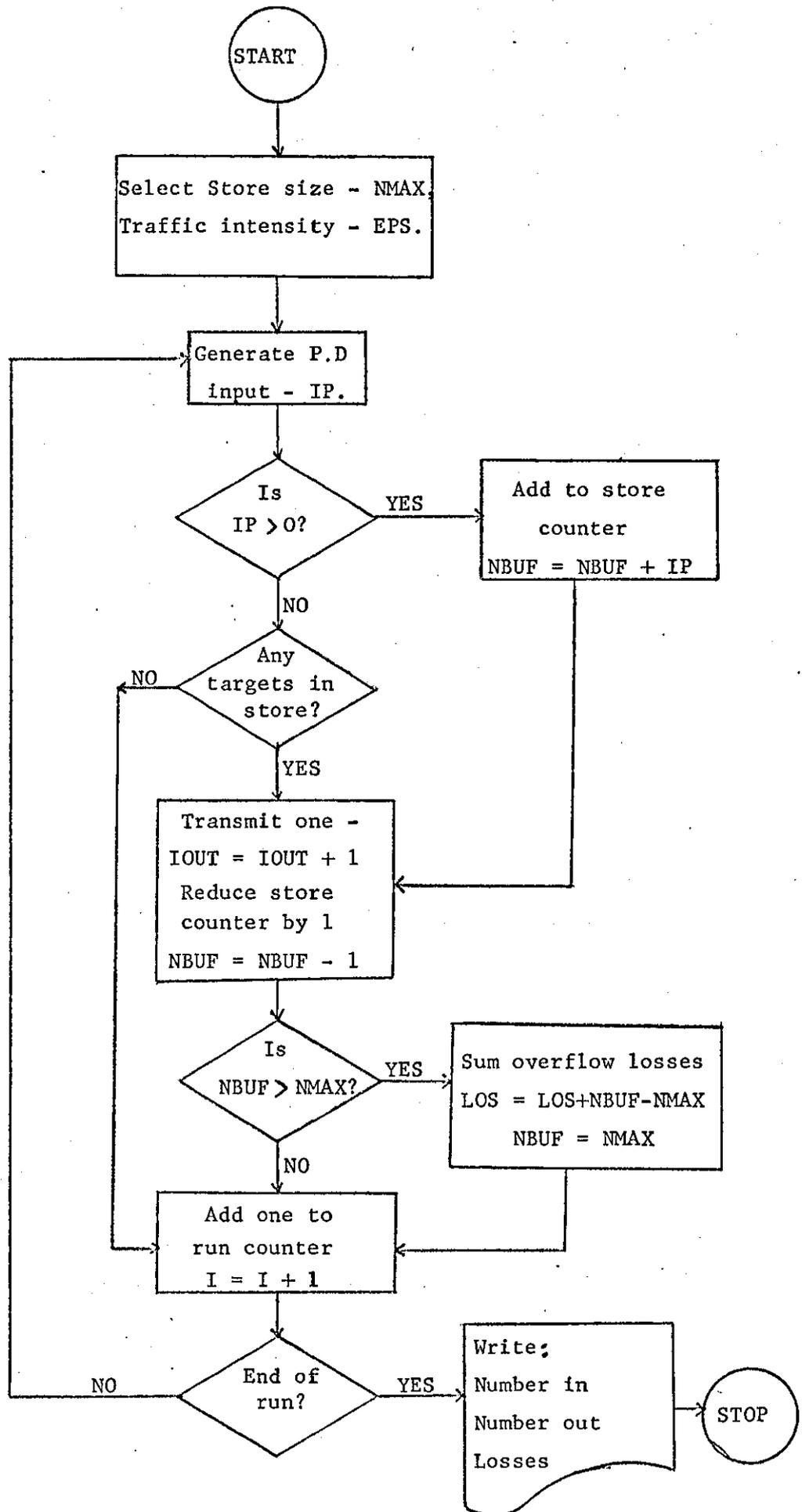
Figure A.3: Simulation of step-down store with Poisson input.
