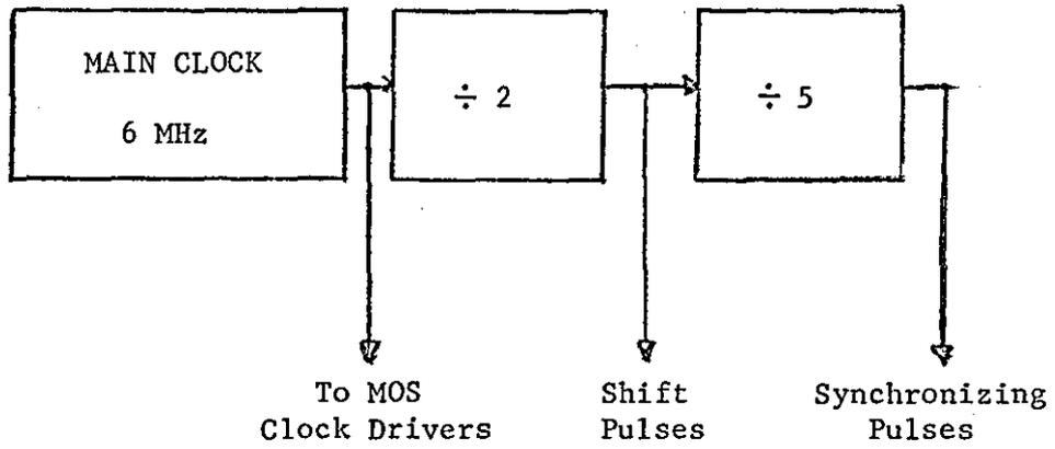
Figure 5.10A: Block Diagram of Main Clock System.
