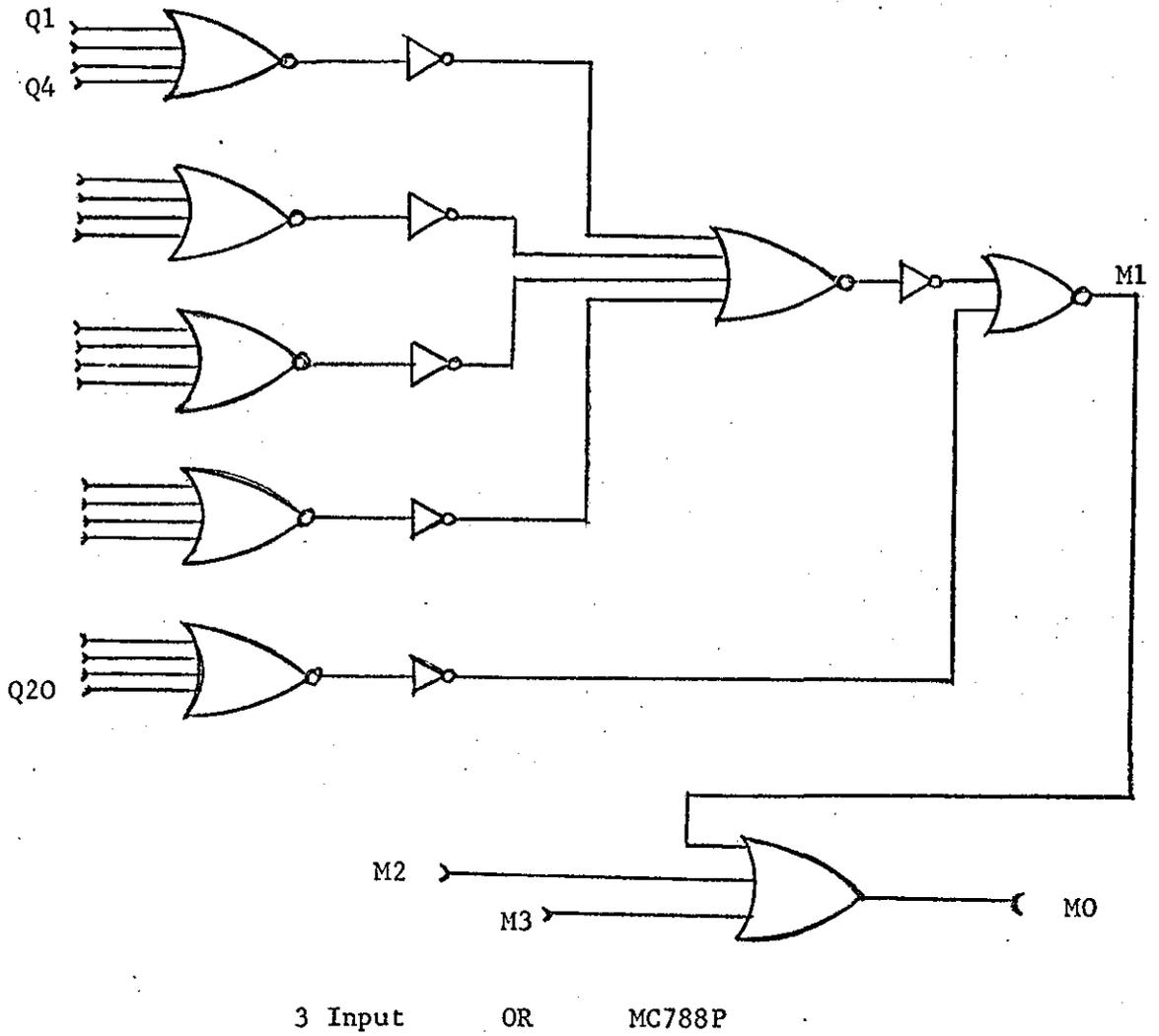
Figure 5.12: Circuit Implementation of State Monitor.
