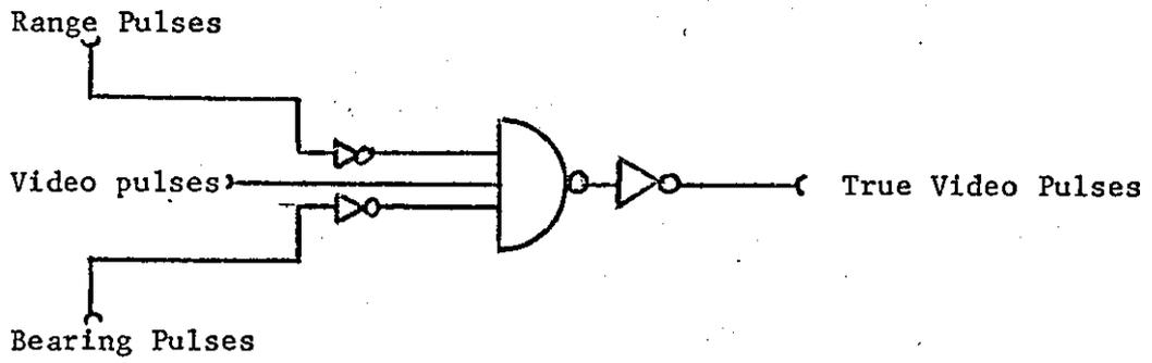
Figure 5.4A: Flyback blanking circuit.
