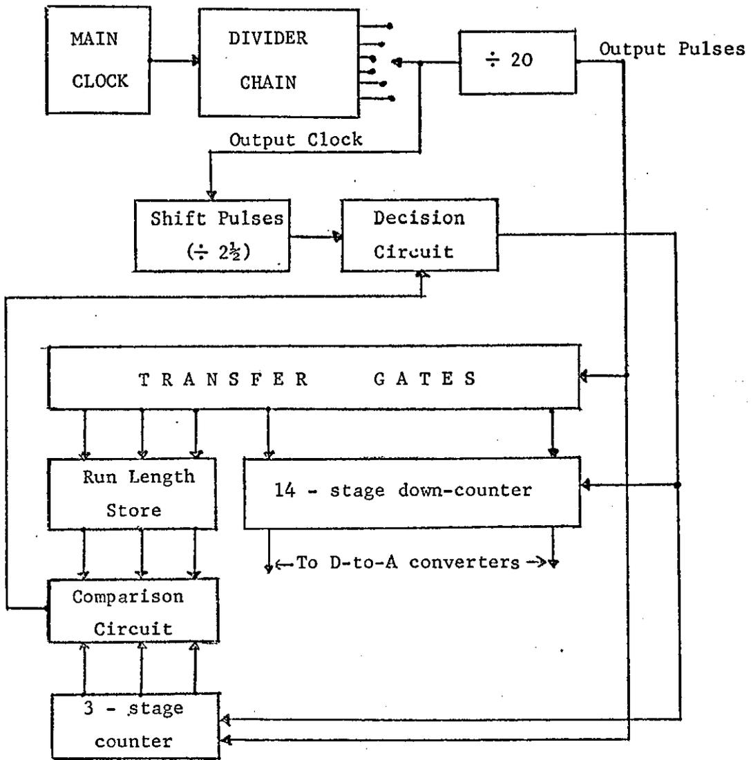
Figure 5.15A: Block Diagram of Output Decoder.
