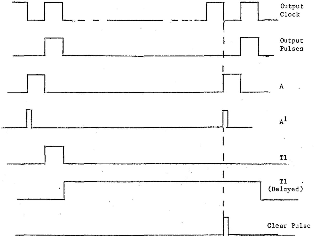
Figure 5.14B: Waveform diagram showing production of clear pulses.
