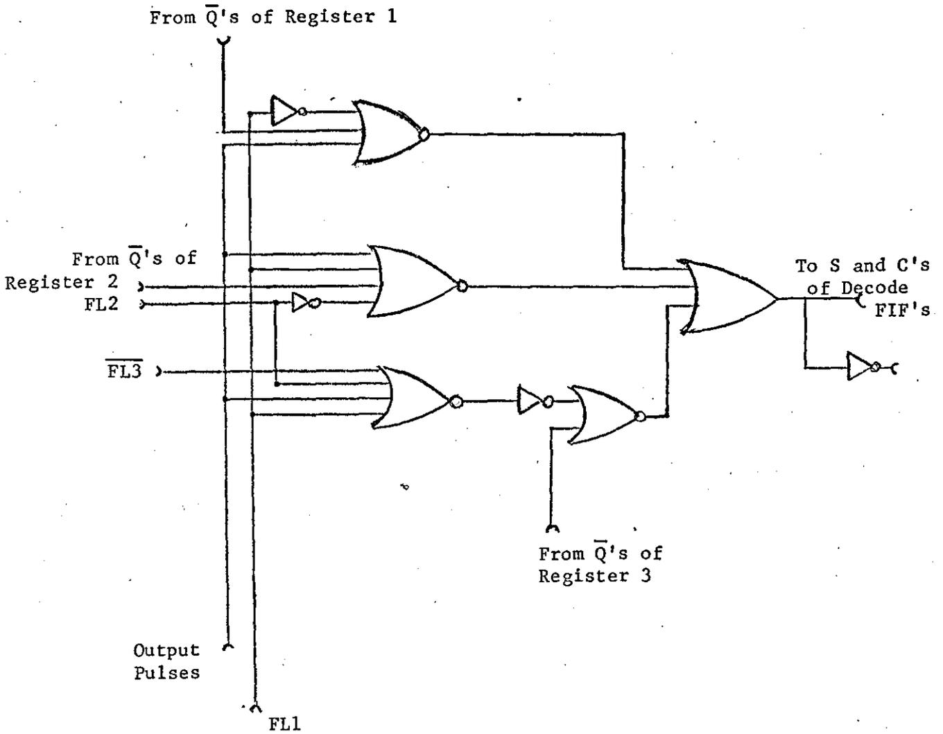
Figure 5.14A: Circuit implementation of Output Transfer Circuit.
