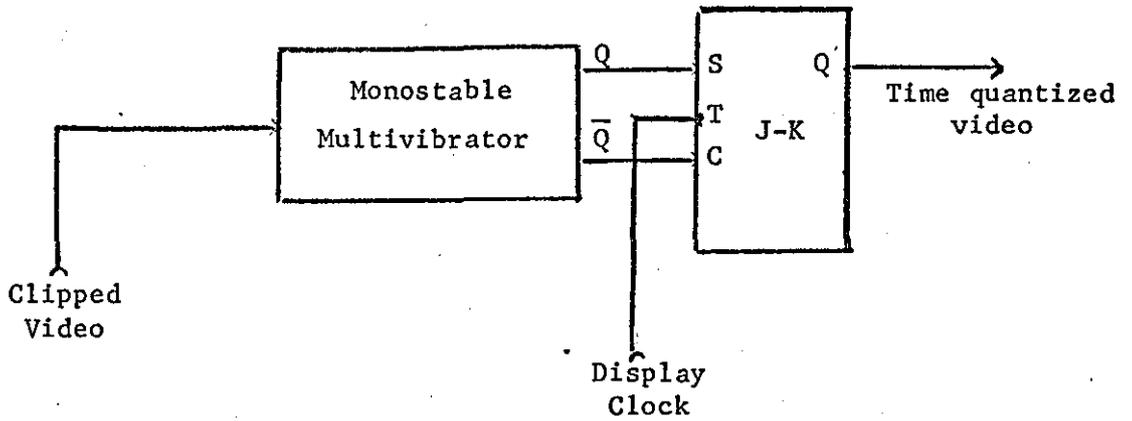
Figure 5.5A: Time Quantization Circuit.
