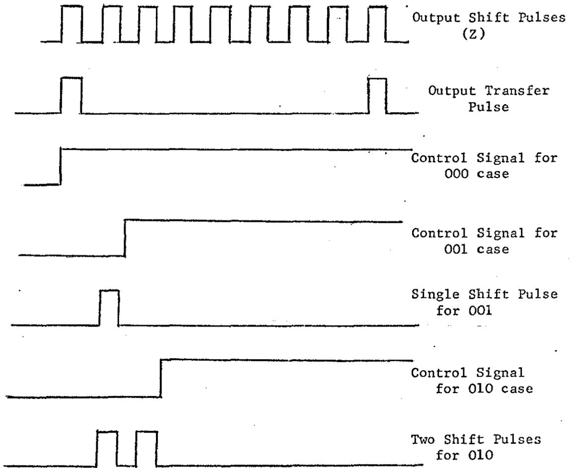
Figure 5.15C: Waveform diagram showing operation of Decoder Circuit.
