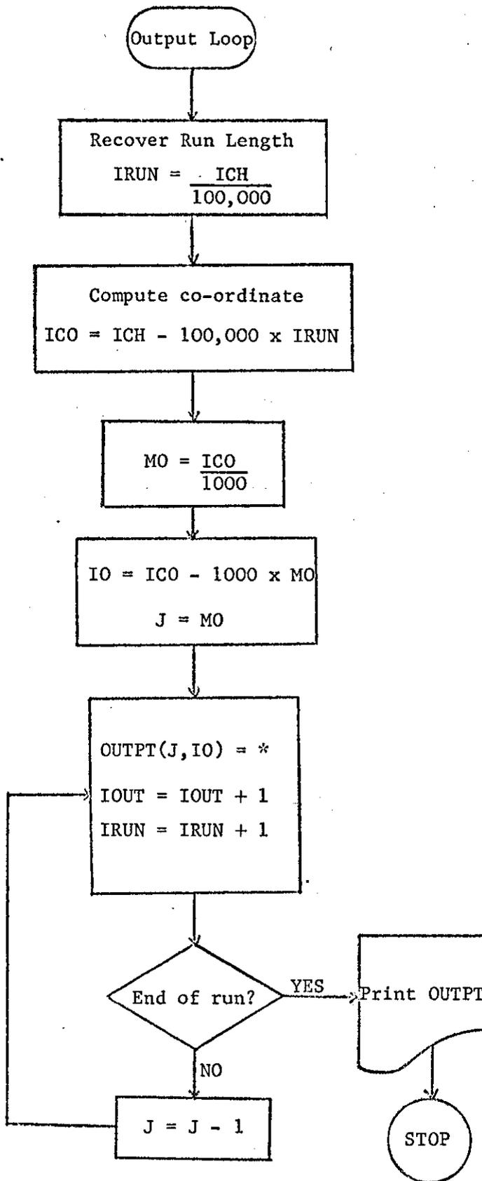
Figure A.10: Decoding process for run-coded inputs.
