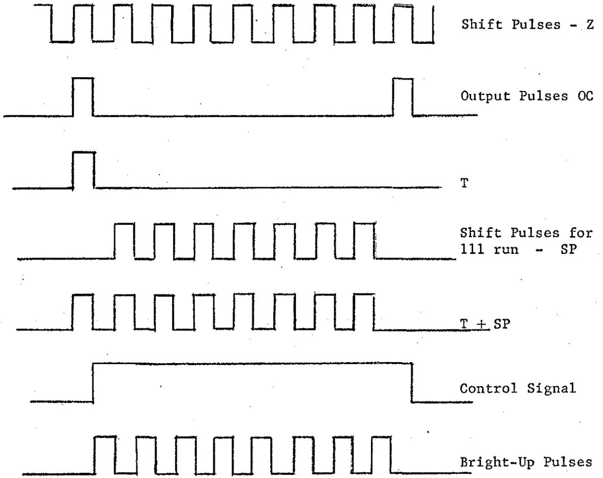
Figure 5.17B: Waveform diagram for Bright-Up Pulse generation.
