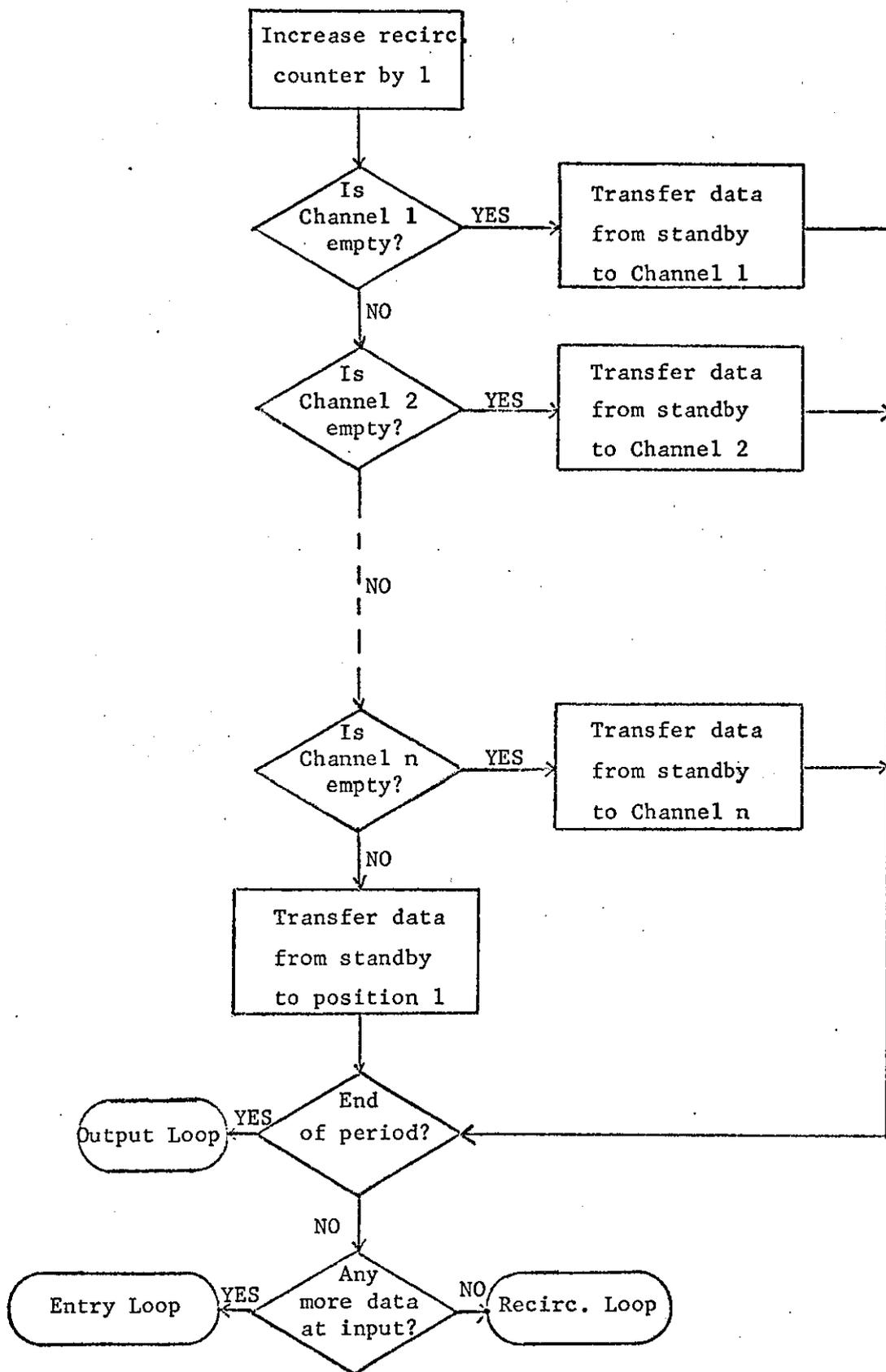
Figure A.6: Modifications to recirculation loop for multiple channels.
