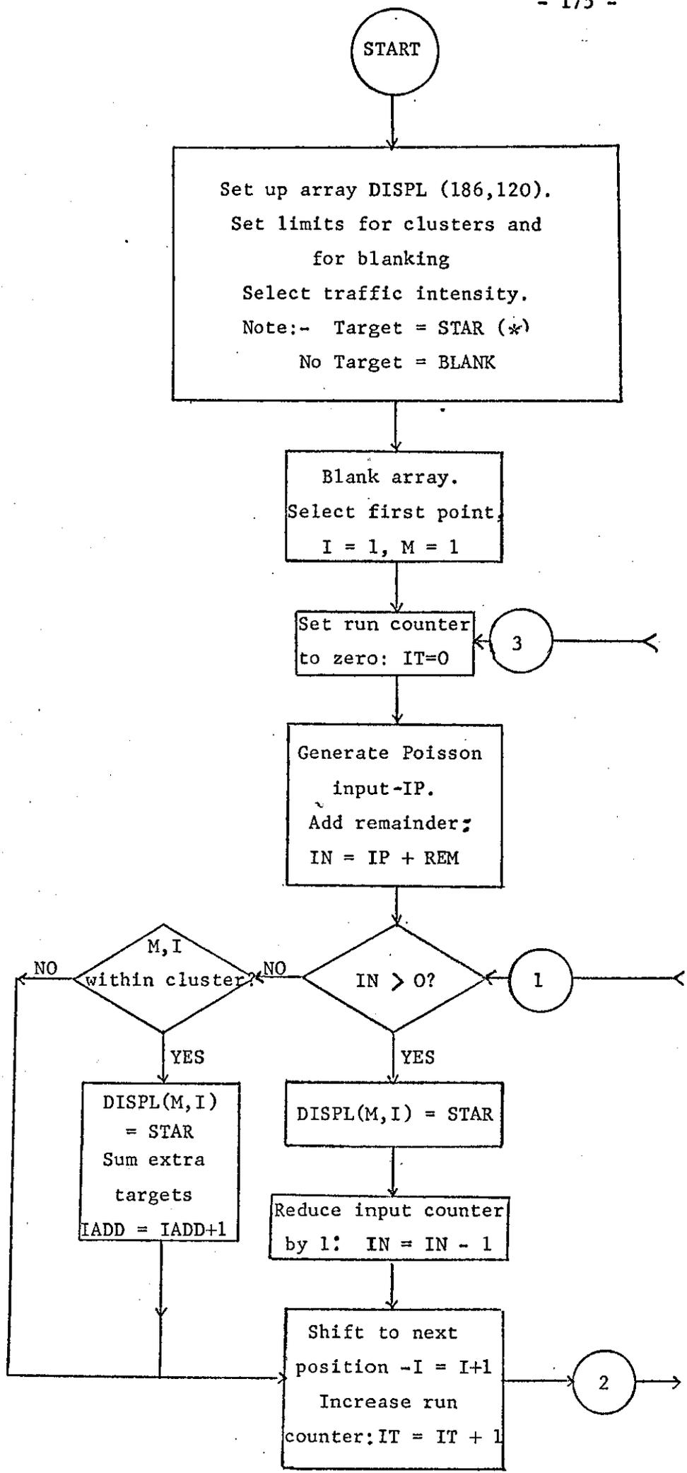
Figure: A.2(1): Generation of Test Pattern.
