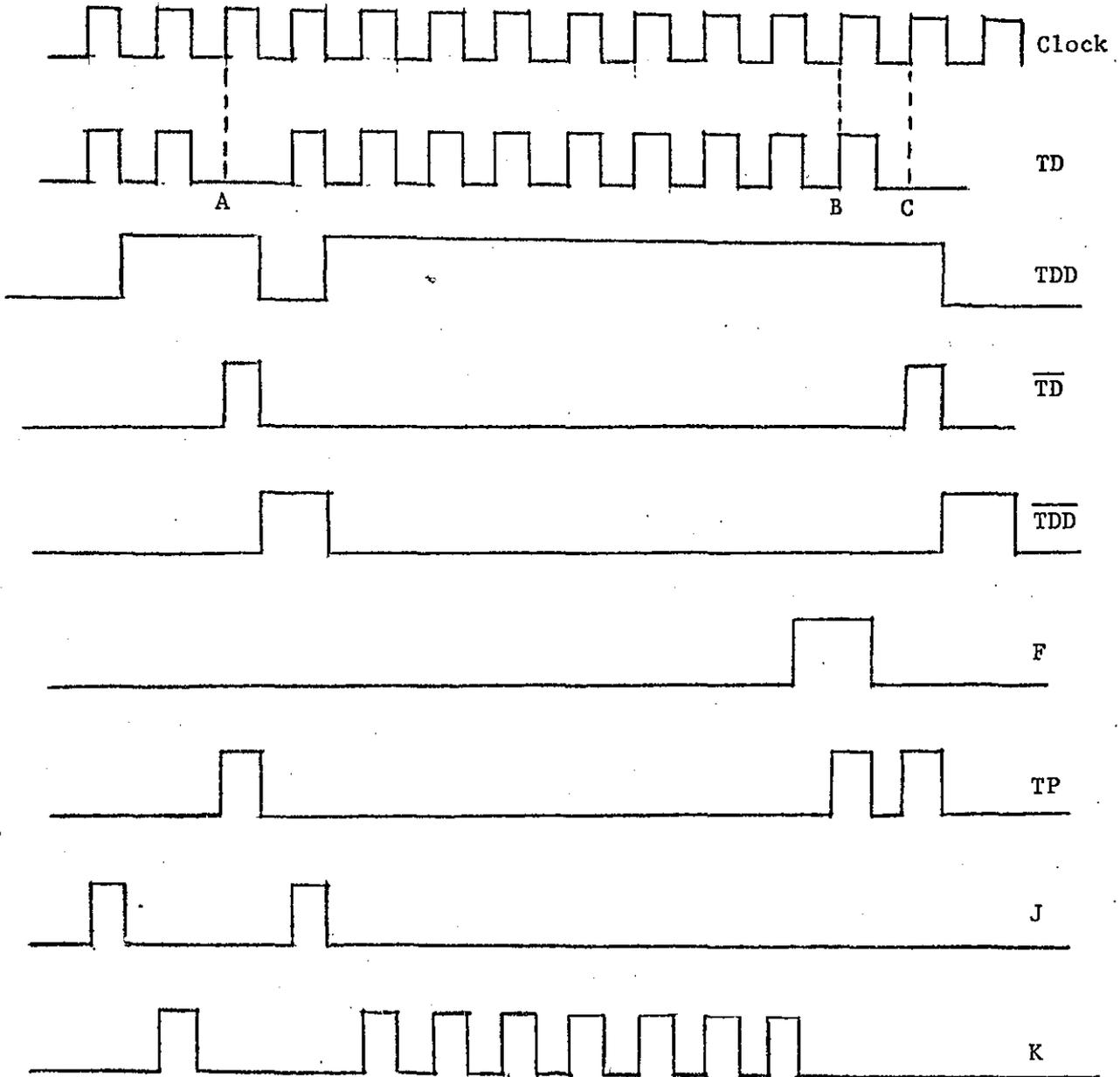
Figure 5.7B: Waveform Diagram showing the operation of the Run Length Decision Circuit
