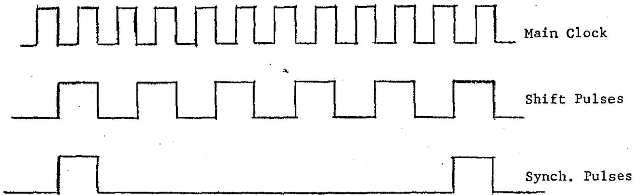
Figure 5.10B: Waveform Diagram of Clock System.
