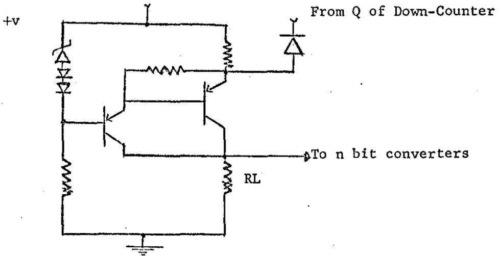
Figure 5.16: Circuit diagram of single bit converter of Digital-to-Analog converter.
