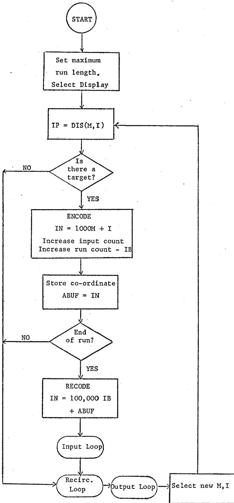
Figure A.8: Run Length Coding using Method 1.
