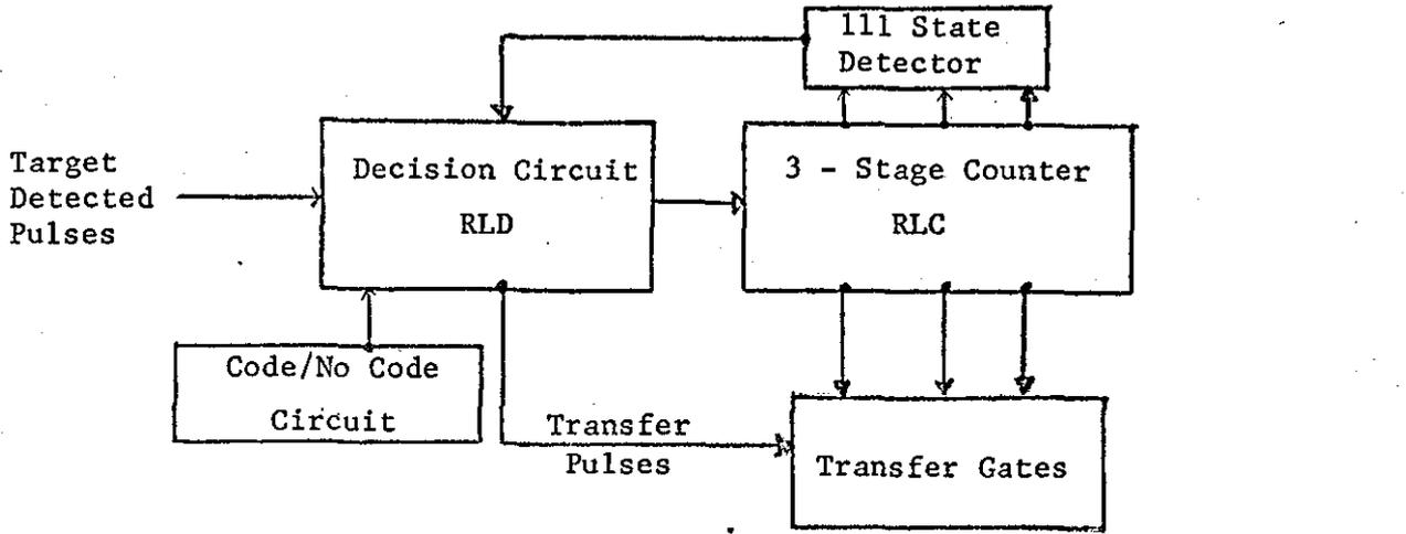
Figure 5.7A: Block Diagram of Run Length Encoder.
