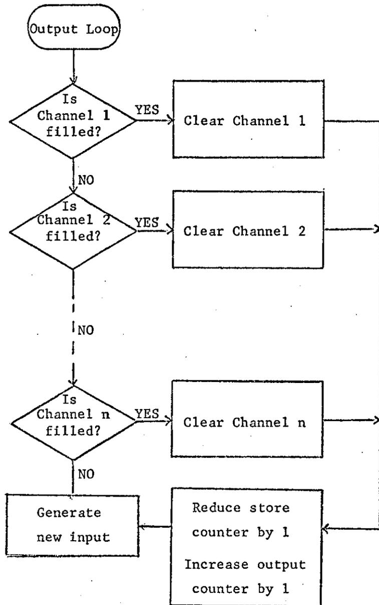
Figure A.7: Modifications to output loop for Multiple Channels.
