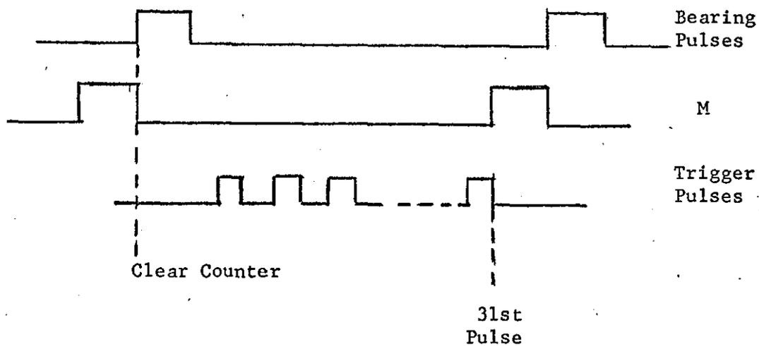
Figure 5.6C: Waveform diagrams for Bearing Digitizer.
