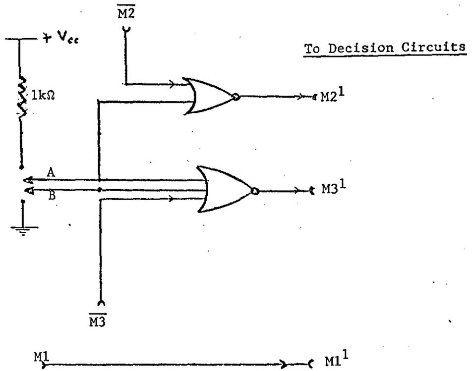
Figure 5.17A: Circuit Implementation of Output Registers Selector.
