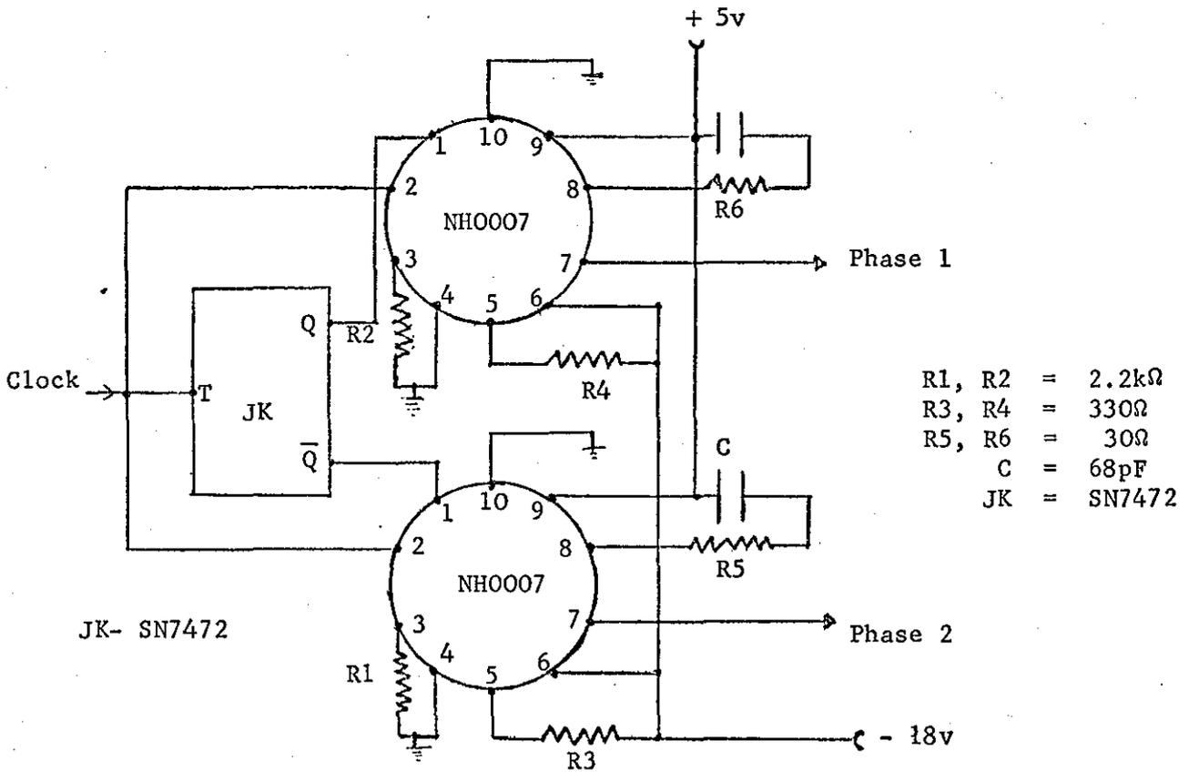
Figure 5.8E: Two Phase clock system.
