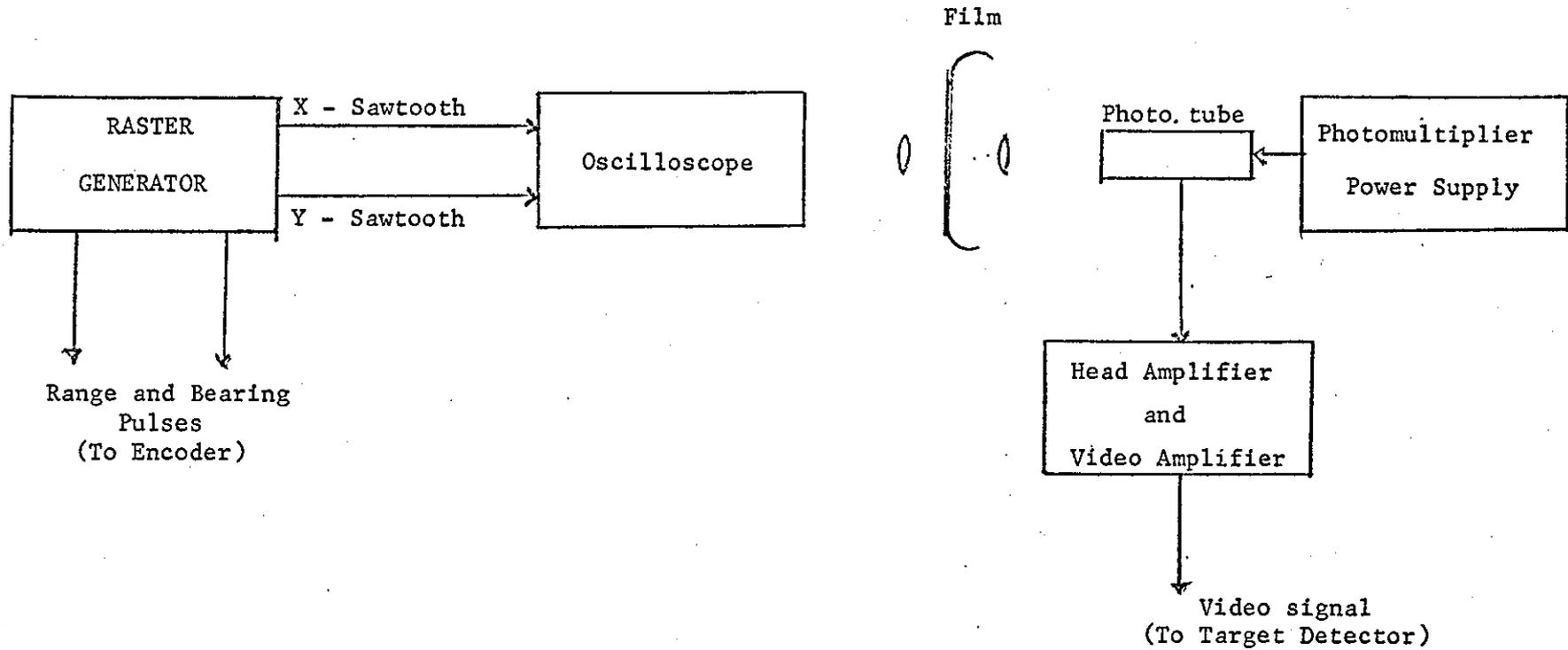
Figure 5.2: Block Diagram of Target Simulator.
