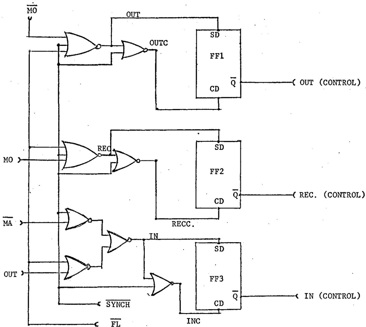
Figure 5.11B: Implementation of Input-Output Control Circuits.
