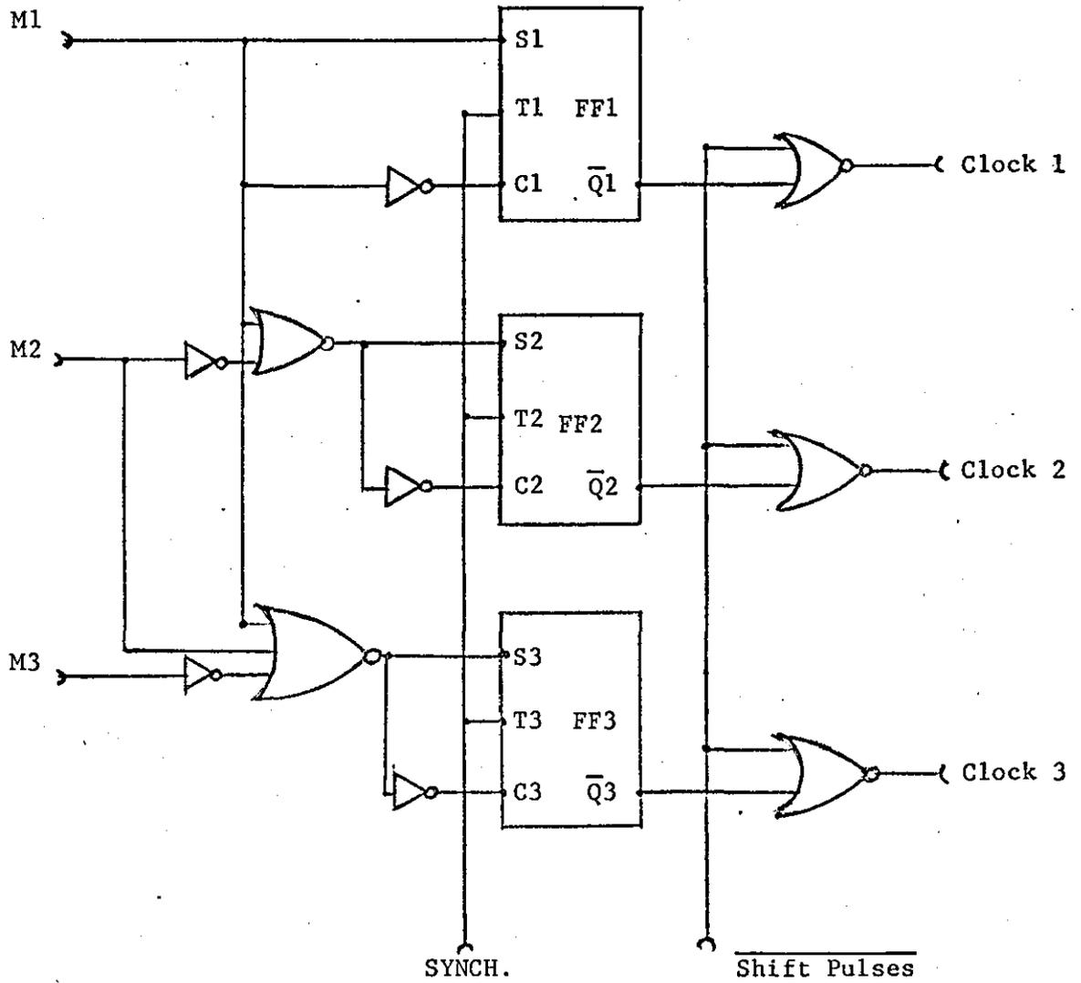
Figure 13A: Implementation of Output Shift Pulses Generator.
