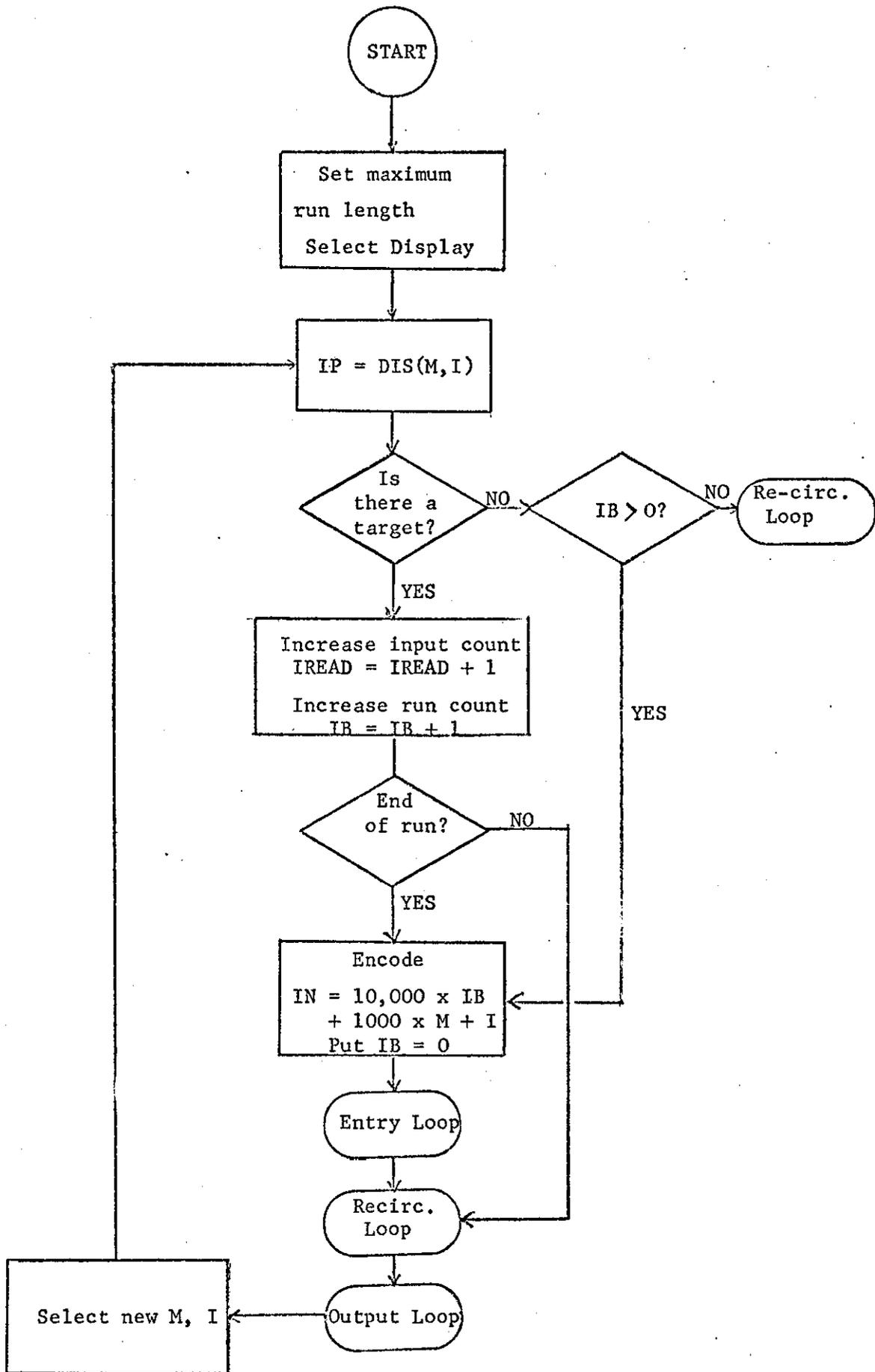
Figure A.9: Run Length Coding using Method 2.
