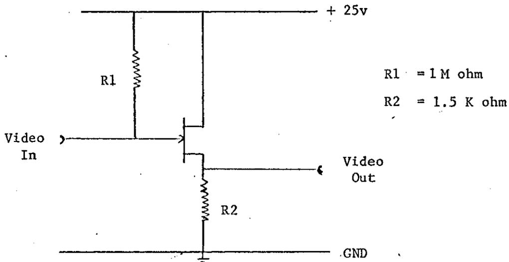
Figure A.12: Head amplifier for video signal.
