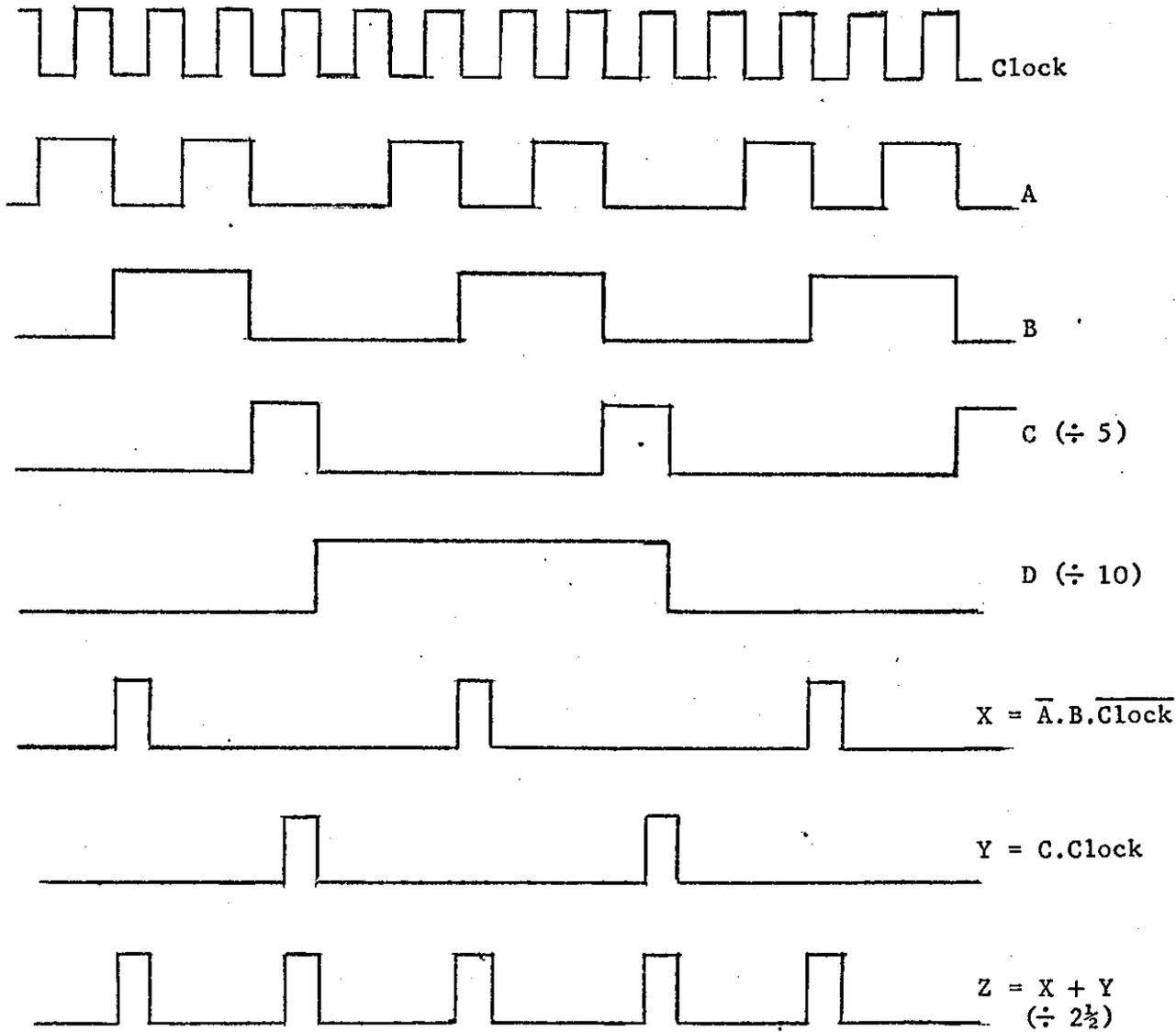
Figure 5.15B: Waveform Diagrams for performing the Divide-by-2½ operation.
