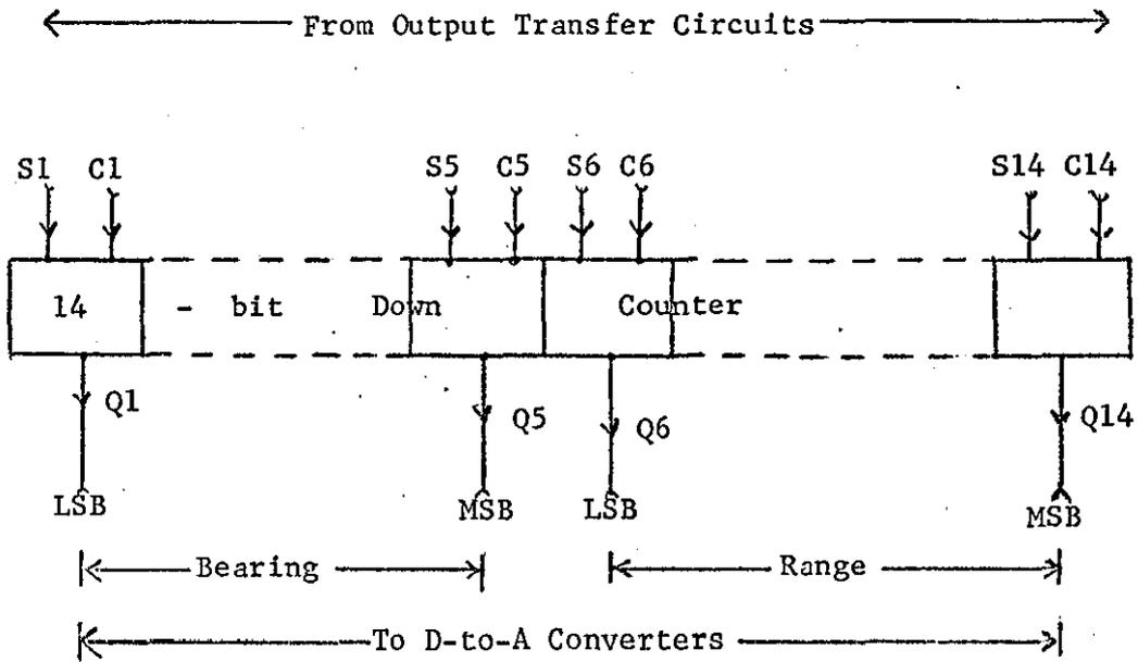
Flip-Flops used in Down-Counter -SN7476
