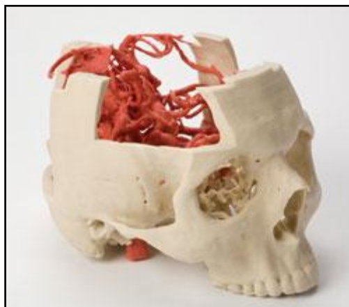
Figure 1: Physical model of main arteries in skull, produced by 3DP [5]
