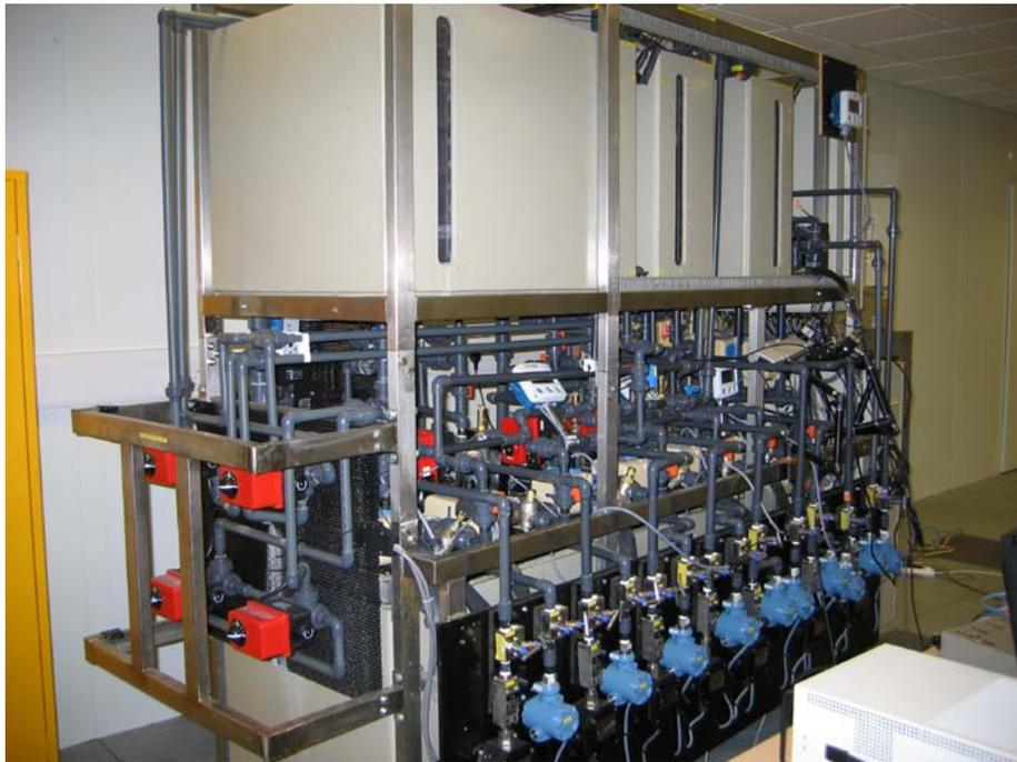
**Figure 79: BAE hardware fuel rig.**
